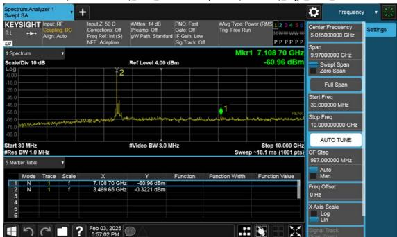
n77(3450~3550 MHz)\_80 M\_Conducted Spurious(30 M-10 G)\_High\_BPSK\_1RB
