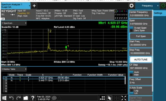
n77(3450~3550 MHz)\_80 M\_Conducted Spurious(30 M-10 G)\_Low\_BPSK\_1RB
