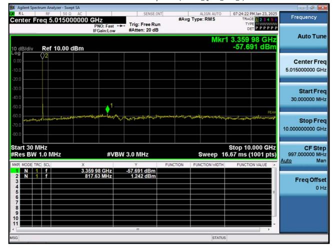
BAND 26. Conducted Spurious (10 MHz\_QPSK\_RB 1\_0)
