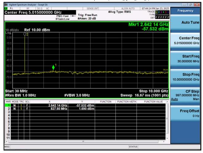
BAND 26. Conducted Spurious (1.4 MHz\_QPSK\_RB 1\_0)
