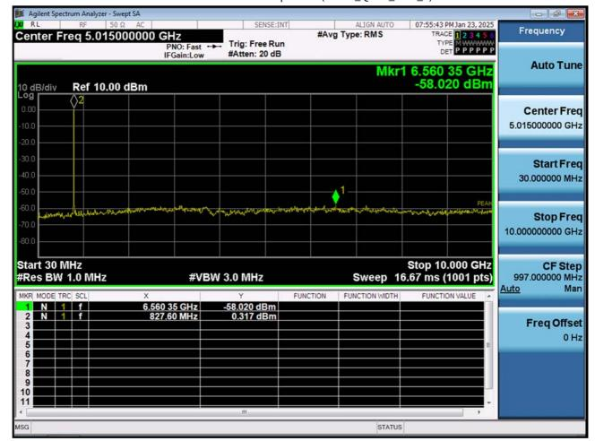
BAND 26. Conducted Spurious (3 MHz\_QPSK\_RB 1\_0)
