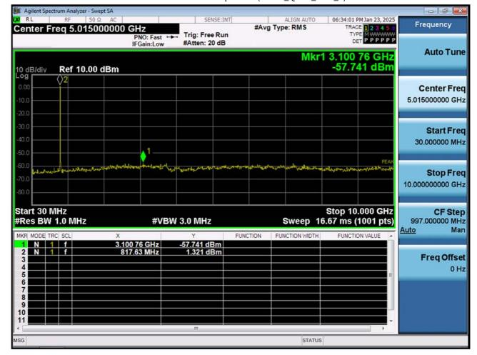
BAND 26. Conducted Spurious (5 MHz\_QPSK\_RB 1\_0)
