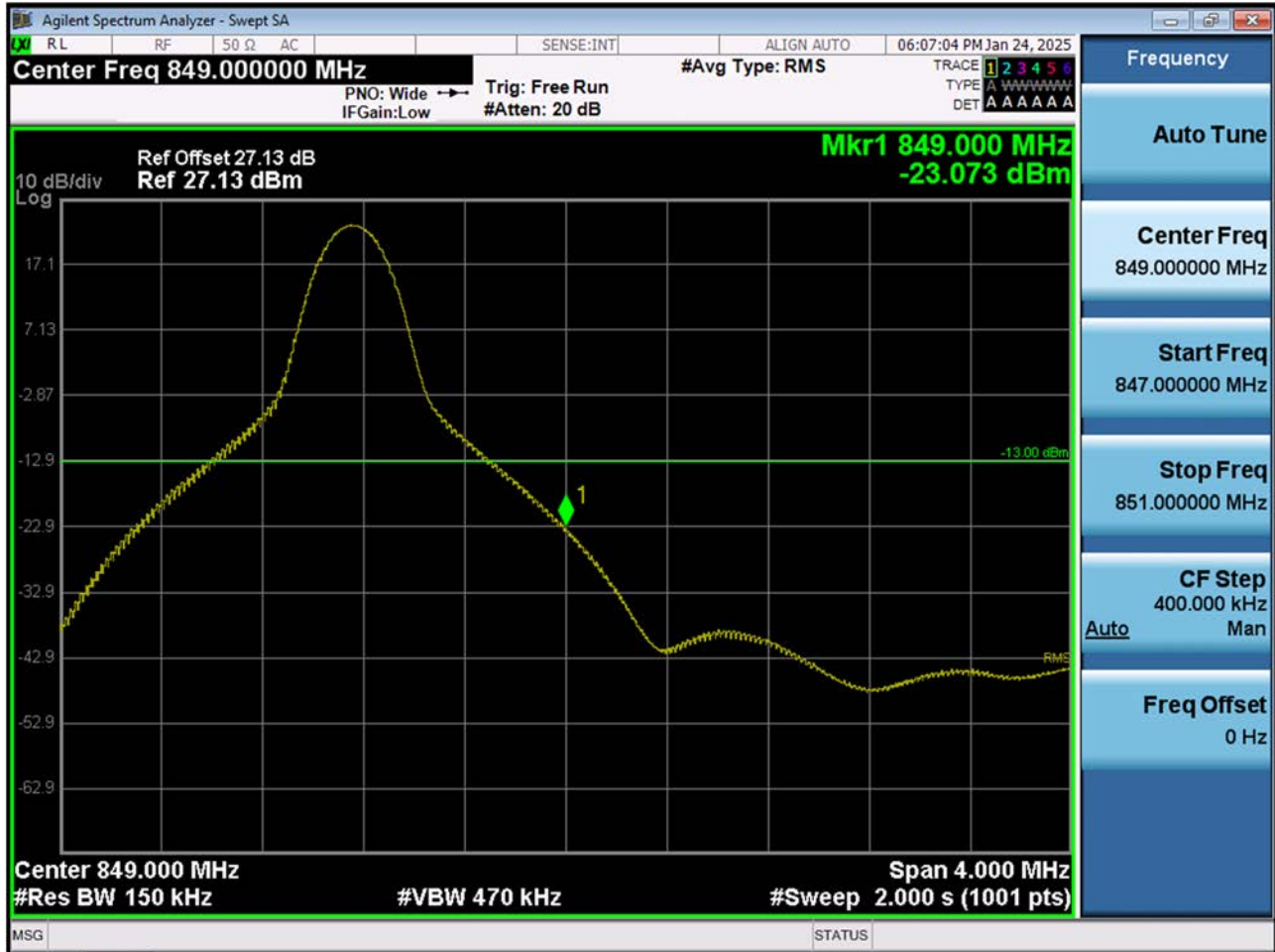
BAND 26. Upper Band Edge Plot (15 M BW Ch.26965 QPSK_RB1_Offset 74)
