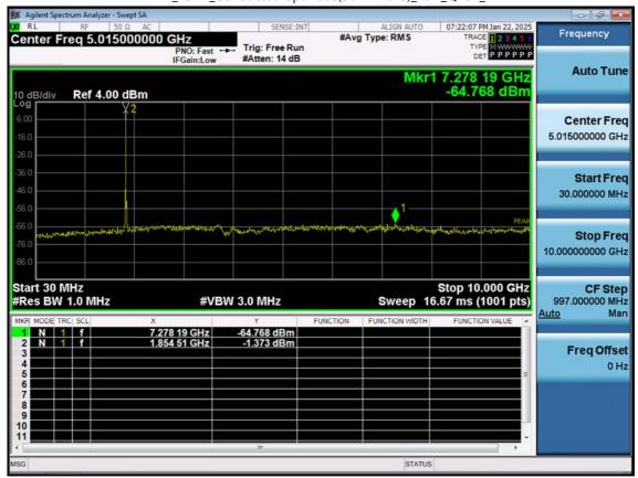
LTE B2\_15 M\_Conducted Spurious(30 M-10 G)\_Low\_QPSK\_1RB
