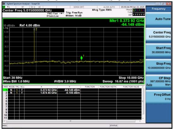
LTE B2\_5 M\_Conducted Spurious(30 M-10 G)\_Mid\_QPSK\_1RB
