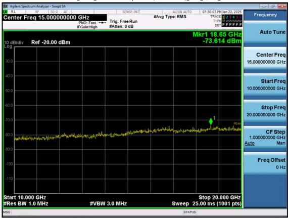
LTE B2\_20 M\_Conducted Spurious(Above10 G)\_Low\_QPSK\_1RB
