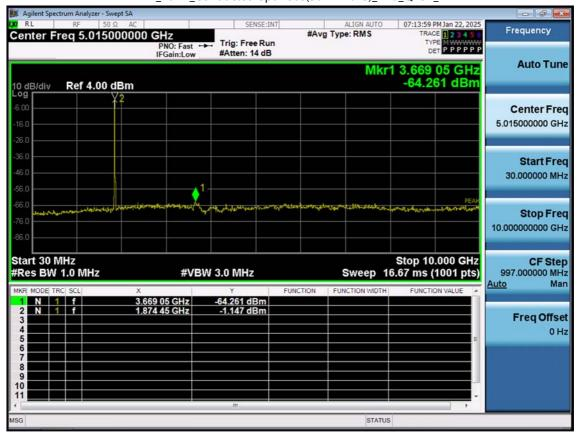
LTE B2\_10 M\_Conducted Spurious(30 M-10 G)\_Mid\_QPSK\_1RB
