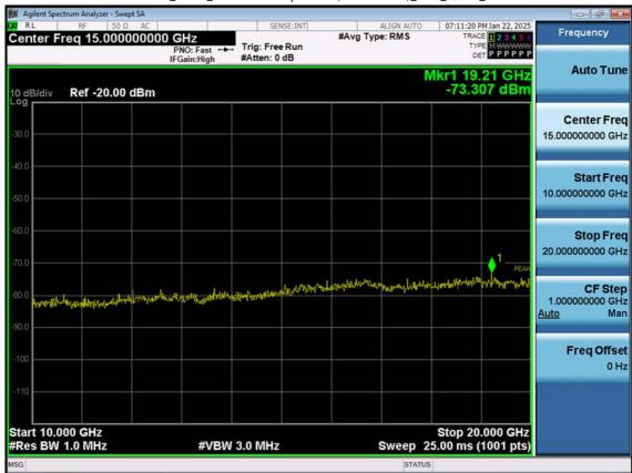
LTE B2\_10 M\_Conducted Spurious(Above10 G)\_Low\_QPSK\_1RB
