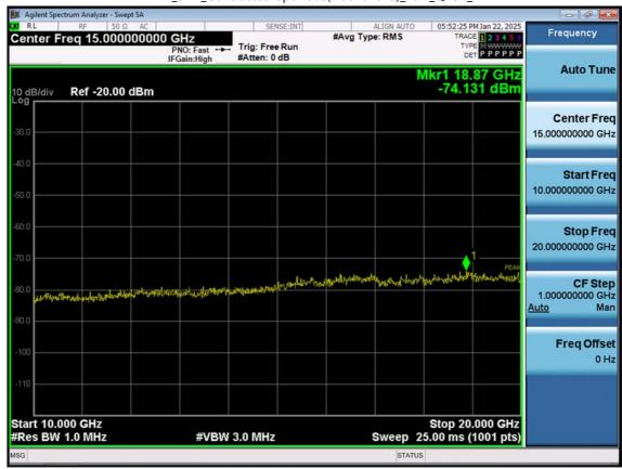
LTE B2\_5 M\_Conducted Spurious(Above10 G)\_Low\_QPSK\_1RB
