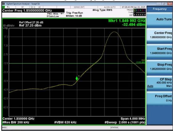
LTE B2\_20 M\_Band Edge\_Low\_QPSK\_1RB
