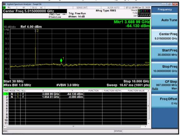
LTE B2\_10 M\_Conducted Spurious(30 M-10 G)\_Low\_QPSK\_1RB
