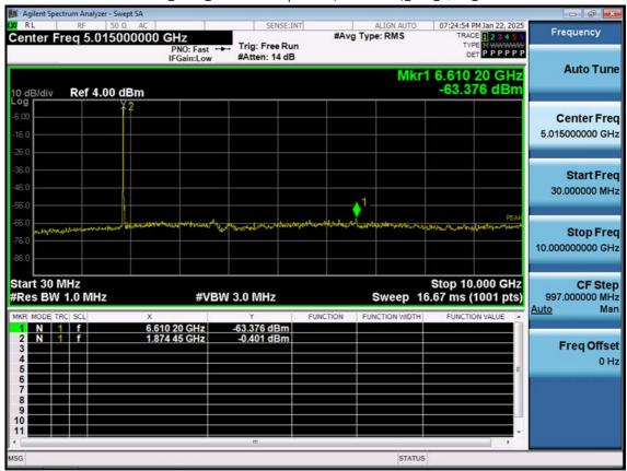
LTE B2\_15 M\_Conducted Spurious(30 M-10 G)\_Mid\_QPSK\_1RB
