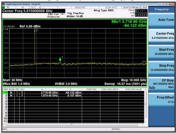
LTE B2\_3 M\_Conducted Spurious(30 M-10 G)\_Mid\_QPSK\_1RB
