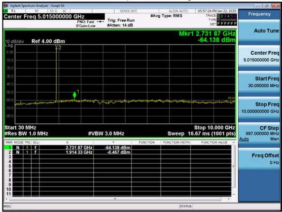
LTE B2\_5 M\_Conducted Spurious(30 M-10 G)\_High\_QPSK\_1RB
