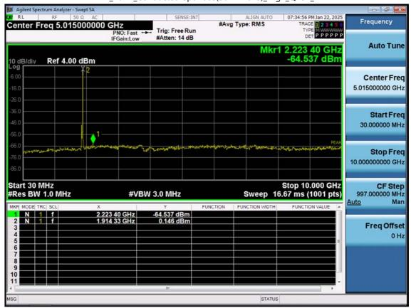
LTE B2\_20 M\_Conducted Spurious(30 M-10 G)\_High\_QPSK\_1RB
