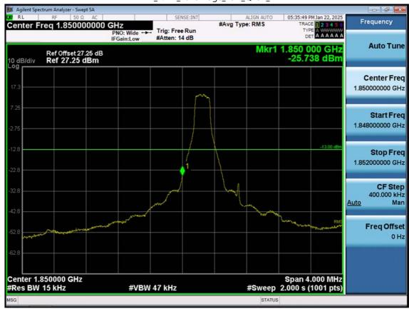
LTE B2\_1.4M\_Band Edge\_Low\_QPSK\_1RB
