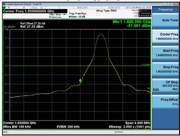
LTE B2\_10 M\_Band Edge\_Low\_QPSK\_1RB
