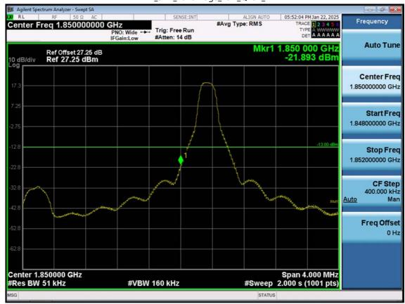
LTE B2\_5 M\_Band Edge\_Low\_QPSK\_1RB
