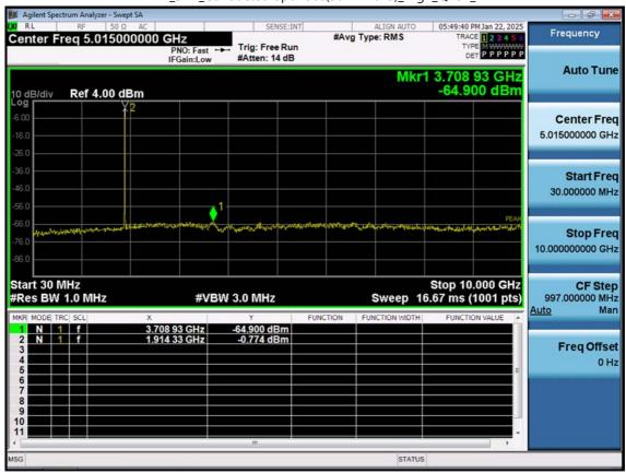
LTE B2\_3 M\_Conducted Spurious(30 M-10 G)\_High\_QPSK\_1RB
