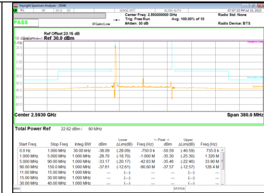
DFT-s_OFDM_16QAM Mid channel 1RB_Offset Low
