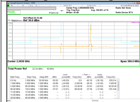
DFT-s_OFDM_16QAM Mid channel 1RB_Offset High
