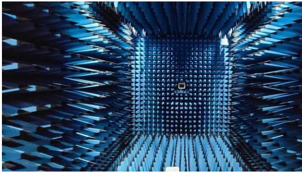
Figure 2: Geometry of Anechoic Chamber for Radiation patterns.
