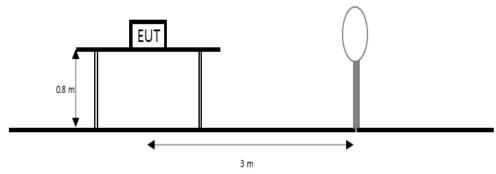
The diagram below shows the test setup that is utilized to make the measurements for emission from 30 Mb to 1 Gb emissions.
