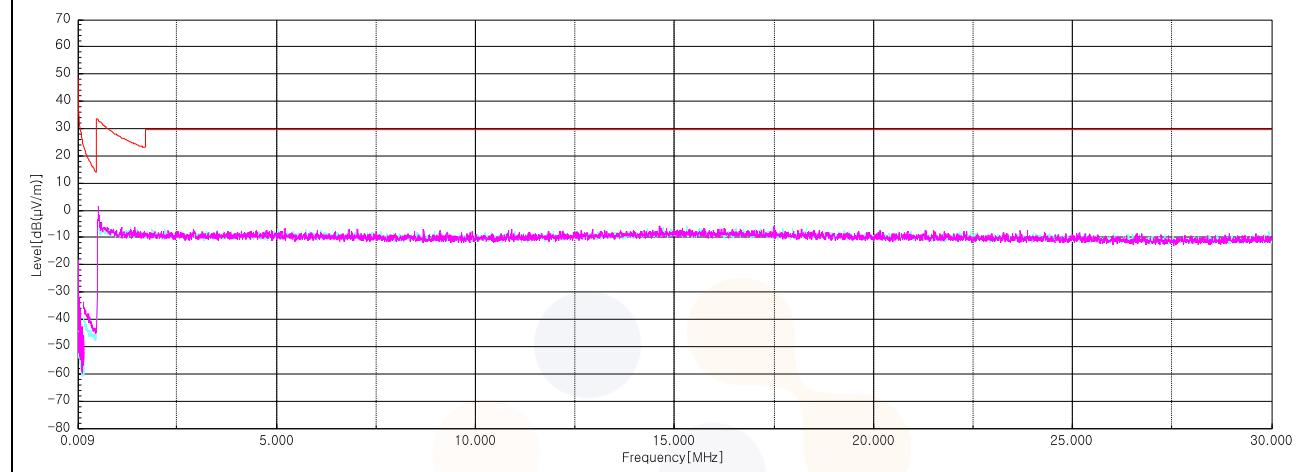
**Test results (Below 1 000 MHz) – Worst case: GFSK 2 480 MHz**
