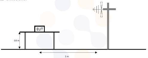
The diagram below shows the test setup that is utilized to make the measurements for emission from 1  $\mathbb{G}_{\mathbb{Z}}$  to the tenth harmonic of the highest fundamental frequency or to 40  $\mathbb{G}_{\mathbb{Z}}$  emissions, whichever is lower.
