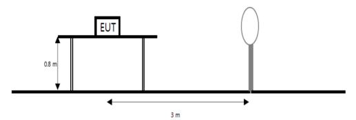
The diagram below shows the test setup that is utilized to make the measurements for emission from 30 Mtz to 1 Gtz emissions.
