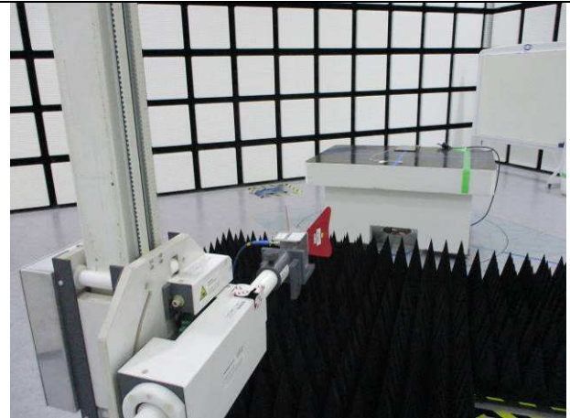
RADIATED FRONT PHOTO (ABOVE 1 GHz)
