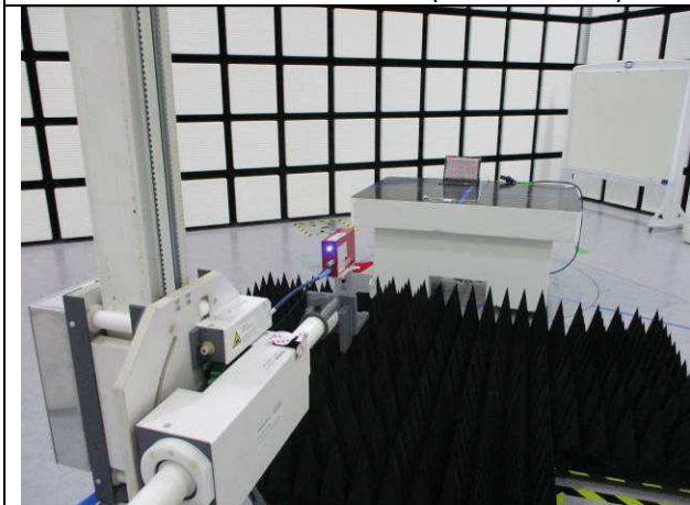
RADIATED FRONT PHOTO (ABOVE 18 GHz)
