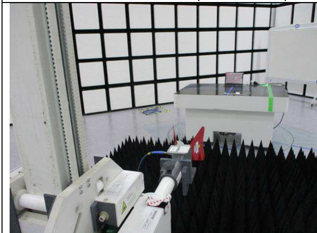
RADIATED FRONT PHOTO (ABOVE 1 GHz)
