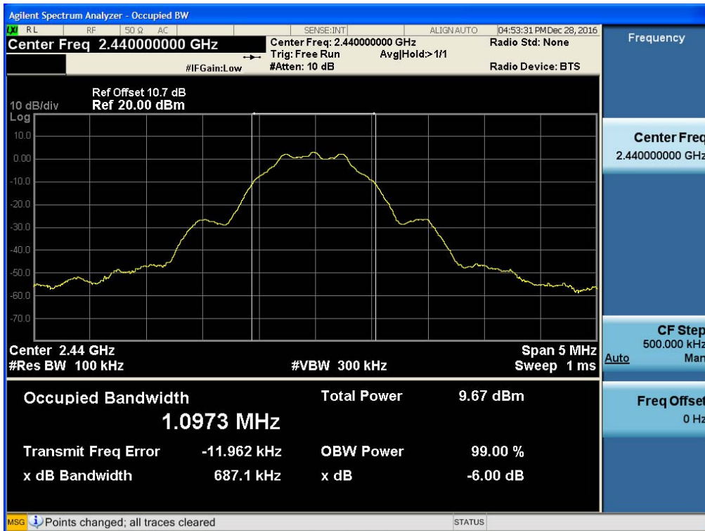
6 dB Bandwidth plot (Mid-CH 19)
