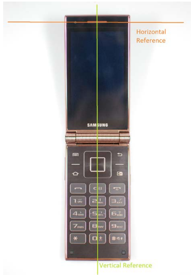
SARTest Setup Photo 11 - Vertical and Horizontal Reference Lines
