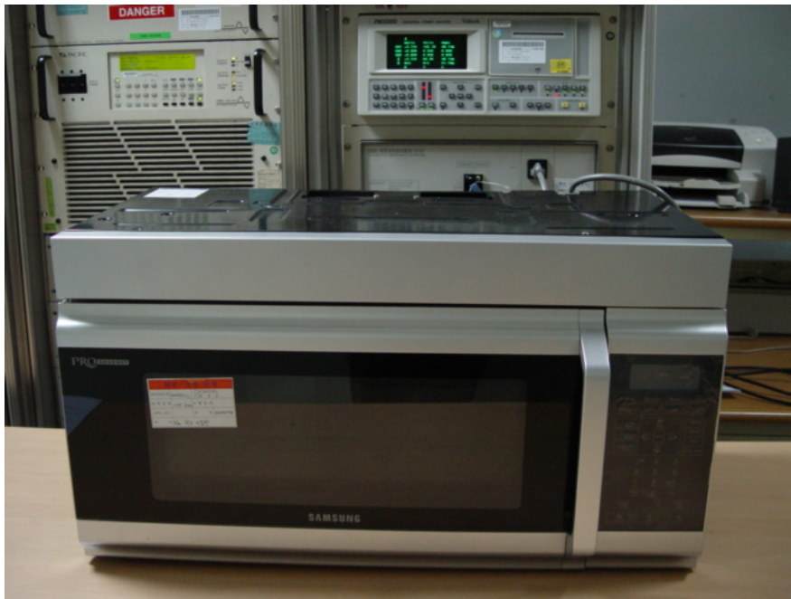
Fig. 2 Test Setup for Input power
