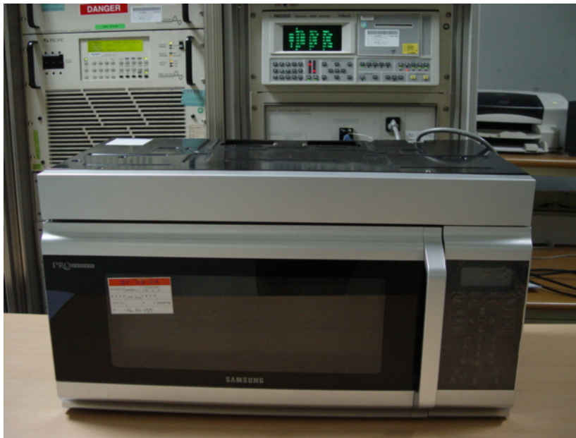
Fig.3 Test Setup for RF output power
