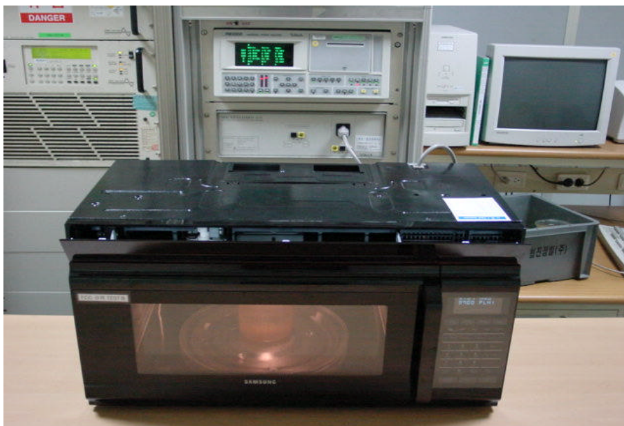
Fig.3 Test Setup for RF output power
