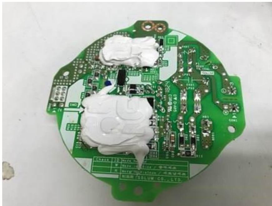
[Rear View of Power Board]
