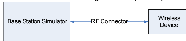
Figure 7-2 Power Measurement Setup
