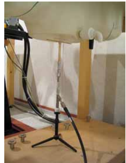
Photo of the dipole Antenna
