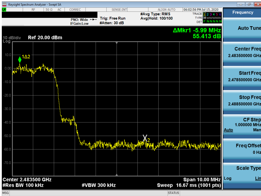
Plot 7-62. Band Edge Plot (Bluetooth with Hopping Enabled, 3 Mbps)
