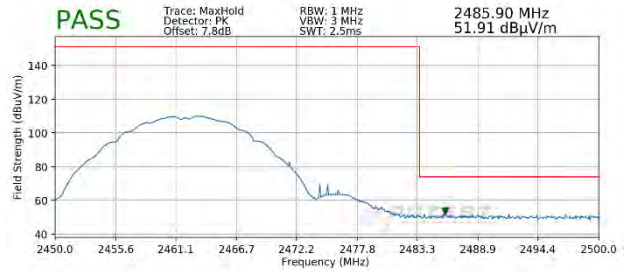
Plot 7-120. Radiated Restricted Upper Band Edge Measurement SISO ANT1 (Peak)
