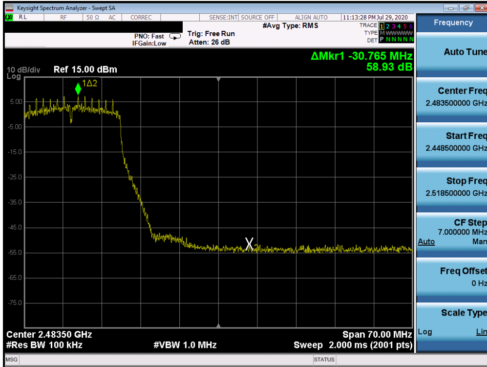
Plot 7-73. Band Edge Plot SISO ANT1 (802.11ac (2.4GHz) – Ch. 10)
