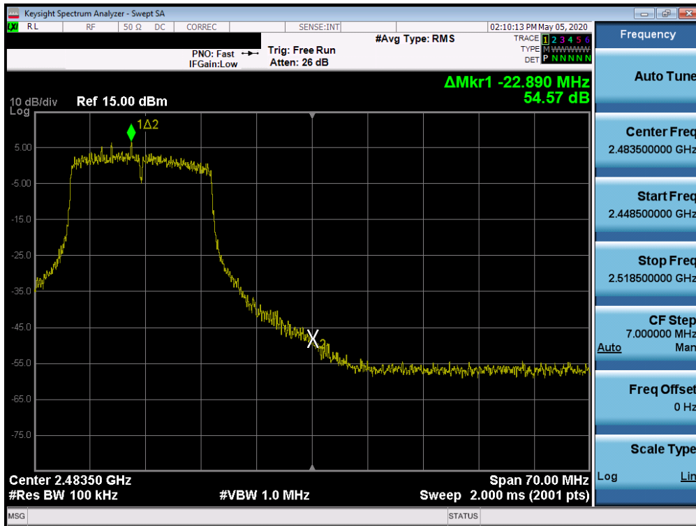
Plot 7-88. Band Edge Plot SISO ANT2 (802.11ac (2.4GHz) – Ch. 11)
