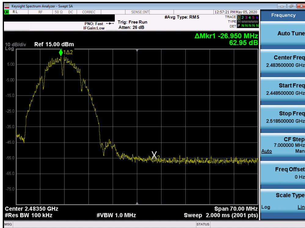
Plot 7-78. Band Edge Plot SISO ANT2 (802.11b – Ch. 11)
