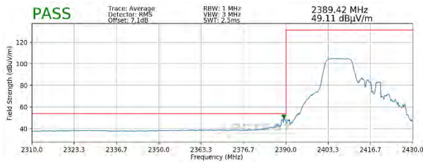
Plot 7-97. Radiated Restricted Lower Band Edge Measurement MIMO (Average – 106 Tones)
