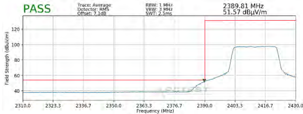
Plot 7-101. Radiated Restricted Lower Band Edge Measurement MIMO (Average – 242 Tones)
