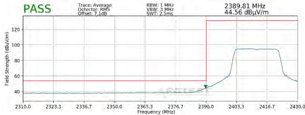
Plot 7-93. Radiated Restricted Lower Band Edge Measurement SISO ANT2 (Average – 242 Tones)
