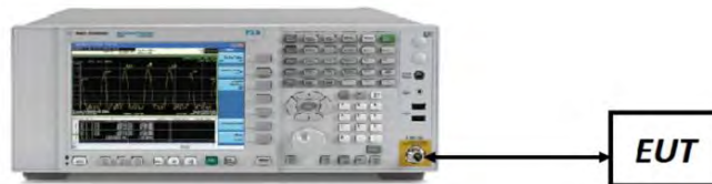
Figure 7-3. Test Instrument & Measurement Setup
