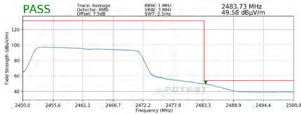
Plot 7-95. Radiated Restricted Upper Band Edge Measurement SISO ANT2 (Average – 242 Tones)
