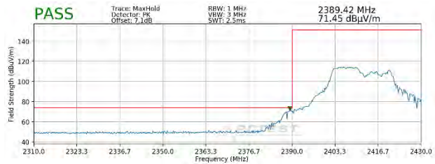
Plot 7-98. Radiated Restricted Lower Band Edge Measurement MIMO (Peak – 106 Tones)
