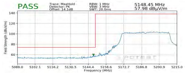
Plot 7-336. Radiated Lower Band Edge Plot MIMO (Peak – UNII Band 1)
