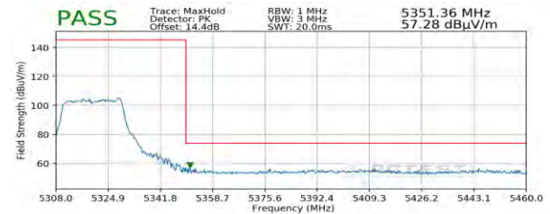
Plot 7-289. Radiated Upper Band Edge Plot SISO ANT1 (Peak – UNII Band 2A)
