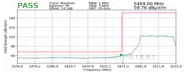
Plot 7-319. Radiated Lower Band Edge Plot SISO ANT2 (Peak – UNII Band 2C)
