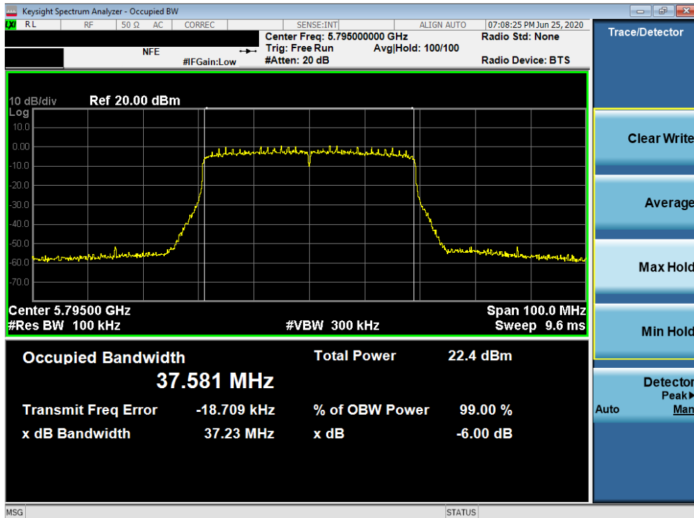
Plot 7-124. 6dB Bandwidth Plot SISO ANT2 (40MHz BW 802.11ax SU (UNII Band 3) – Ch. 159)
