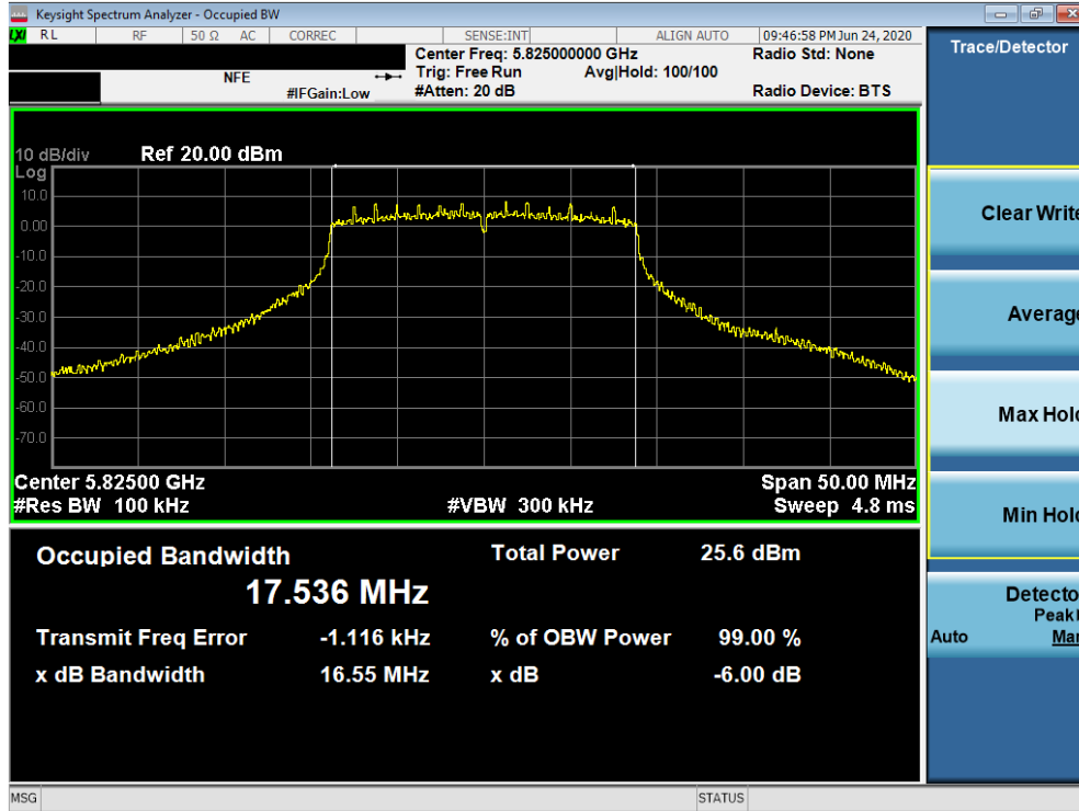
Plot 7-102. 6dB Bandwidth Plot SISO ANT1 (20MHz BW 802.11n (UNII Band 3) – Ch. 165)
