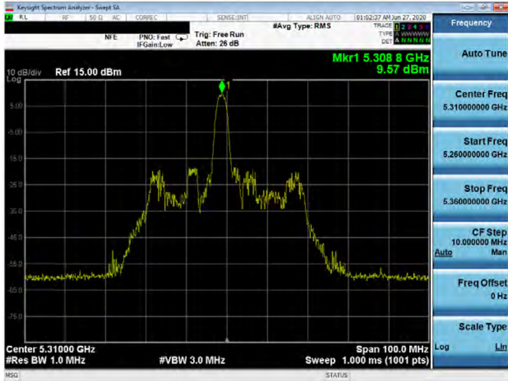
Plot 7-173. Power Spectral Density Plot SISO ANT2 (40MHz BW 802.11ax – 26 Tones (UNII Band 2A) – Ch. 62)
