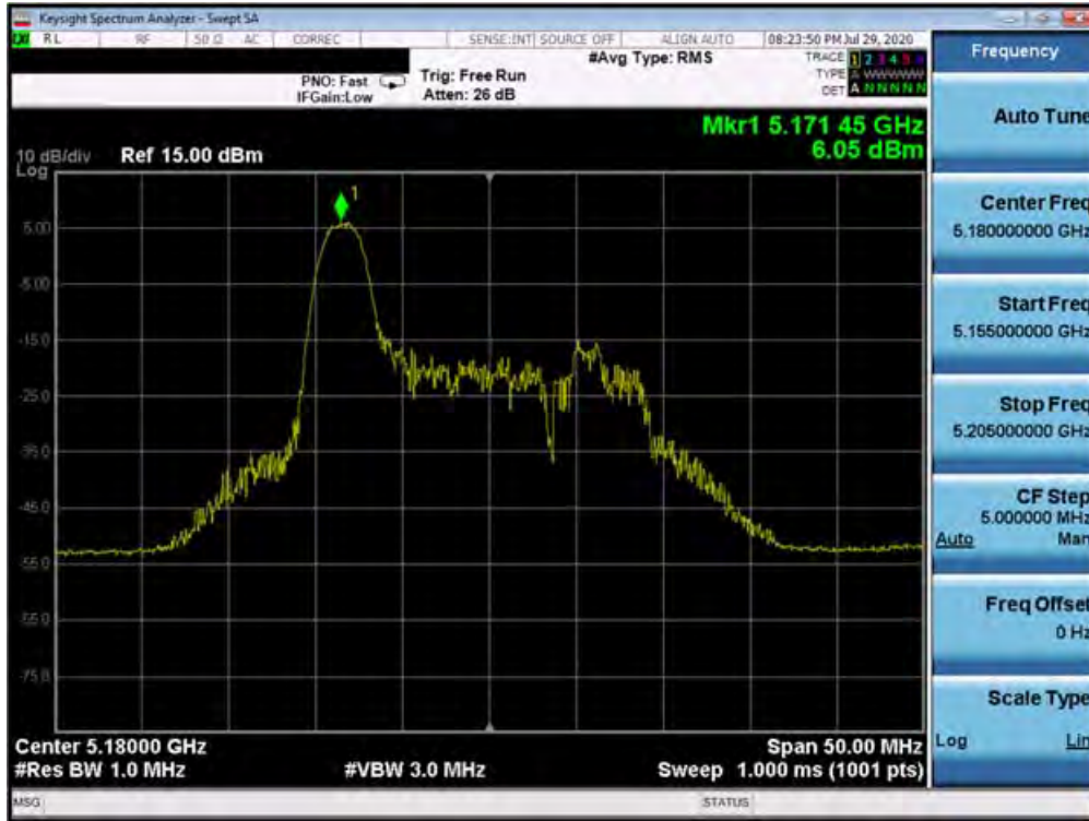
Plot 7-217. Power Spectral Density Plot MIMO ANT1 (20MHz BW 802.11ax – 26 Tones (UNII Band 1) – Ch. 36)
