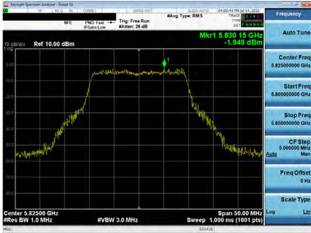
Plot 7-159. Power Spectral Density Plot SISO ANT1 (20 MHz BW 802.11ax – Full Tones (UNII Band 3) – Ch. 165)
