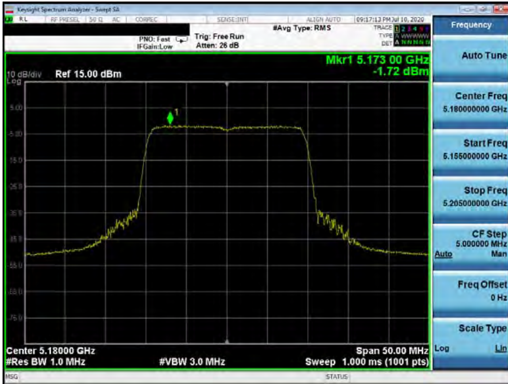
Plot 7-190. Power Spectral Density Plot SISO ANT2 (20MHz BW 802.11ax – Full Tones (UNII Band 1) – Ch. 36)
