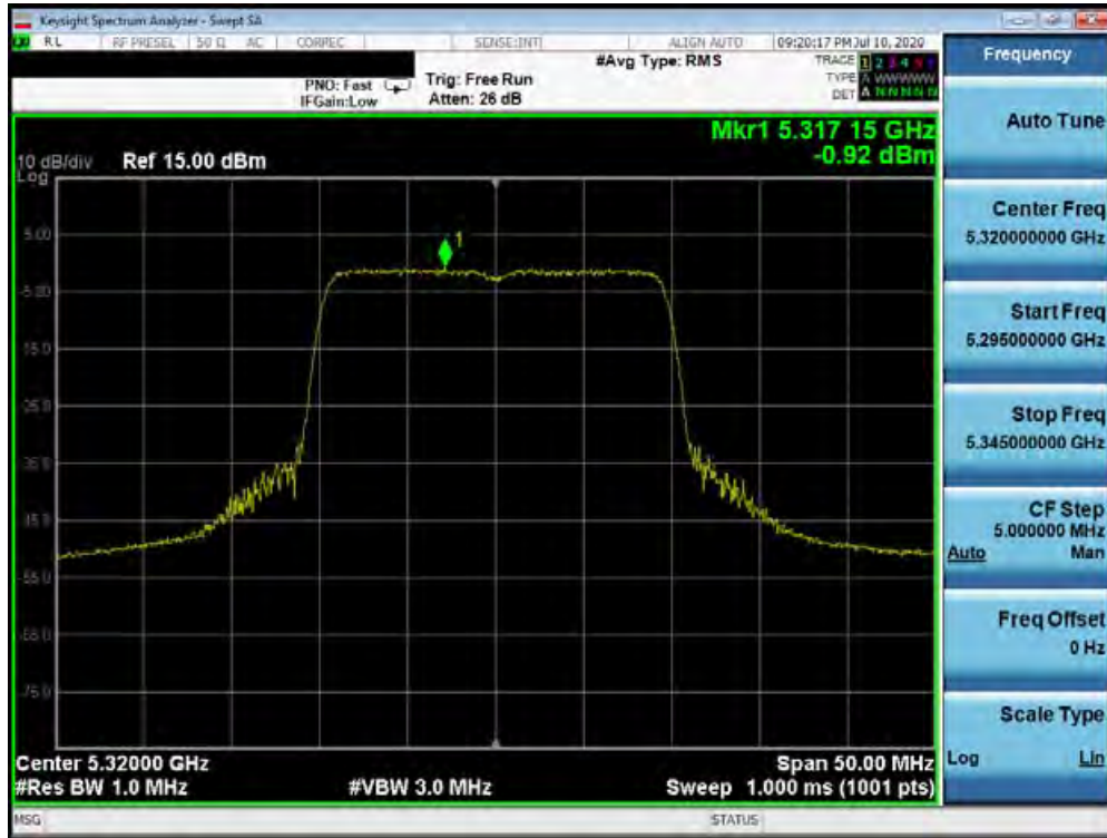
Plot 7-198. Power Spectral Density Plot SISO ANT2 (20MHz BW 802.11ax – Full Tones (UNII Band 2A) – Ch. 64)
