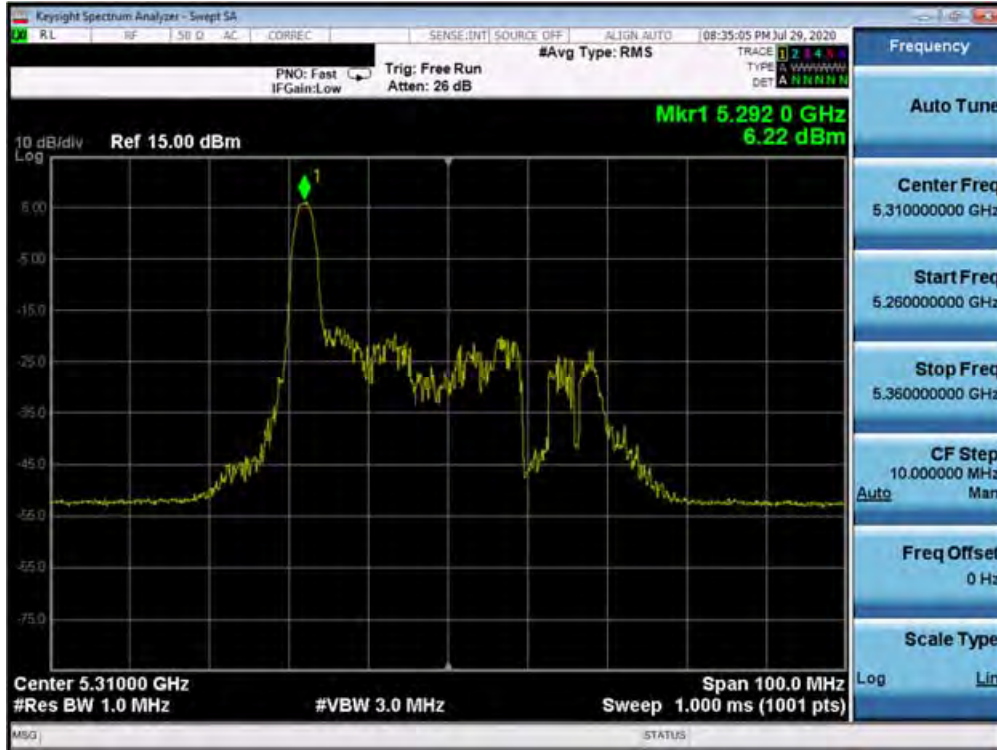
Plot 7-254. Power Spectral Density Plot MIMO ANT2 (40MHz BW 802.11ax – 26 Tones (UNII Band 2A) – Ch. 62)
