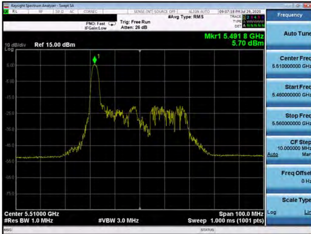
Plot 7-259. Power Spectral Density Plot MIMO ANT2 (40MHz BW 802.11ax – 26 Tones (UNII Band 2C) – Ch. 102)
