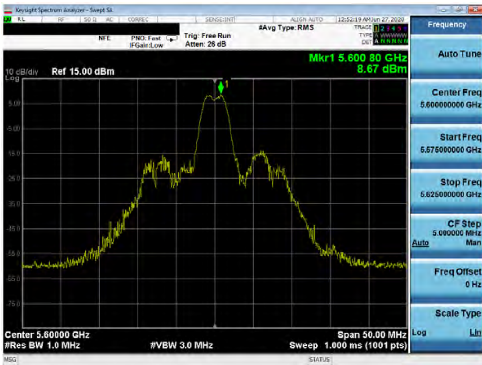
Plot 7-176. Power Spectral Density Plot SISO ANT2 (20MHz BW 802.11ax – 26 Tones (UNII Band 2C) – Ch. 120)
