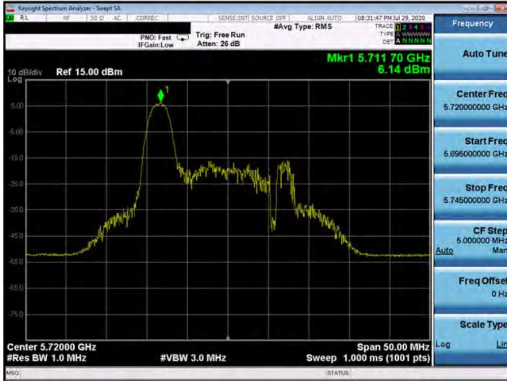
Plot 7-231. Power Spectral Density Plot MIMO ANT1 (20MHz BW 802.11ax – 26 Tones (UNII Band 2C) – Ch. 144)
