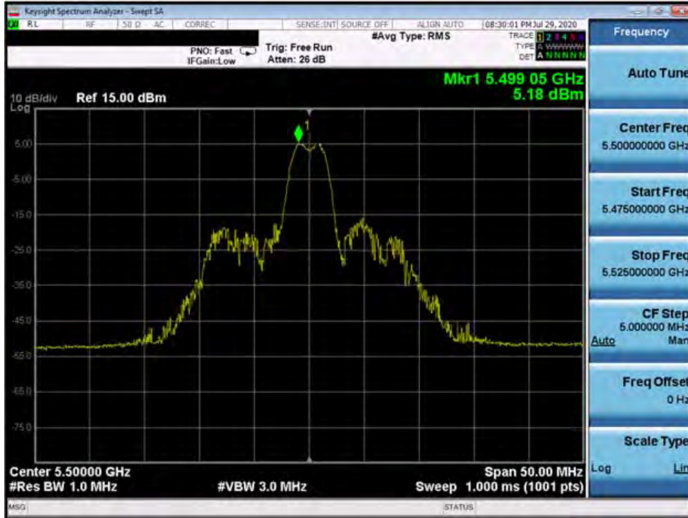
Plot 7-229. Power Spectral Density Plot MIMO ANT1 (20MHz BW 802.11ax – 26 Tones (UNII Band 2C) – Ch. 100)
