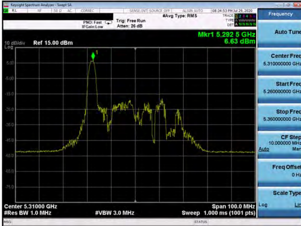
Plot 7-227. Power Spectral Density Plot MIMO ANT1 (40MHz BW 802.11ax – 26 Tones (UNII Band 2A) – Ch. 62)
