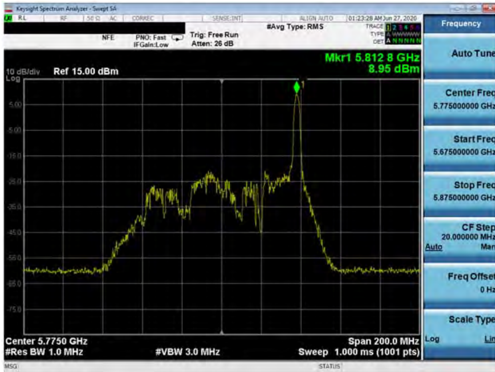
Plot 7-243. Power Spectral Density Plot MIMO ANT1 (80MHz BW 802.11ax – 26 Tones (UNII Band 3) – Ch. 155)
