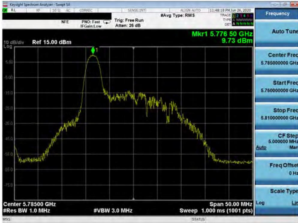
Plot 7-239. Power Spectral Density Plot MIMO ANT1 (20MHz BW 802.11ax – 26 Tones (UNII Band 3) – Ch. 157)
