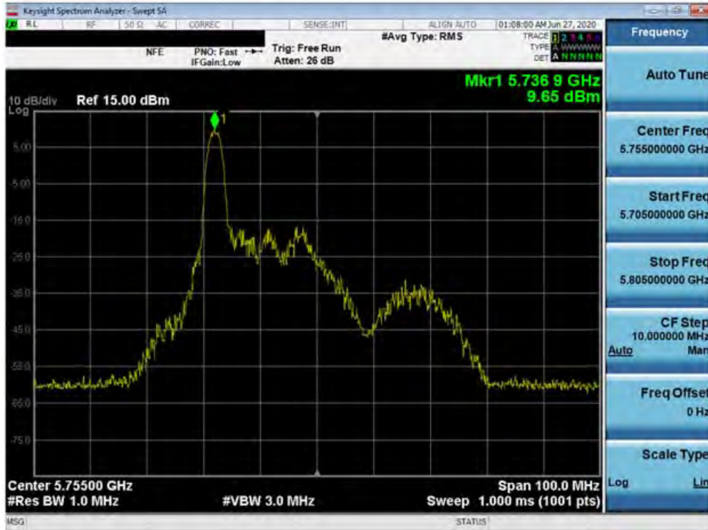
Plot 7-268. Power Spectral Density Plot MIMO ANT2 (40MHz BW 802.11ax – 26 Tones (UNII Band 3) – Ch. 151)
