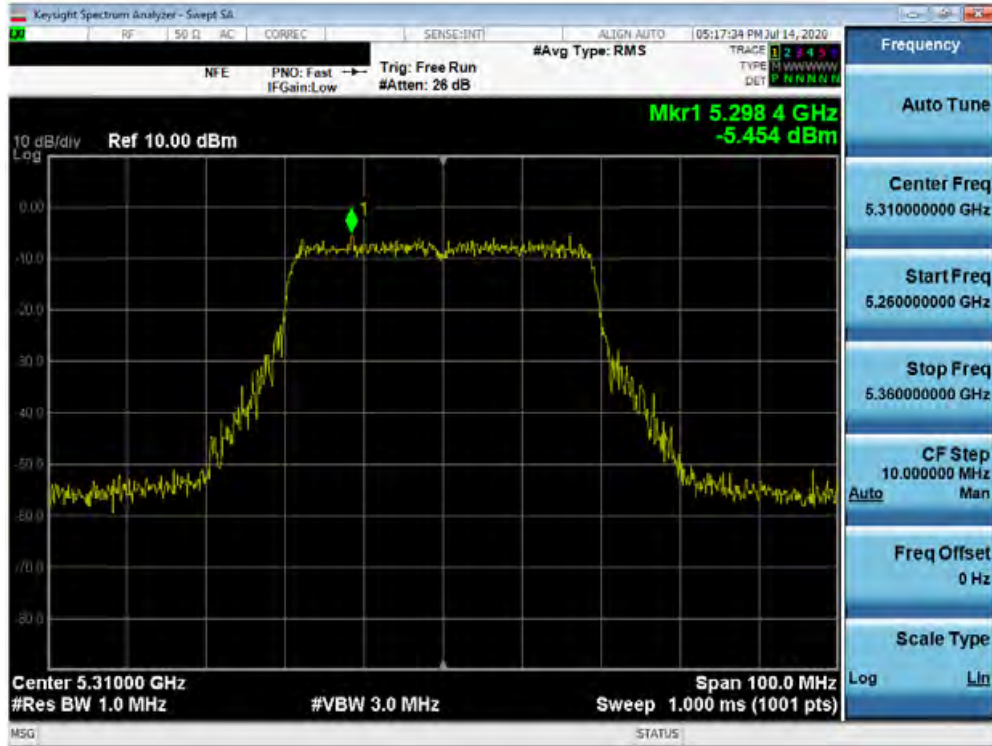
Plot 7-200. Power Spectral Density Plot SISO ANT2 (40MHz BW 802.11ax – Full Tones (UNII Band 2A) – Ch. 62)
