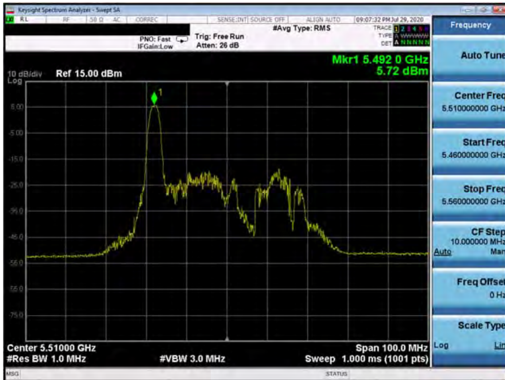
Plot 7-232. Power Spectral Density Plot MIMO ANT1 (40MHz BW 802.11ax – 26 Tones (UNII Band 2C) – Ch. 102)
