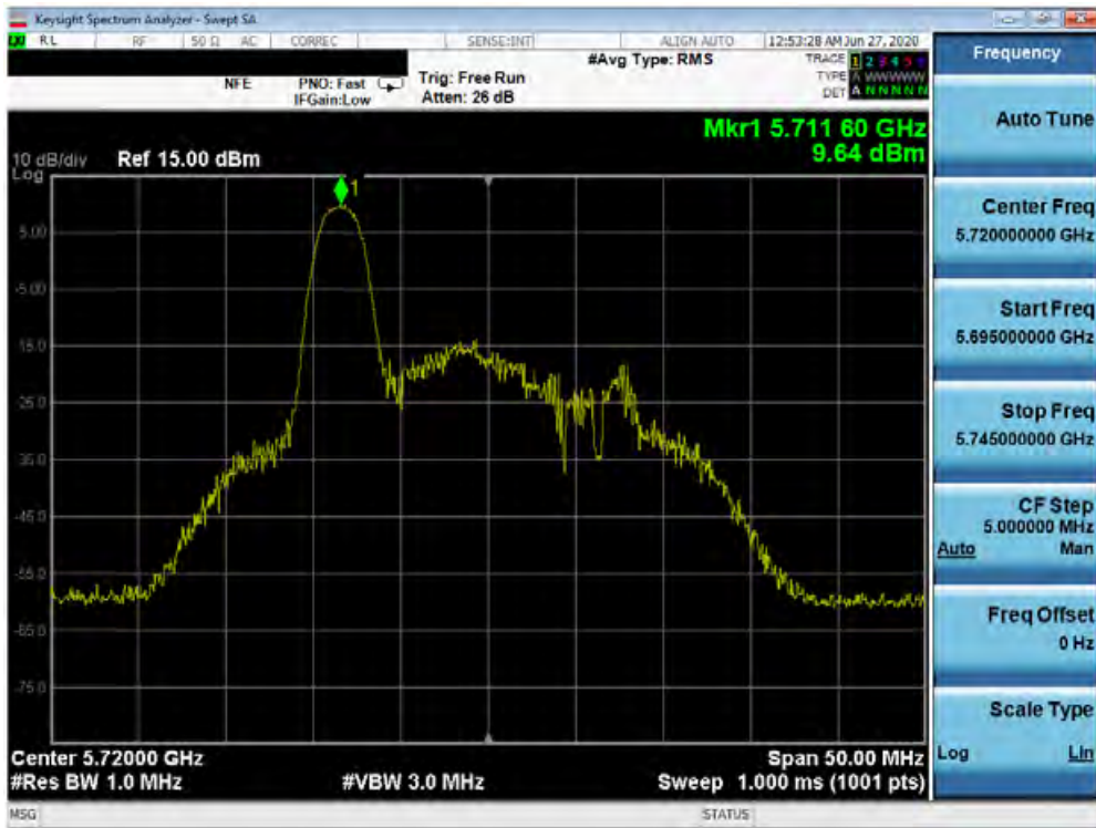
Plot 7-177. Power Spectral Density Plot SISO ANT2 (20MHz BW 802.11ax – 26 Tones (UNII Band 2C) – Ch. 144)
