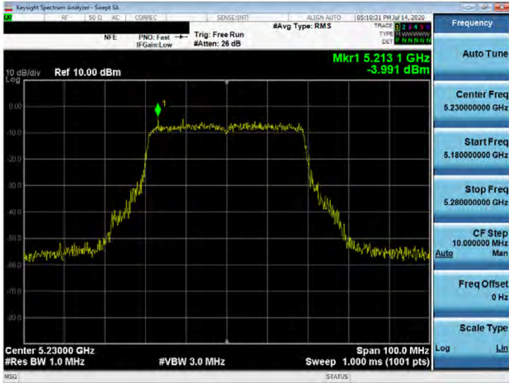
Plot 7-194. Power Spectral Density Plot SISO ANT2 (40MHz BW 802.11ax – Full Tones (UNII Band 1) – Ch. 46)
