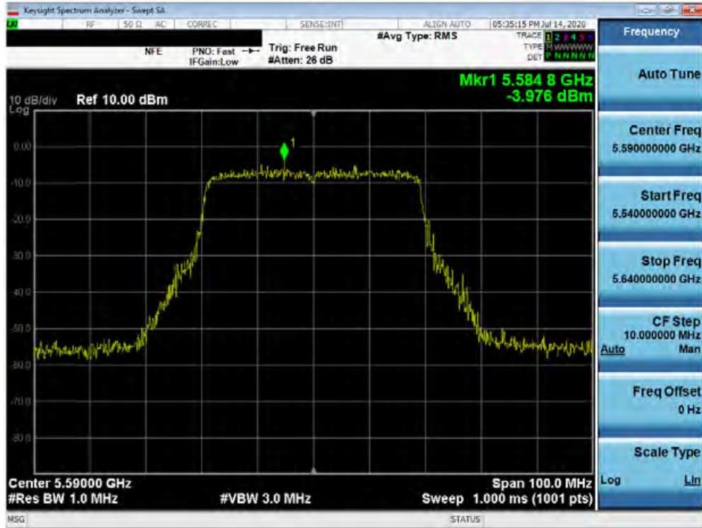
Plot 7-206. Power Spectral Density Plot SISO ANT2 (40MHz BW 802.11ax – Full Tones (UNII Band 2C) – Ch. 118)
