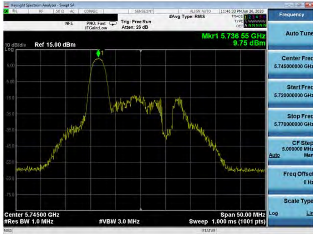
Plot 7-238. Power Spectral Density Plot MIMO ANT1 (20MHz BW 802.11ax – 26 Tones (UNII Band 3) – Ch. 149)
