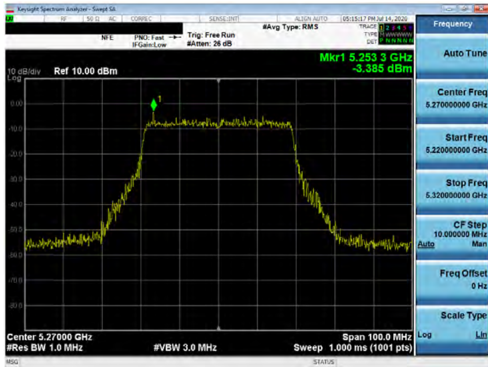
Plot 7-199. Power Spectral Density Plot SISO ANT2 (40MHz BW 802.11ax – Full Tones (UNII Band 2A) – Ch. 54)
