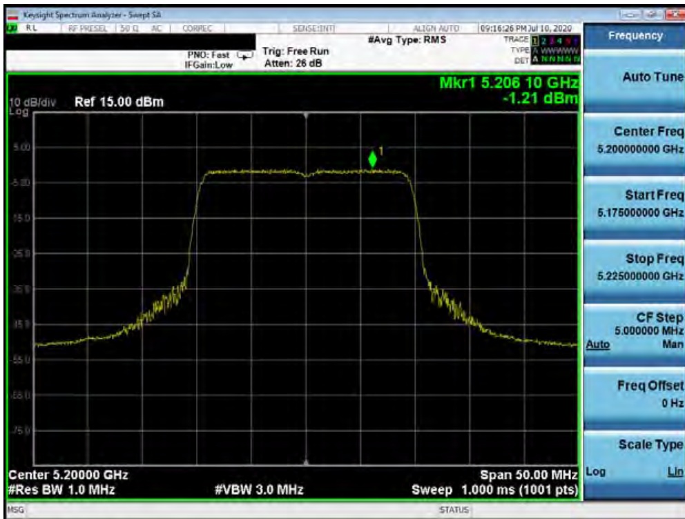
Plot 7-191. Power Spectral Density Plot SISO ANT2 (20MHz BW 802.11ax – Full Tones (UNII Band 1) – Ch. 40)
