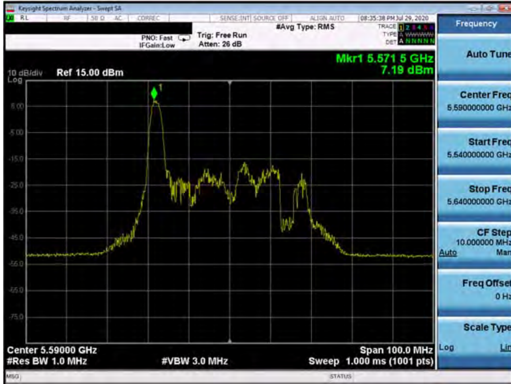
Plot 7-260. Power Spectral Density Plot MIMO ANT2 (40MHz BW 802.11ax – 26 Tones (UNII Band 2C) – Ch. 118)
