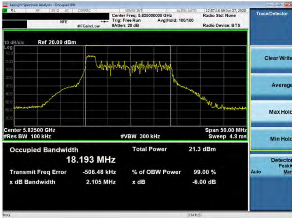
Plot 7-267. Power Spectral Density Plot MIMO ANT2 (20MHz BW 802.11ax – 26 Tones (UNII Band 3) – Ch. 165)
