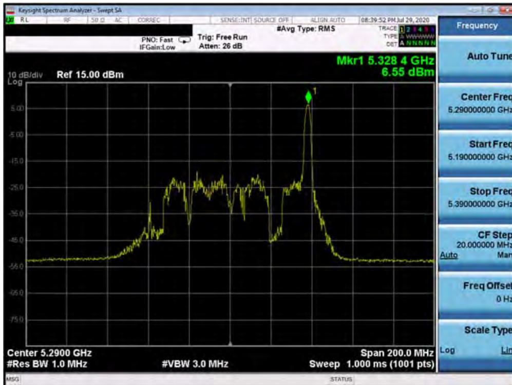
Plot 7-255. Power Spectral Density Plot MIMO ANT2 (80MHz BW 802.11ax – 26 Tones (UNII Band 2A) – Ch. 58)
