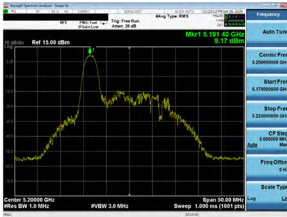
Plot 7-110. Power Spectral Density Plot SISO ANT1 (20MHz BW 802.11ax – 26 Tones (UNII Band 1) – Ch. 40)
