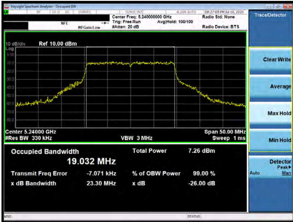
Plot 7-24. 26dB Bandwidth Plot SISO ANT1 (20MHz BW 802.11ax – 242 Tones (UNII Band 1) – Ch. 48)
