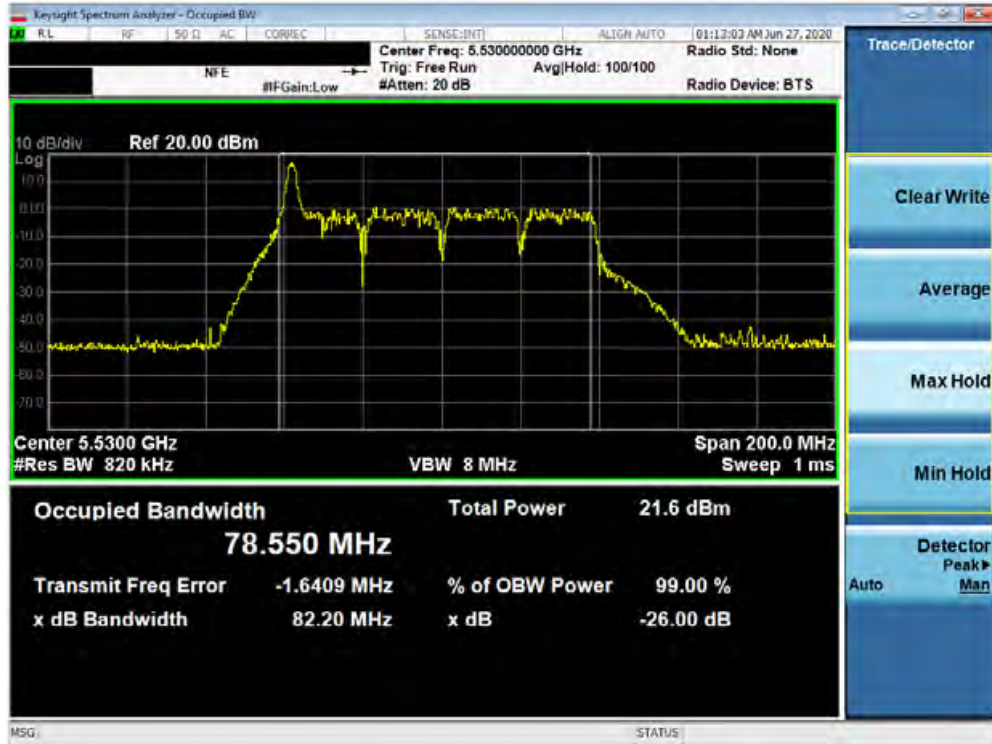
Plot 7-61. 26dB Bandwidth Plot SISO ANT2 (80MHz BW 802.11ax – 26 Tones (UNII Band 2C) – Ch. 106)
