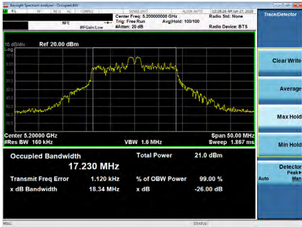
Plot 7-44. 26dB Bandwidth Plot SISO ANT2 (20MHz BW 802.11ax – 26 Tones (UNII Band 1) – Ch. 40)
