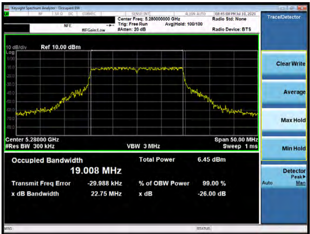
Plot 7-29. 26dB Bandwidth Plot SISO ANT1 (20MHz BW 802.11ax – 242 Tones (UNII Band 2A) – Ch. 56)
