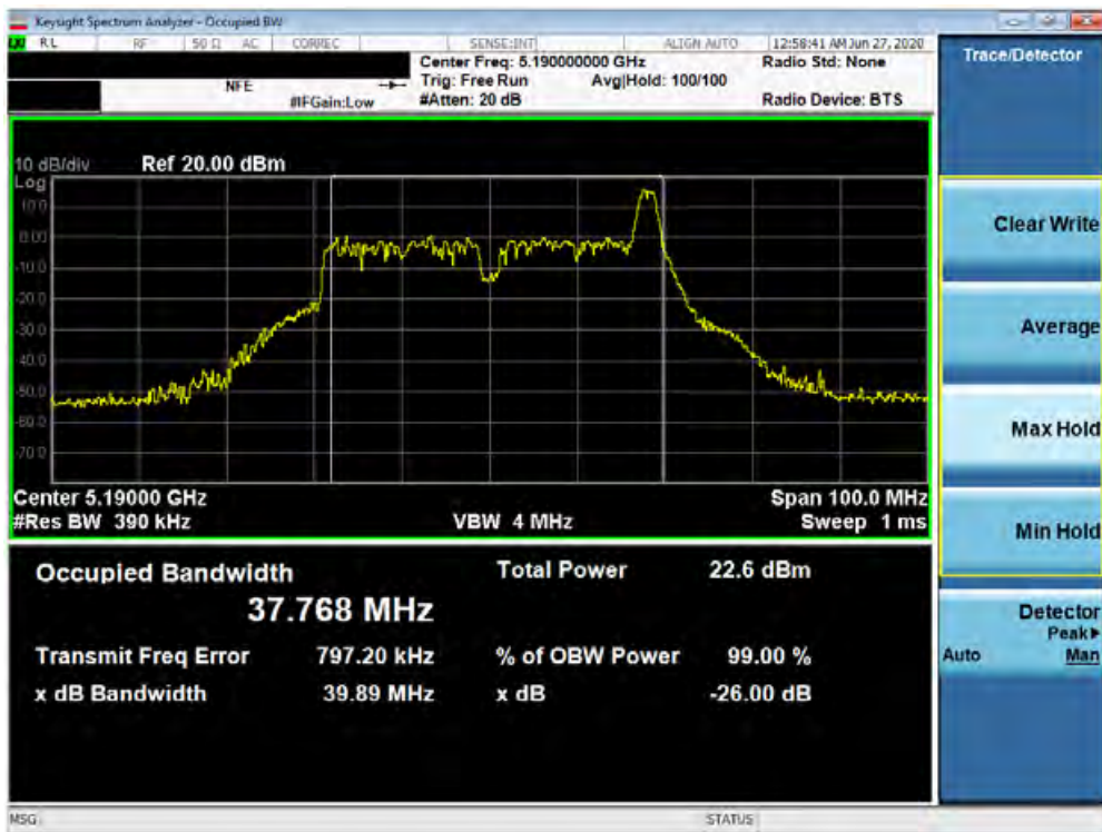
Plot 7-46. 26dB Bandwidth Plot SISO ANT2 (40MHz BW 802.11ax – 26 Tones (UNII Band 1) – Ch. 38)
