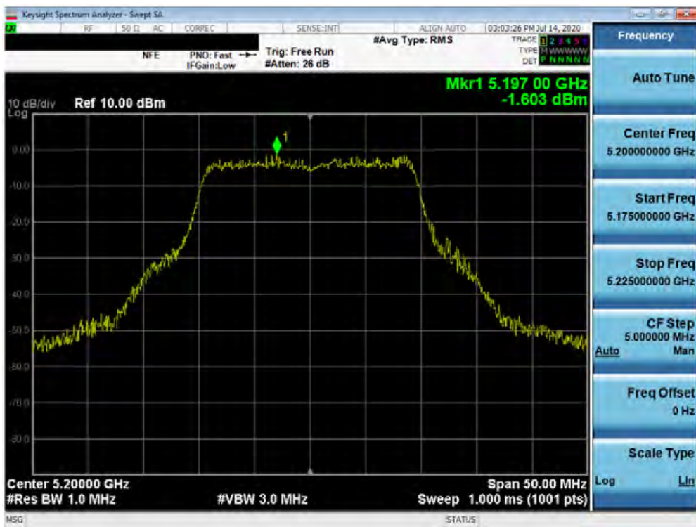
Plot 7-137. Power Spectral Density Plot SISO ANT1 (20MHz BW 802.11ax – Full Tones (UNII Band 1) – Ch. 40)
