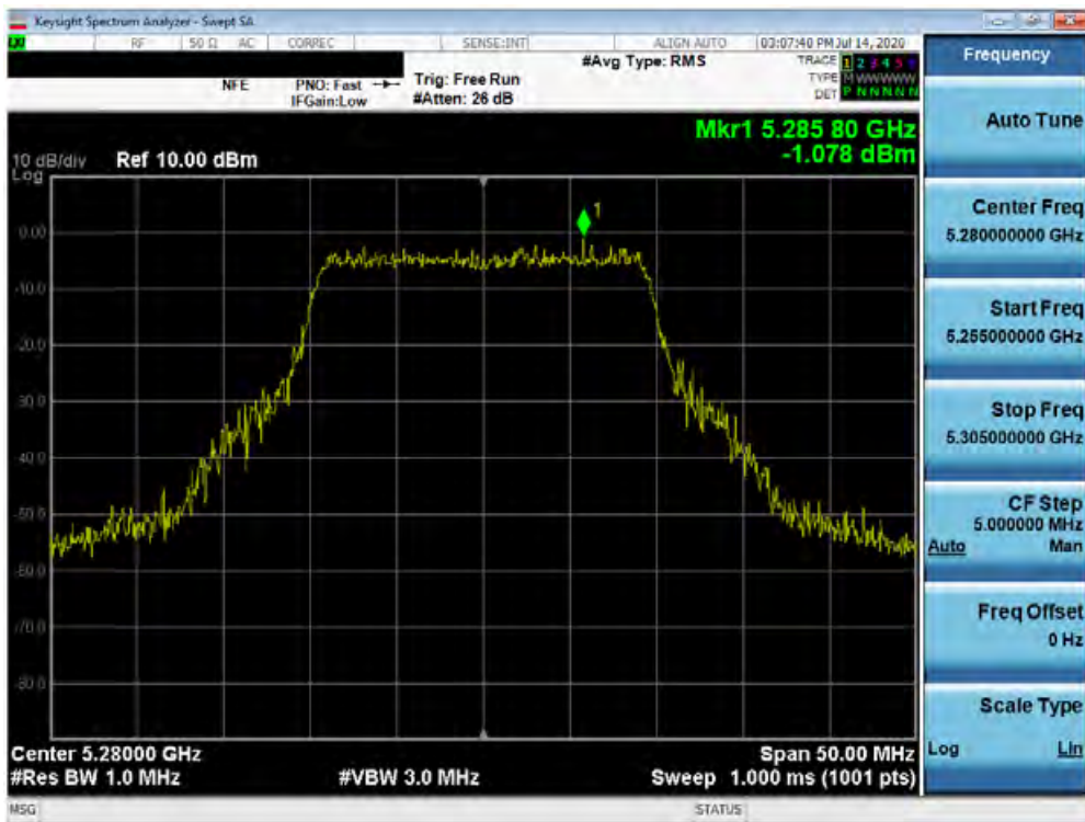
Plot 7-143. Power Spectral Density Plot SISO ANT1 (20MHz BW 802.11ax – Full Tones (UNII Band 2A) – Ch. 56)
