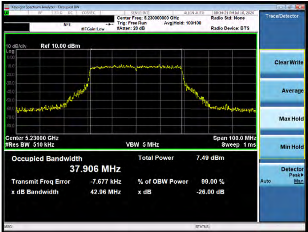
Plot 7-26. 26dB Bandwidth Plot SISO ANT1 (40MHz BW 802.11ax – 484 Tones (UNII Band 1) – Ch. 46)
