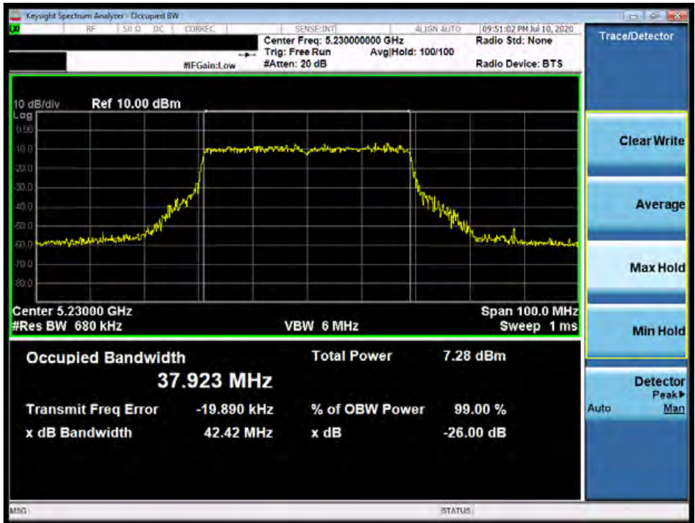
Plot 7-68. 26dB Bandwidth Plot SISO ANT2 (40MHz BW 802.11ax – 484 Tones (UNII Band 1) – Ch. 46)
