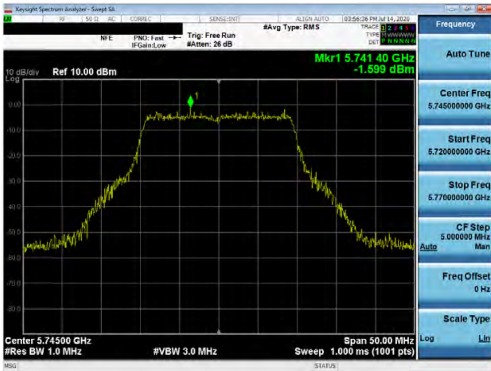
Plot 7-157. Power Spectral Density Plot SISO ANT1 (20MHz BW 802.11ax – Full Tones (UNII Band 3) – Ch. 149)
