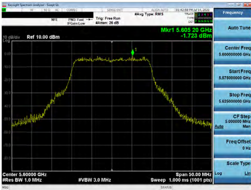
Plot 7-149. Power Spectral Density Plot SISO ANT1 (20MHz BW 802.11ax – Full Tones (UNII Band 2C) – Ch. 120)
