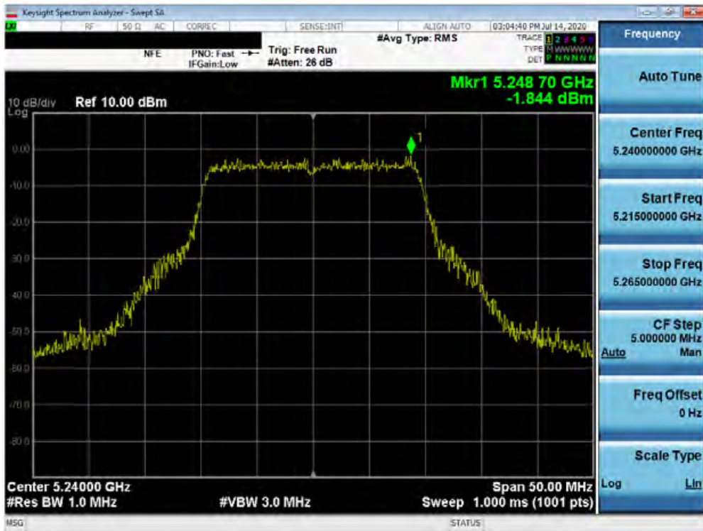
Plot 7-138. Power Spectral Density Plot SISO ANT1 (20MHz BW 802.11ax – Full Tones (UNII Band 1) – Ch. 48)
