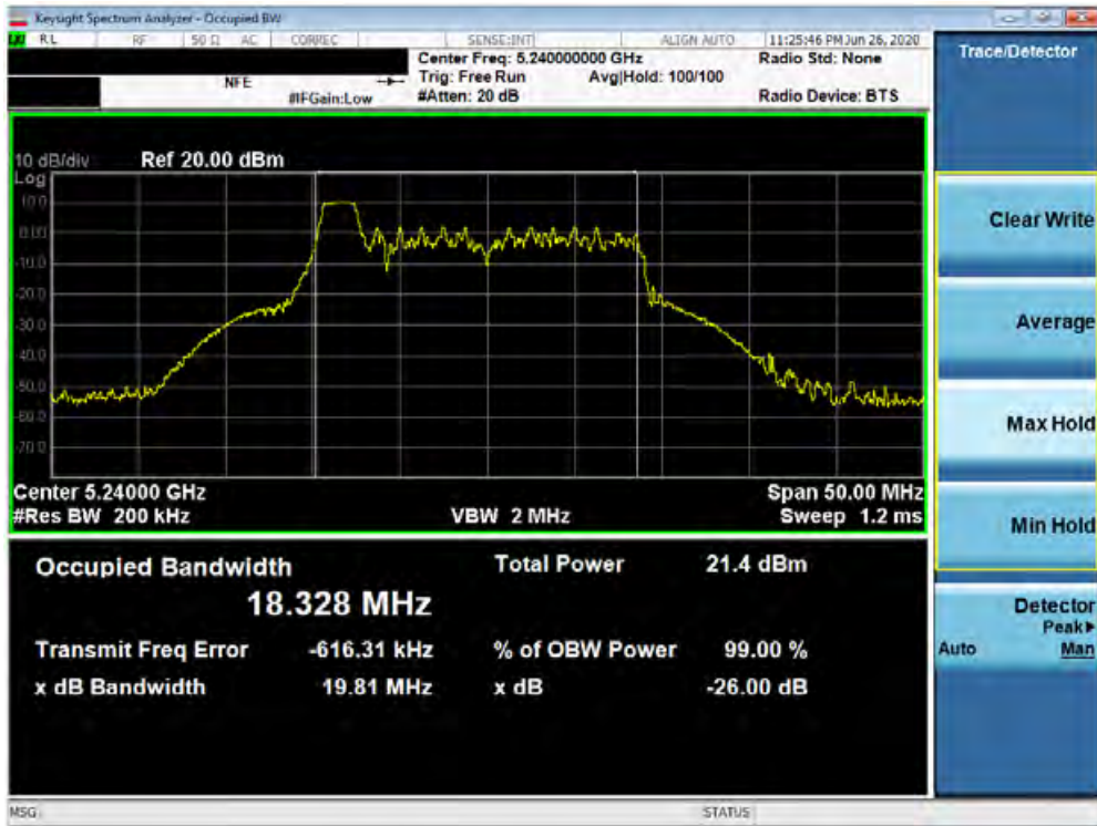
Plot 7-3. 26dB Bandwidth Plot SISO ANT1 (20MHz BW 802.11ax – 26 Tones (UNII Band 1) – Ch. 48)
