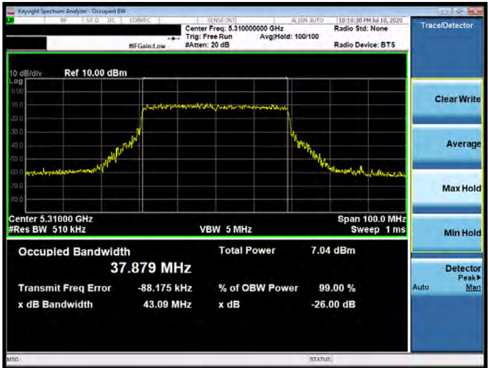
Plot 7-74. 26dB Bandwidth Plot SISO ANT2 (40MHz BW 802.11ax – 484 Tones (UNII Band 2A) – Ch. 62)
