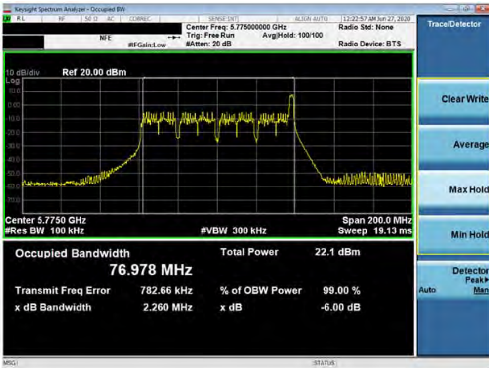
Plot 7-90. 6dB Bandwidth Plot SISO ANT1 (80MHz BW 802.11ax – 26 Tones (UNII Band 3) – Ch. 155)
