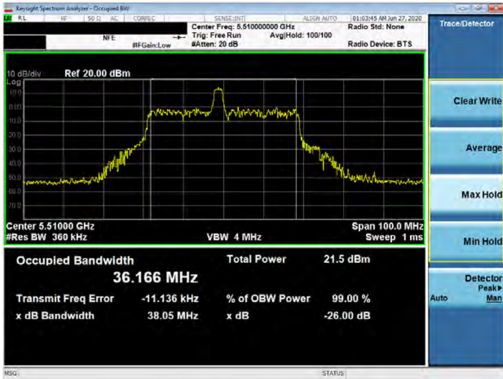
Plot 7-58. 26dB Bandwidth Plot SISO ANT2 (40MHz BW 802.11ax – 26 Tones (UNII Band 2C) – Ch. 102)
