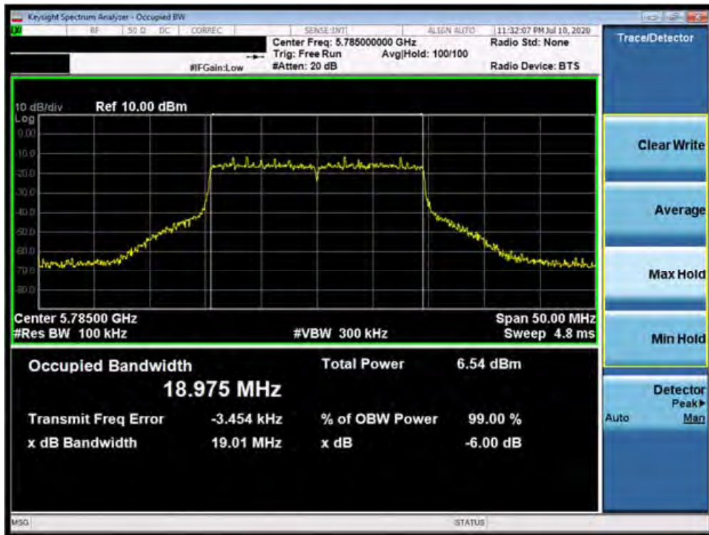
Plot 7-92. 6dB Bandwidth Plot SISO ANT1 (20MHz BW 802.11ax – 242 Tones (UNII Band 3) – Ch. 157)
