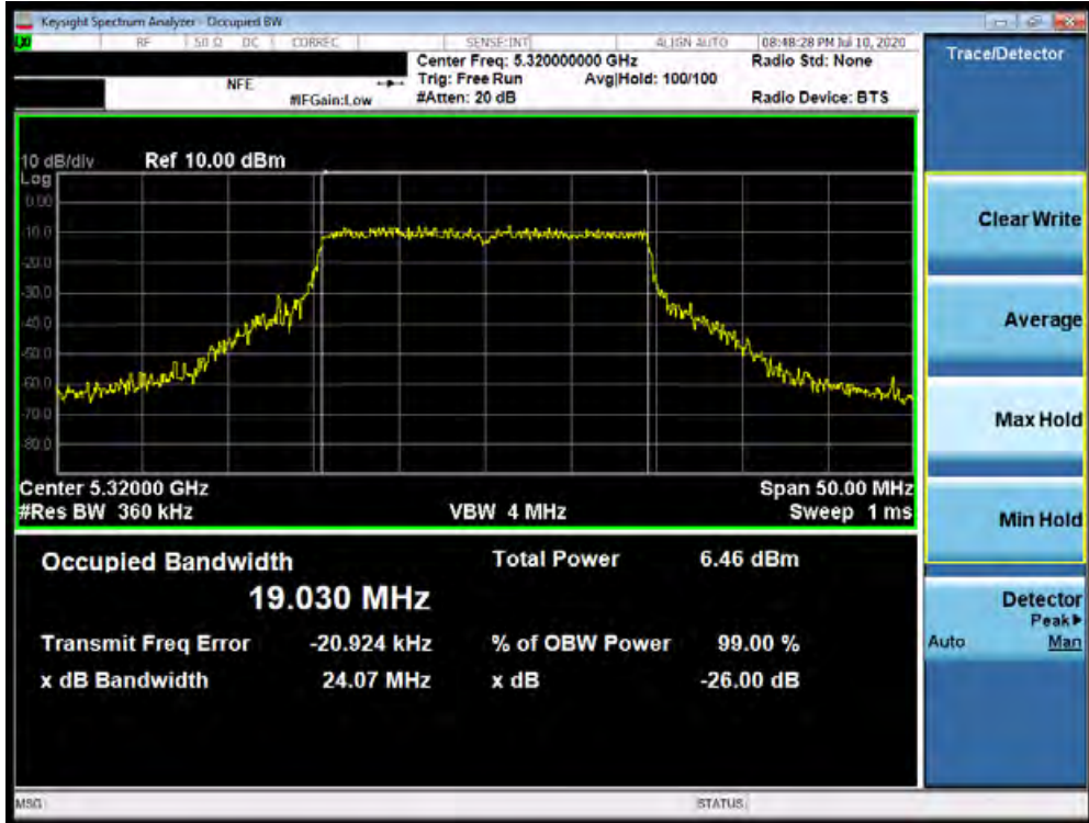
Plot 7-30. 26dB Bandwidth Plot SISO ANT1 (20MHz BW 802.11ax – 242 Tones (UNII Band 2A) – Ch. 64)
