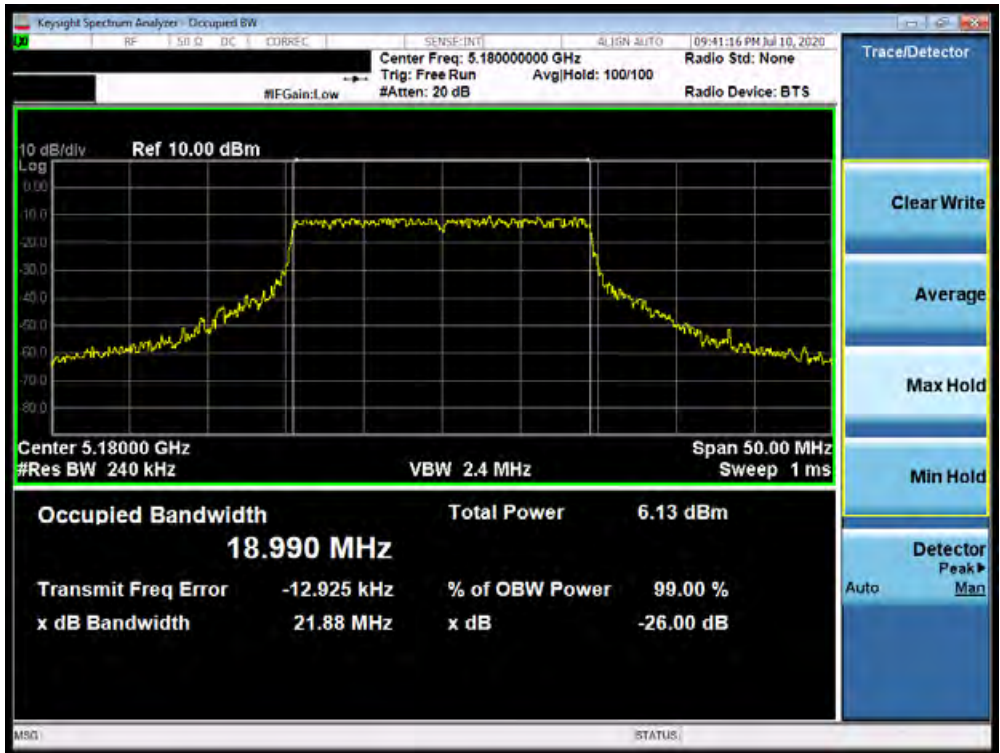
Plot 7-64. 26dB Bandwidth Plot SISO ANT2 (20MHz BW 802.11ax – 242 Tones (UNII Band 1) – Ch. 36)
