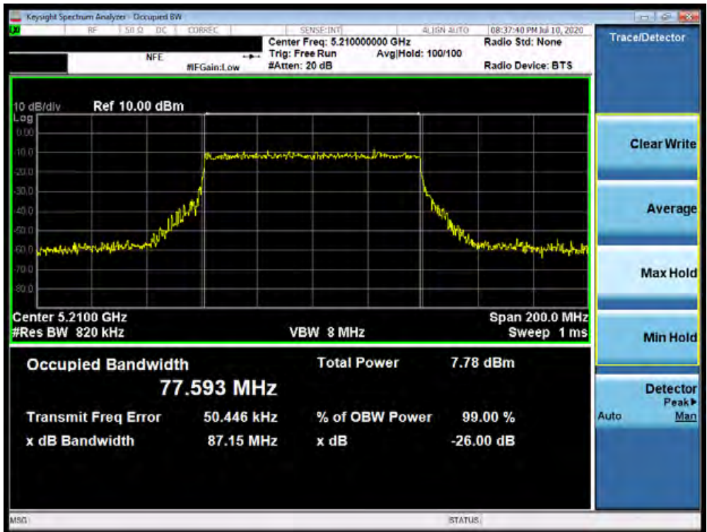
Plot 7-27. 26dB Bandwidth Plot SISO ANT1 (80MHz BW 802.11ax – 996 Tones (UNII Band 1) – Ch. 42)
