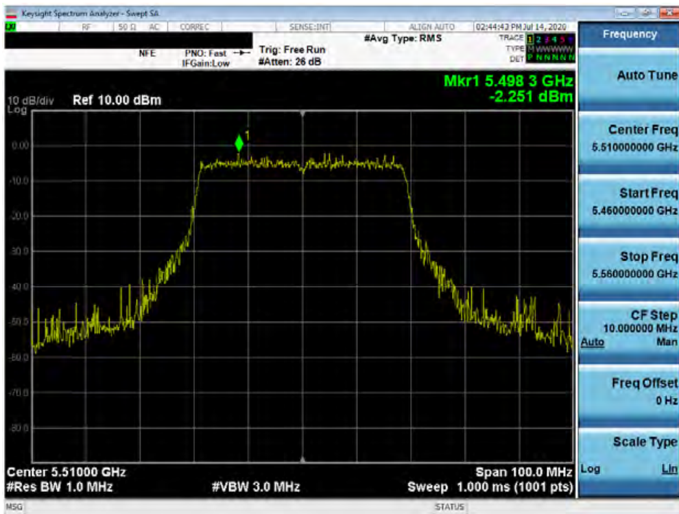
Plot 7-151. Power Spectral Density Plot SISO ANT1 (40MHz BW 802.11ax – Full Tones (UNII Band 2C) – Ch. 102)
