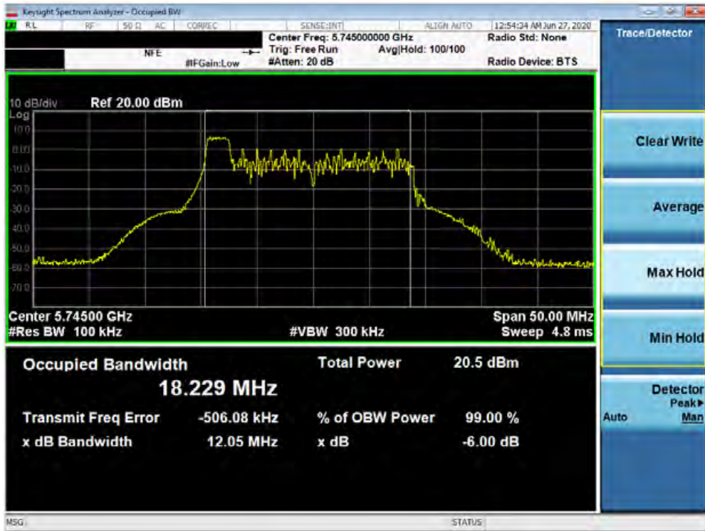
Plot 7-97. 6dB Bandwidth Plot SISO ANT2 (20MHz BW 802.11ax – 26 Tones (UNII Band 3) – Ch. 149)
