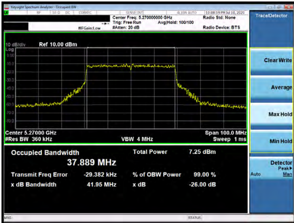
Plot 7-73. 26dB Bandwidth Plot SISO ANT2 (40MHz BW 802.11ax – 484 Tones (UNII Band 2A) – Ch. 54)
