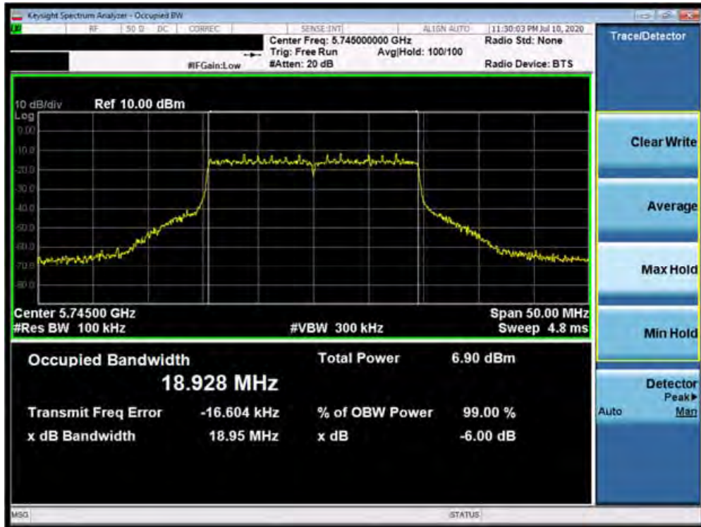
Plot 7-91. 6dB Bandwidth Plot SISO ANT1 (20MHz BW 802.11ax – 242 Tones (UNII Band 3) – Ch. 149)
