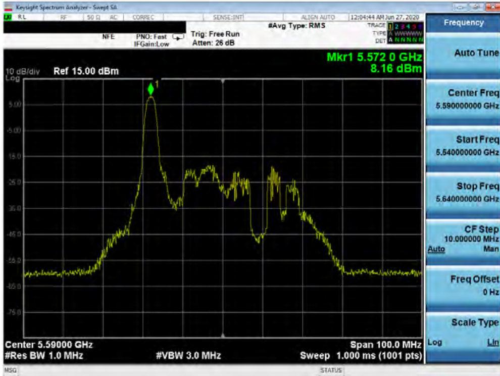
Plot 7-125. Power Spectral Density Plot SISO ANT1 (40MHz BW 802.11ax – 26 Tones (UNII Band 2C) – Ch. 118)
