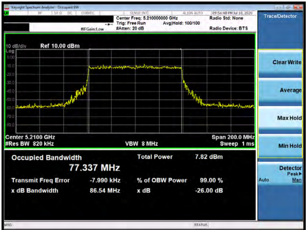
Plot 7-69. 26dB Bandwidth Plot SISO ANT2 (80MHz BW 802.11ax – 996 Tones (UNII Band 1) – Ch. 42)
