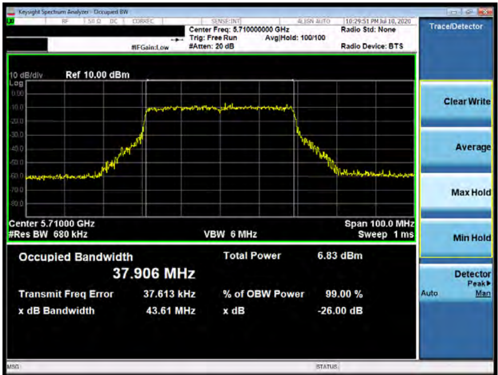
Plot 7-81. 26dB Bandwidth Plot SISO ANT2 (40MHz BW 802.11ax – 484 Tones (UNII Band 2C) – Ch. 142)
