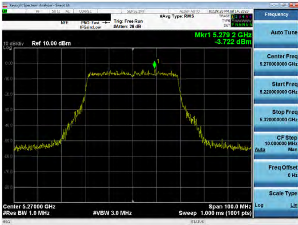
Plot 7-145. Power Spectral Density Plot SISO ANT1 (40MHz BW 802.11ax – Full Tones (UNII Band 2A) – Ch. 54)
