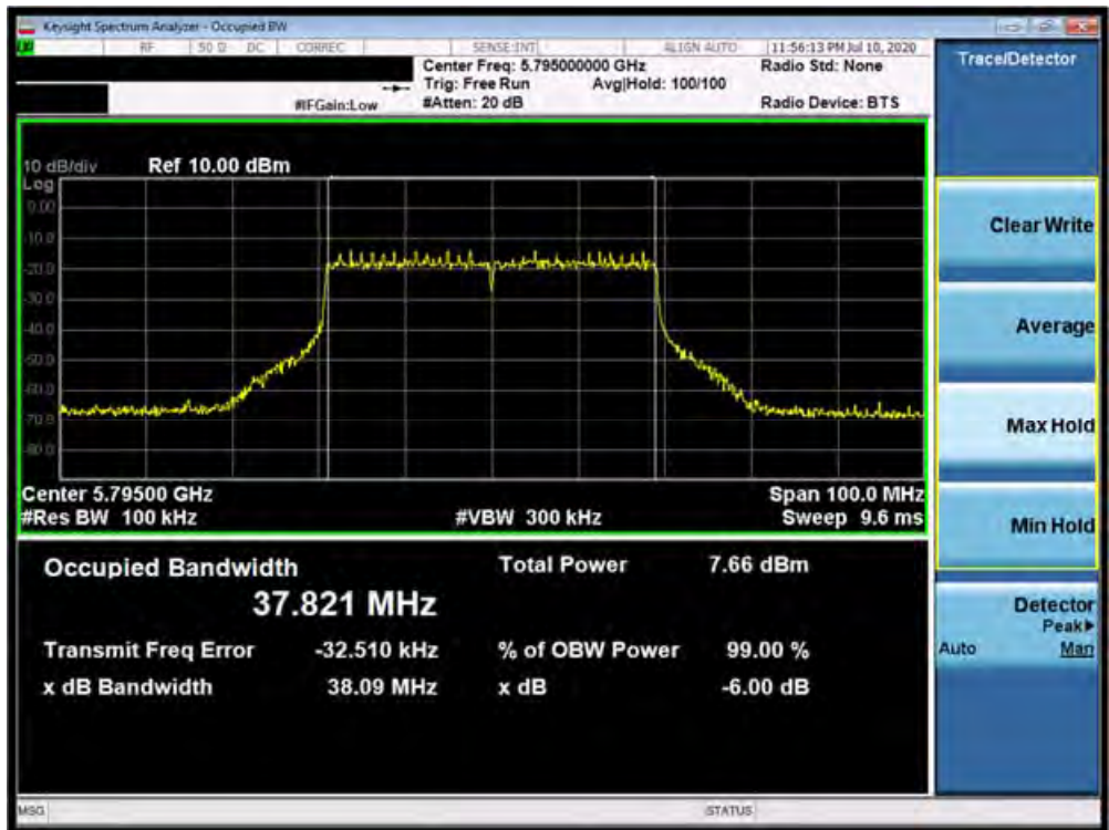
Plot 7-107. 6dB Bandwidth Plot SISO ANT2 (40MHz BW 802.11ax – 484 Tones (UNII Band 3) – Ch. 159)
