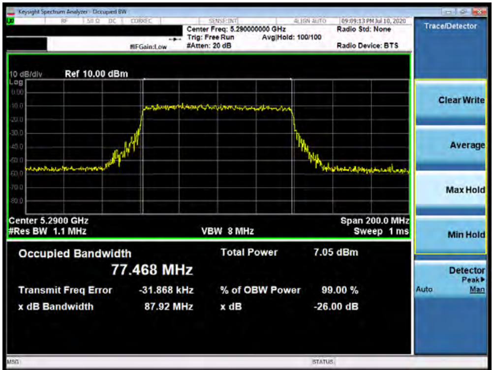
Plot 7-33. 26dB Bandwidth Plot SISO ANT1 (80MHz BW 802.11ax – 996 Tones (UNII Band 2A) – Ch. 58)
