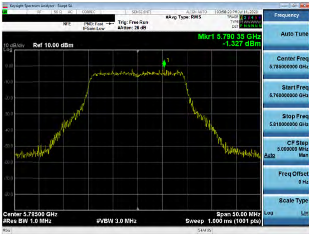
Plot 7-158. Power Spectral Density Plot SISO ANT1 (20MHz BW 802.11ax – Full Tones (UNII Band 3) – Ch. 157)
