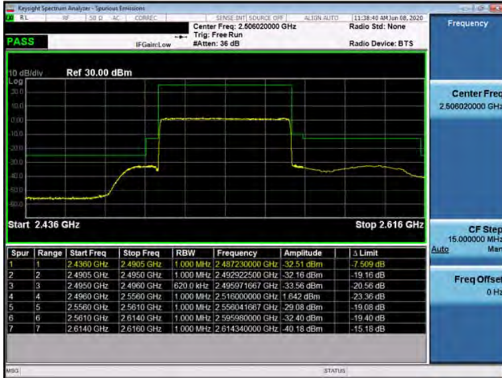
Plot 7-549. Lower ACP Plot at 2496 MHz (n41 - 60.0MHz DFT-s-OFDM-QPSK - Full RB Configuration)
