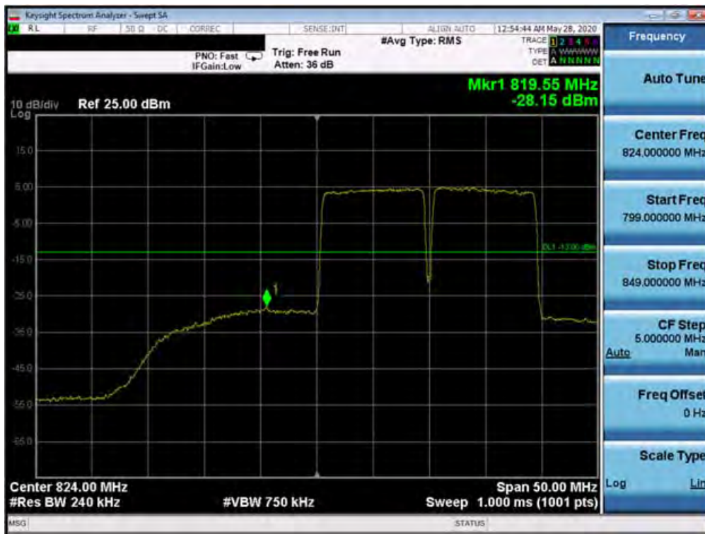
Plot 7-653. Lower Band Edge Plot (Band 5 QPSK – PCC:10 MHz SCC:10 MHz – Full RB)
