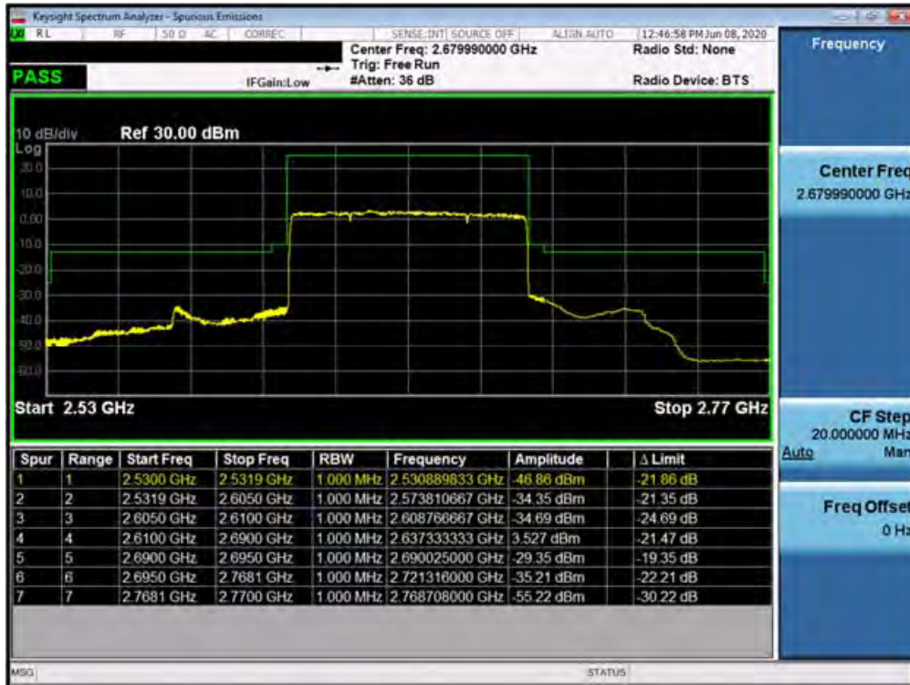
Plot 7-552. Upper ACP Plot (Band 41 - 80.0MHz DFT-s-OFDM-QPSK - Full RB Configuration)
