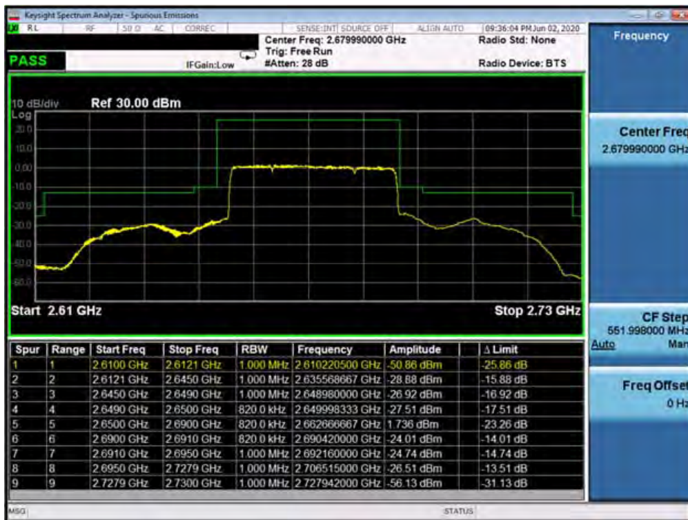
Plot 7-546. Upper ACP Plot (Band 41 - 40.0MHz DFT-s-OFDM-QPSK - Full RB Configuration)
