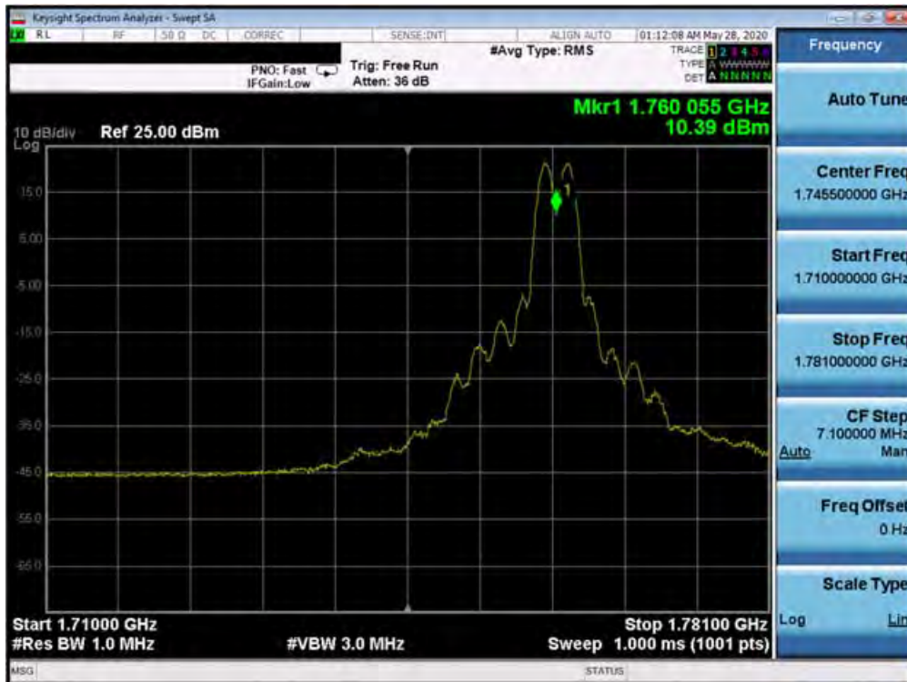
Plot 7-664. Conducted Spurious Plot (Band 66 – 20.0MHz QPSK – PCC 1/0 SCC 1/99 – High Channel)
