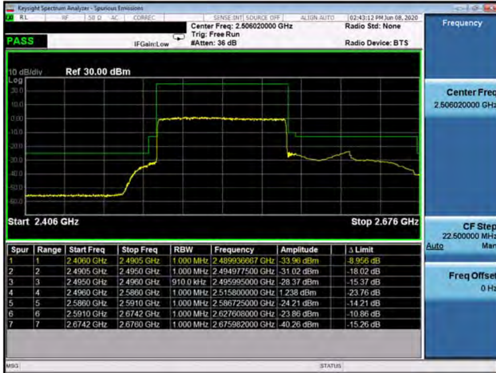
Plot 7-553. Lower ACP Plot at 2496 MHz (n41 - 90.0MHz DFT-s-OFDM-QPSK - Full RB Configuration)
