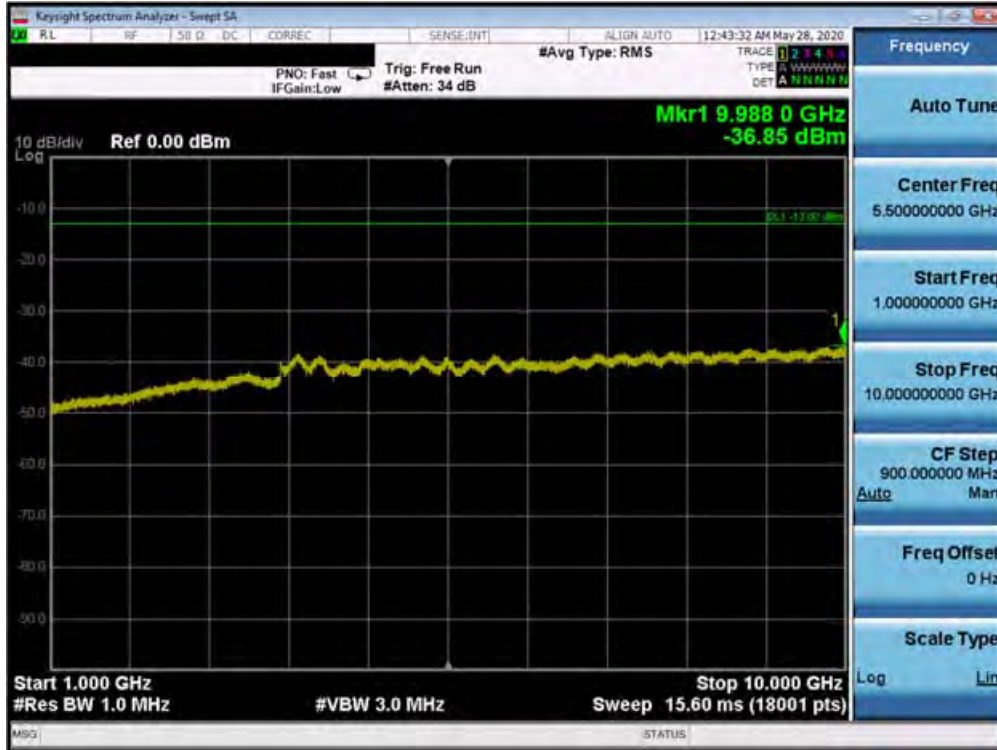
Plot 7-648. Conducted Spurious Plot (Band 5 – 10.0MHz QPSK – PCC 1/49 SCC 1/0 – Low Channel)
