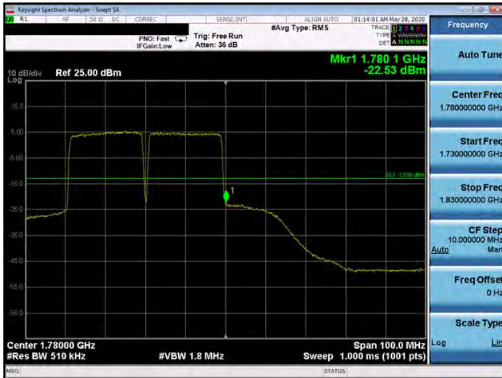
Plot 7-669. Upper Band Edge Plot (Band 66 QPSK – PCC:20 MHz SCC:20 MHz – Full RB)
