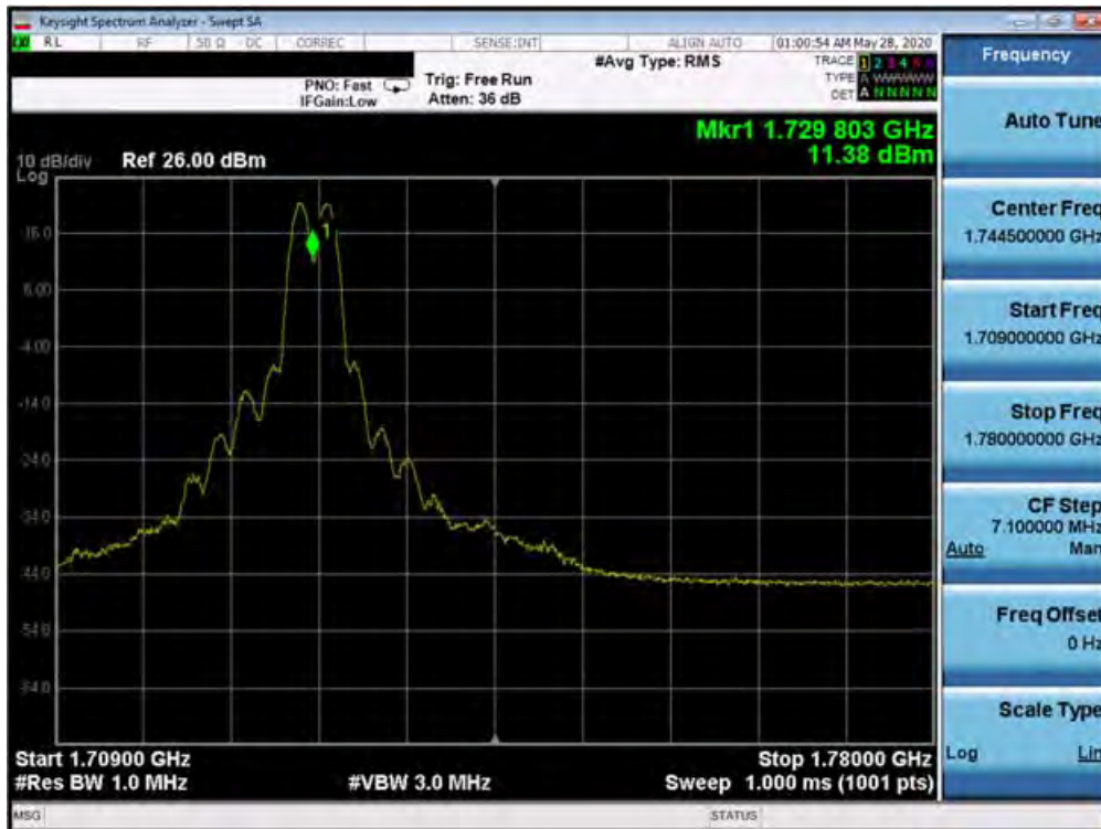
Plot 7-656. Conducted Spurious Plot (Band 66 – 20.0MHz QPSK – PCC 1/99 SCC 1/0 – Low Channel)
