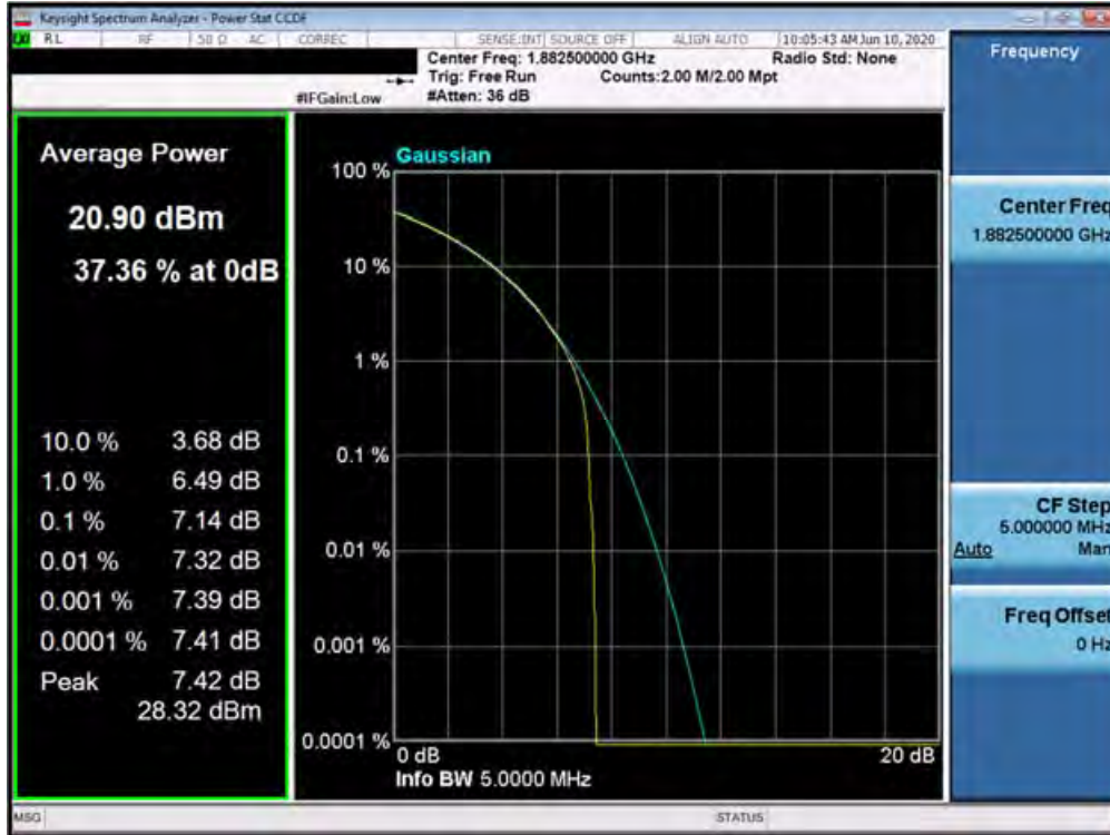
Plot 7-583. PAR Plot (Band n25/2 - 5.0MHz 16-QAM - Full RB Configuration)
