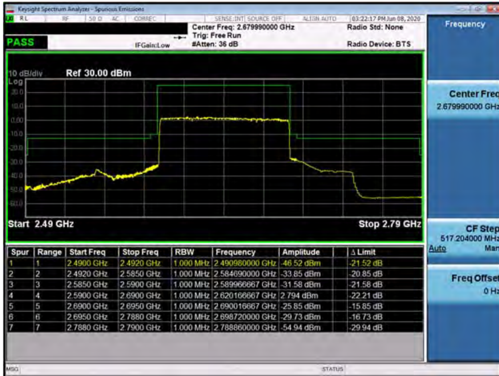
Plot 7-556. Upper ACP Plot (Band n41 - 100.0MHz DFT-s-OFDM-QPSK - Full RB Configuration)
