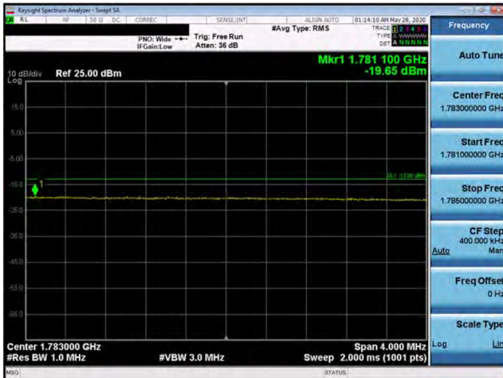
Plot 7-670. Extended Upper Band Edge Plot (Band 66 QPSK – PCC:20 MHz SCC:20 MHz – Full RB)
