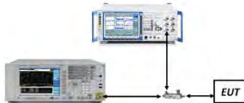
Figure 7-4. Test Instrument & Measurement Setup
