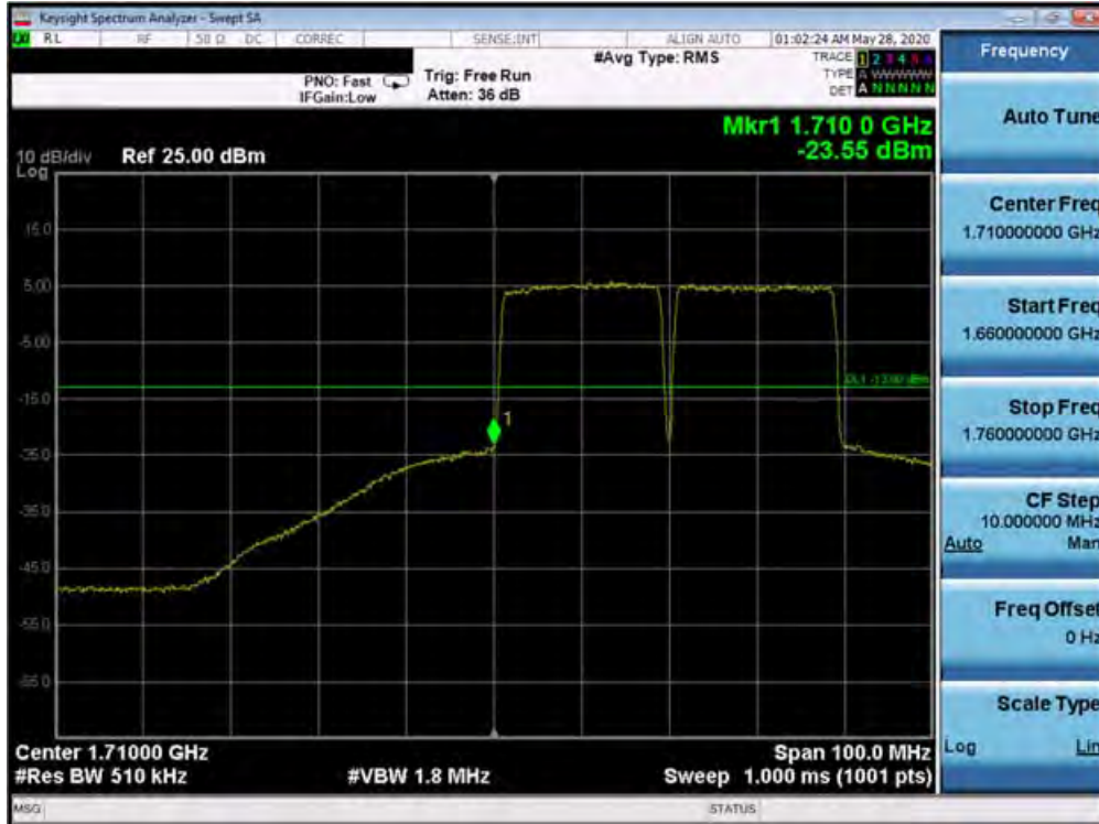
Plot 7-667. Lower Band Edge Plot (Band 66 QPSK – PCC:20 MHz SCC:20 MHz – Full RB)
