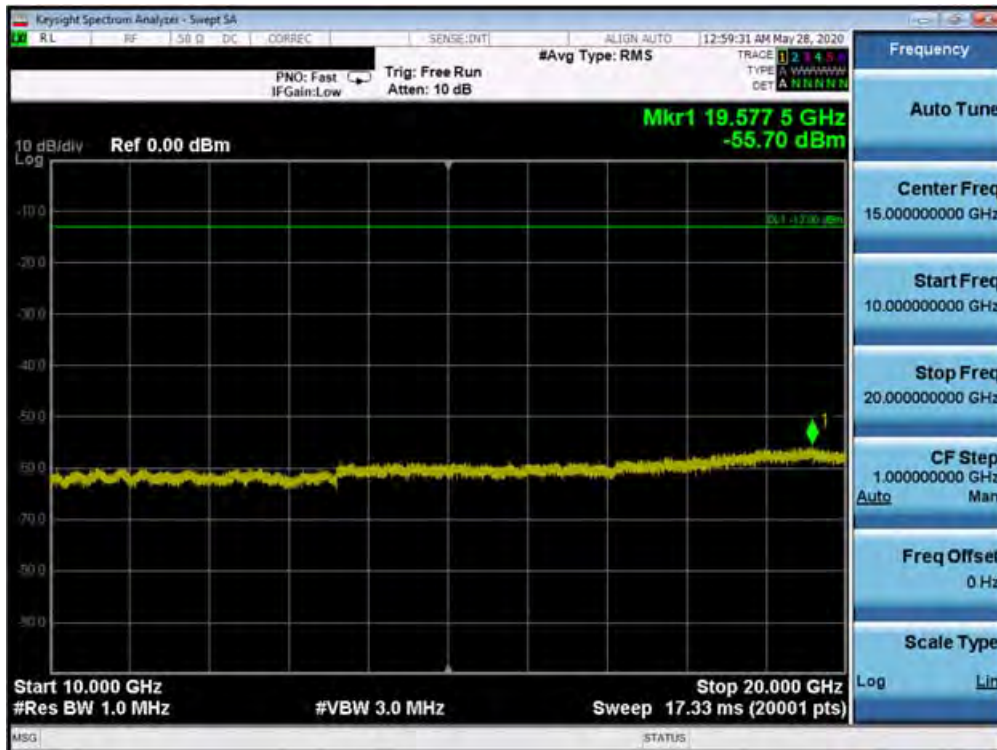
Plot 7-658. Conducted Spurious Plot (Band 66 – 20.0MHz QPSK – PCC 1/99 SCC 1/0 – Low Channel)
