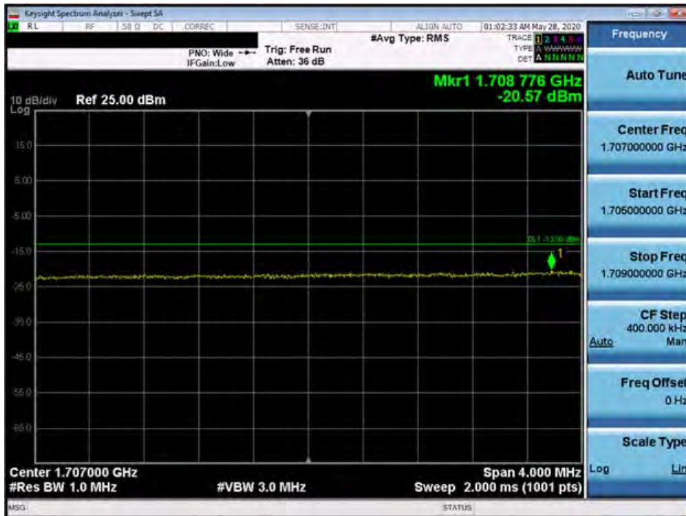
Plot 7-668. Extended Lower Band Edge Plot (Band 66 QPSK – PCC:20 MHz SCC:20 MHz – Full RB)
