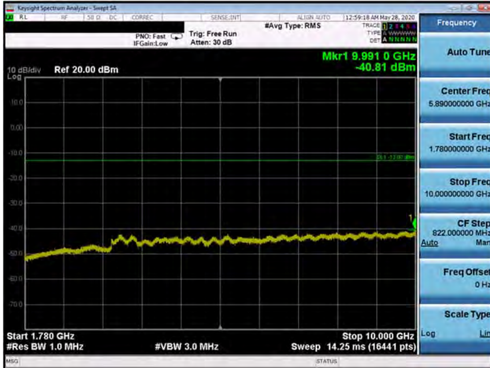
Plot 7-657. Conducted Spurious Plot (Band 66 – 20.0MHz QPSK – PCC 1/99 SCC 1/0 – Low Channel)
