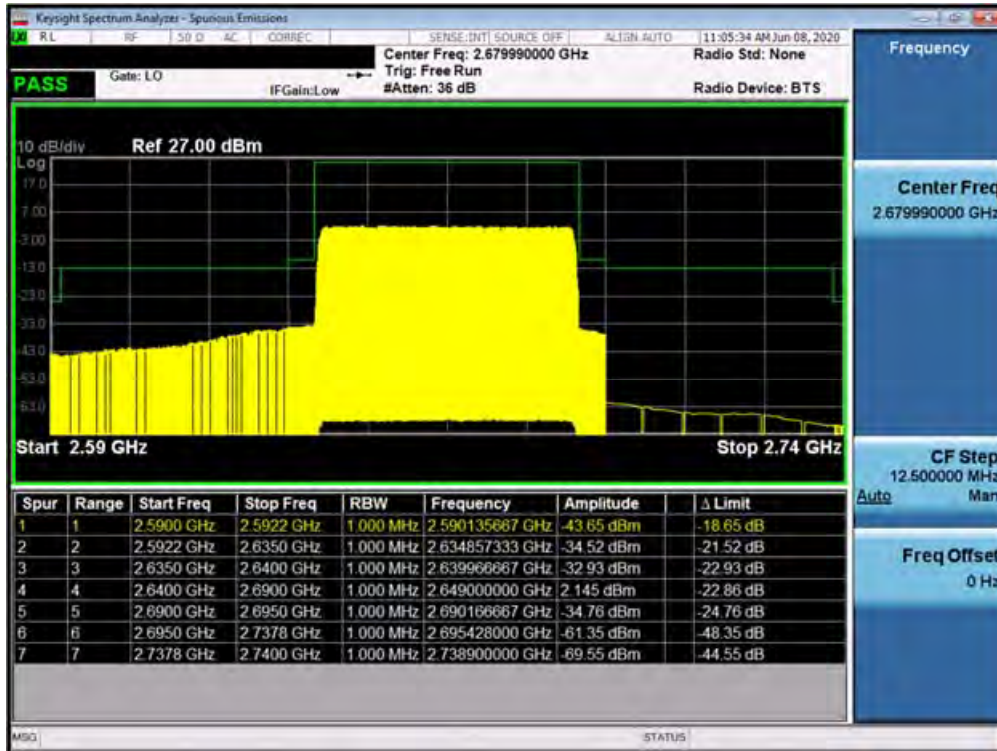
Plot 7-548. Upper ACP Plot (Band 41 - 50.0MHz DFT-s-OFDM-QPSK - Full RB Configuration)
