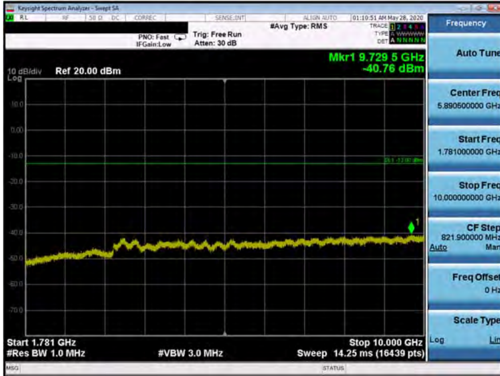
Plot 7-665. Conducted Spurious Plot (Band 66 – 20.0MHz QPSK – PCC 1/0 SCC 1/99 – High Channel)
