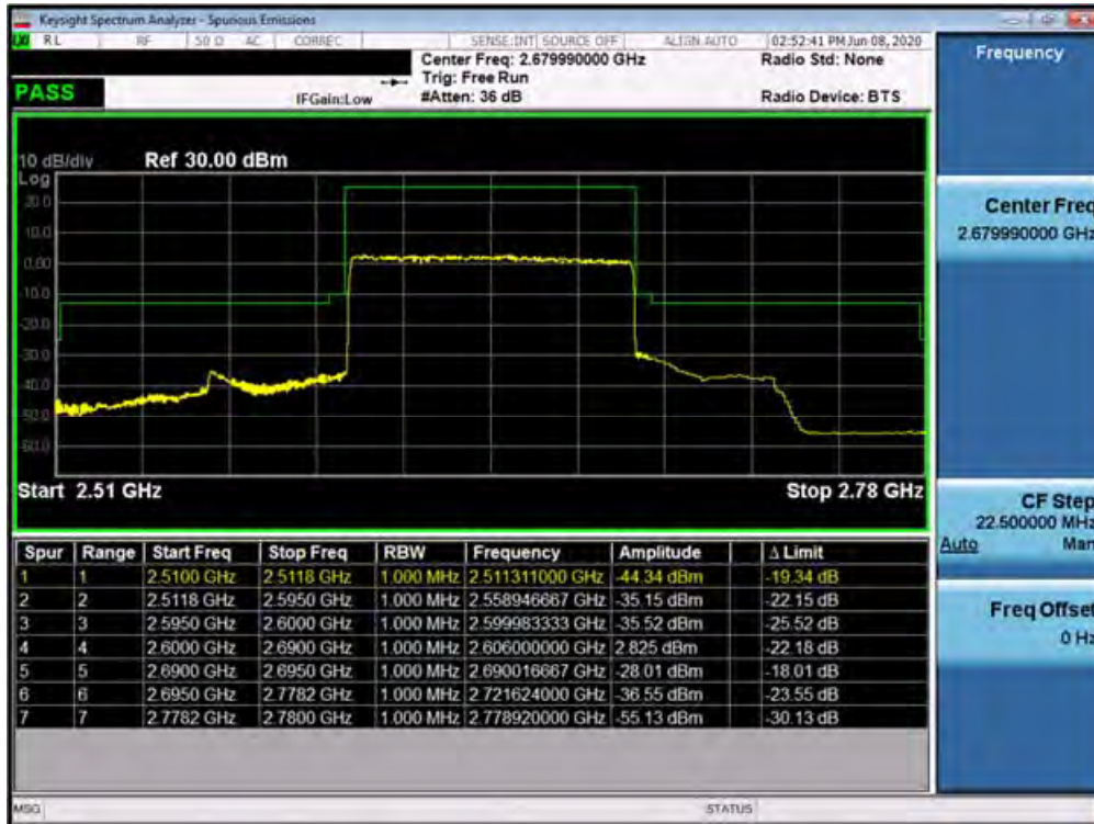
Plot 7-554. Upper ACP Plot (Band 41 - 90.0MHz DFT-s-OFDM-QPSK - Full RB Configuration)
