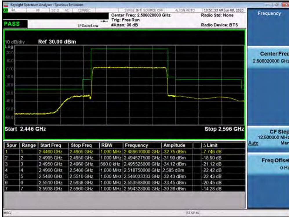
Plot 7-547. Lower ACP Plot at 2496 MHz (n41 - 50.0MHz DFT-s-OFDM-QPSK - Full RB Configuration)
