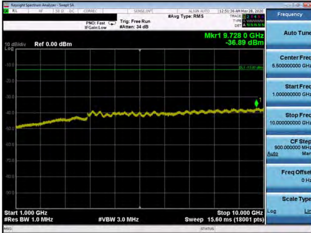
Plot 7-652. Conducted Spurious Plot (Band 5 – 10.0MHz QPSK – PCC 1/0 SCC 1/49 – High Channel)
