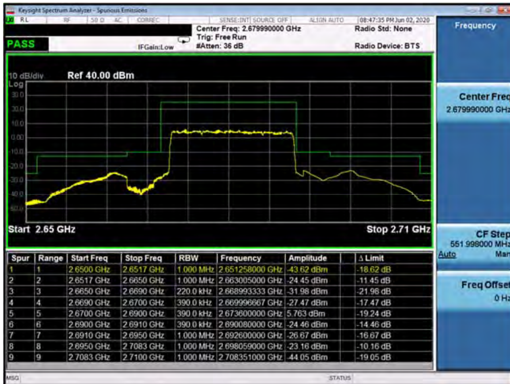
Plot 7-544. Upper ACP Plot (Band 41 - 20.0MHz DFT-s-OFDM-QPSK - Full RB Configuration)
