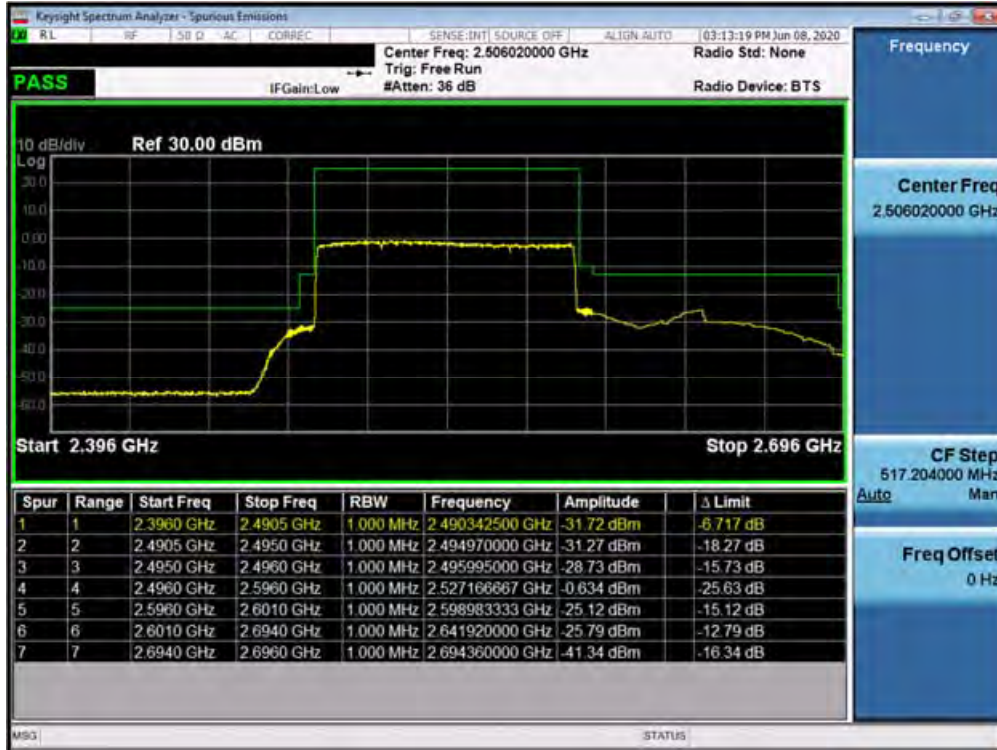
Plot 7-555. Lower ACP Plot at 2496 MHz (n41 - 100.0MHz DFT-s-OFDM-QPSK - Full RB Configuration)
