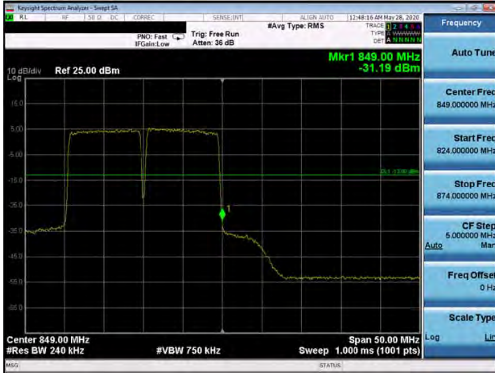
Plot 7-654. Upper Band Edge Plot (Band 5 QPSK – PCC:10 MHz SCC:10 MHz – Full RB)
