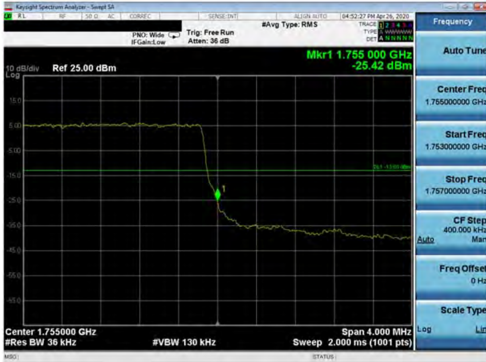
Plot 7-423. Upper Band Edge Plot (Band 4 - 3.0MHz QPSK - Full RB Configuration)
