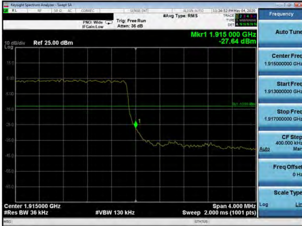
Plot 7-477. Upper Band Edge Plot (Band 25 - 3.0MHz QPSK - Full RB Configuration)
