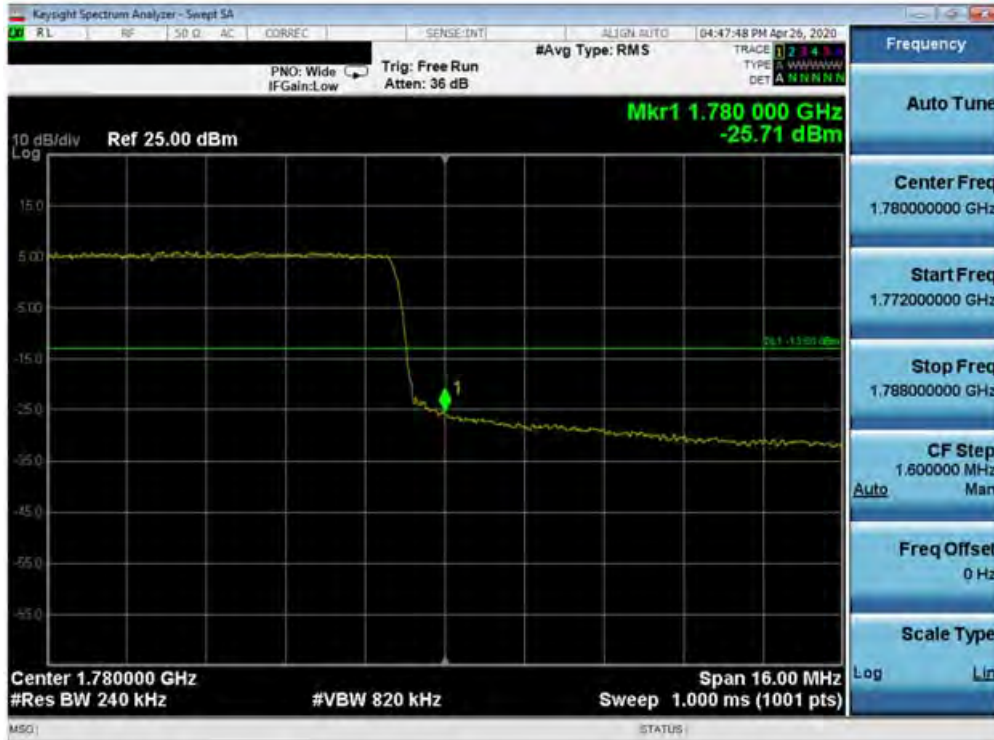
Plot 7-449. Upper Band Edge Plot (Band 66 - 20.0MHz QPSK - Full RB Configuration)
