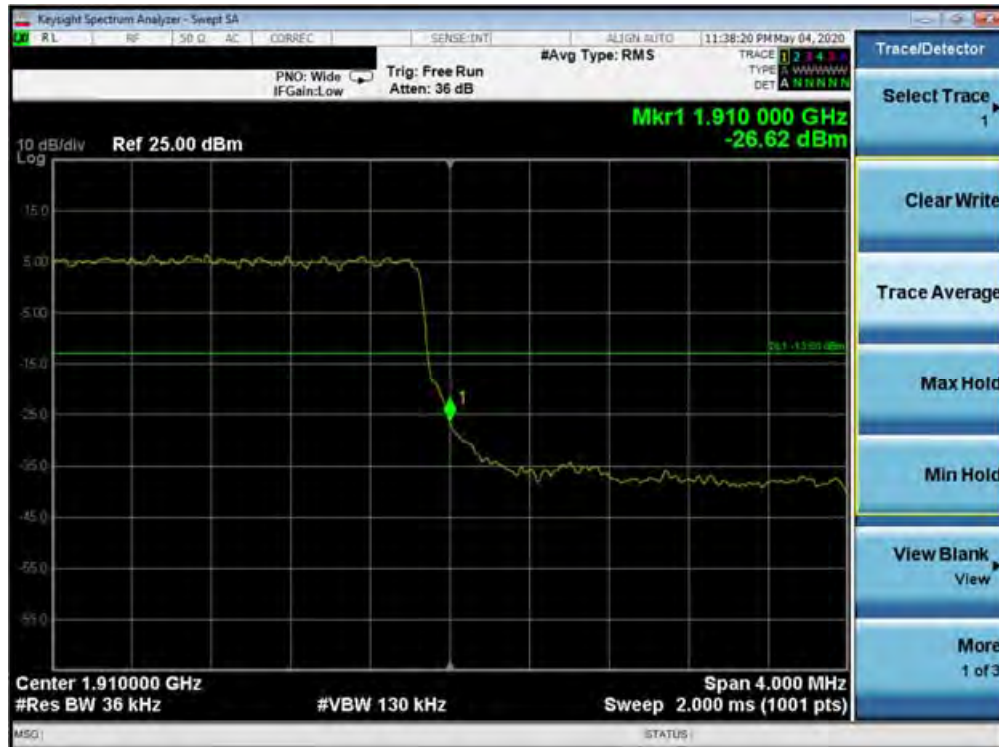
Plot 7-475. Upper Band Edge Plot (Band 2 - 3.0MHz QPSK - Full RB Configuration)
