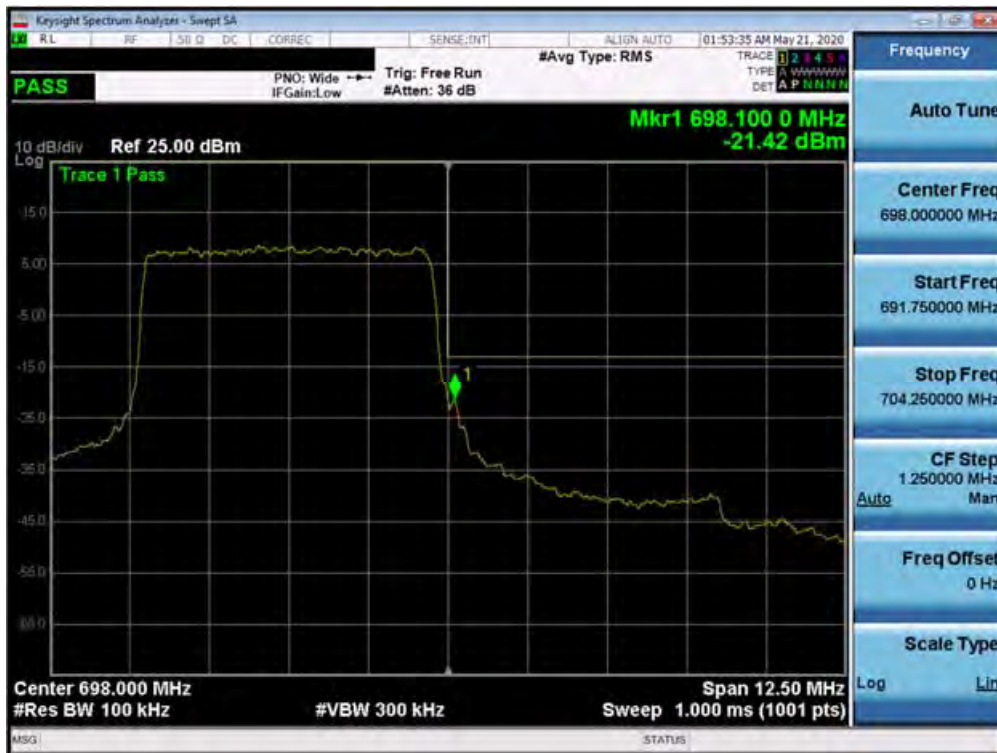
Plot 7-376. Upper Band Edge Plot (n71 - 5MHz DFT-s-OFDM-QPSK - Full RB Configuration)
