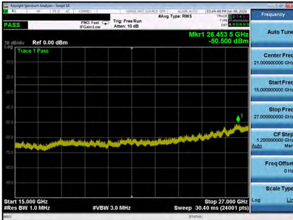
Plot 7-363. Conducted Spurious Plot (n41 - 100MHz DFT-s-OFDM-QPSK - RB Size 1, RB Offset 1 - Mid Channel)
