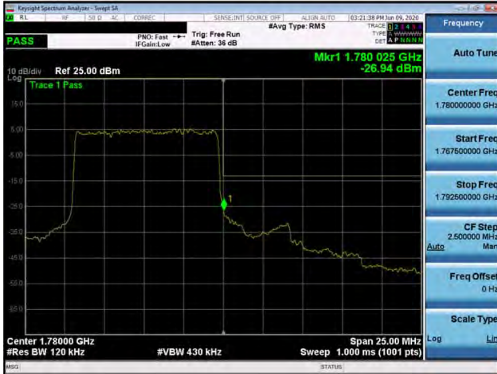
Plot 7-457. Upper Band Edge Plot (n66 - 10MHz DFT-s-OFDM-QPSK - Full RB Configuration)
