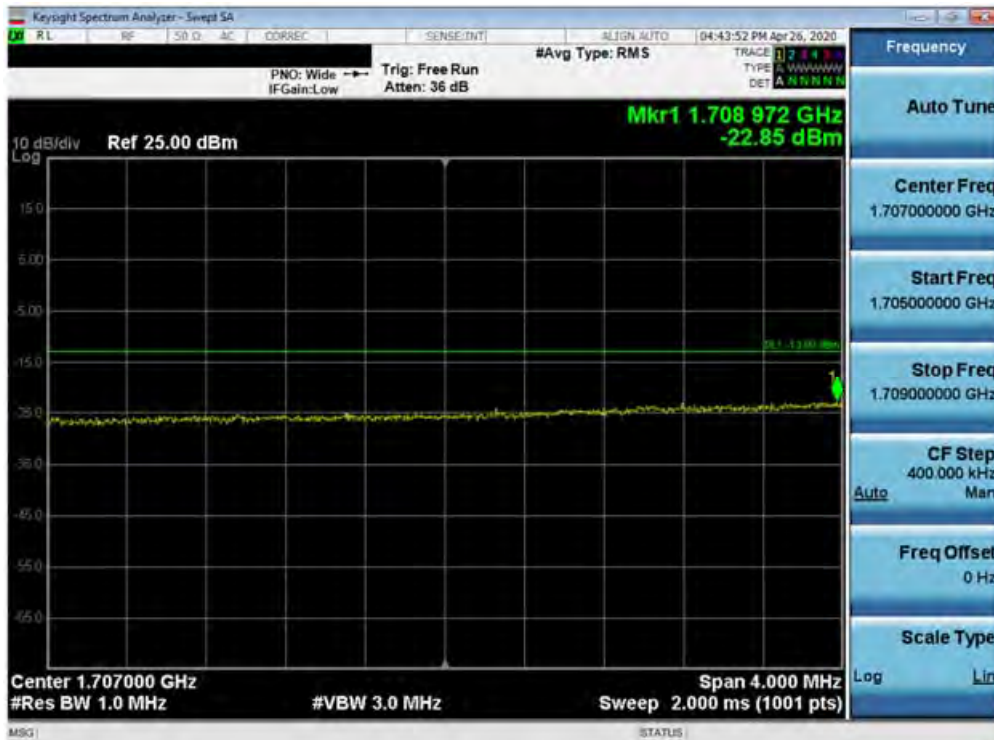
Plot 7-440. Lower Extended Band Edge Plot (Band 66/4 - 15.0MHz QPSK - Full RB Configuration)
