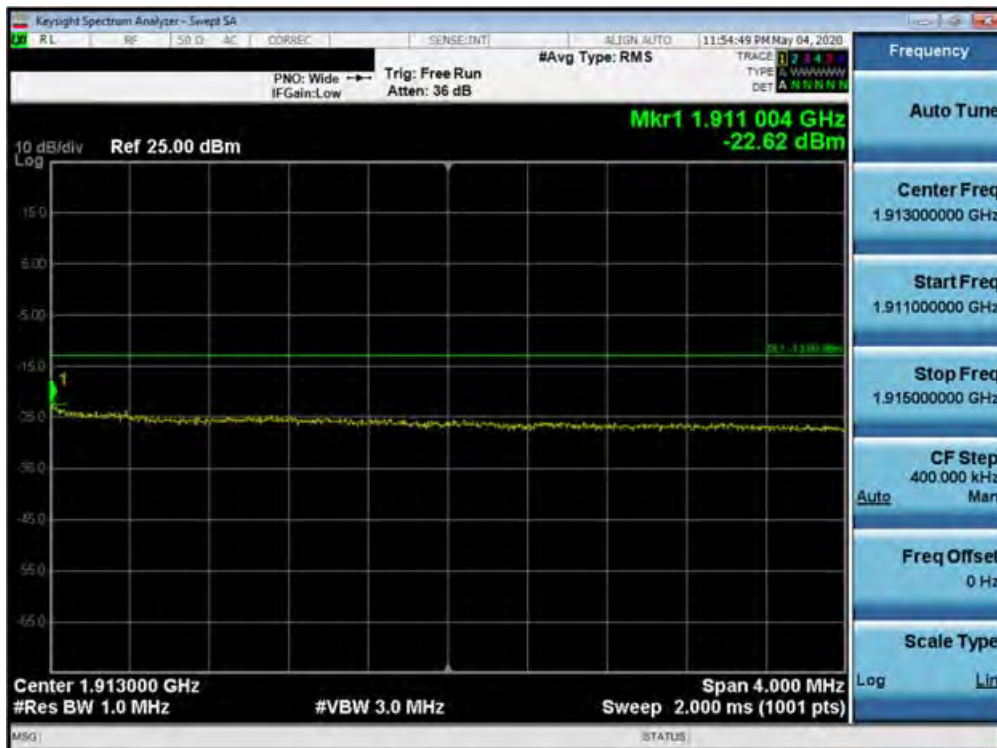
Plot 7-488. Upper Extended Band Edge Plot (Band 2 - 10.0MHz QPSK - Full RB Configuration)
