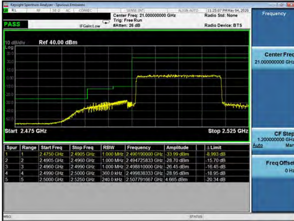
Plot 7-533. Lower ACP Plot (Band 7 - 20.0MHz QPSK - Full RB Configuration)
