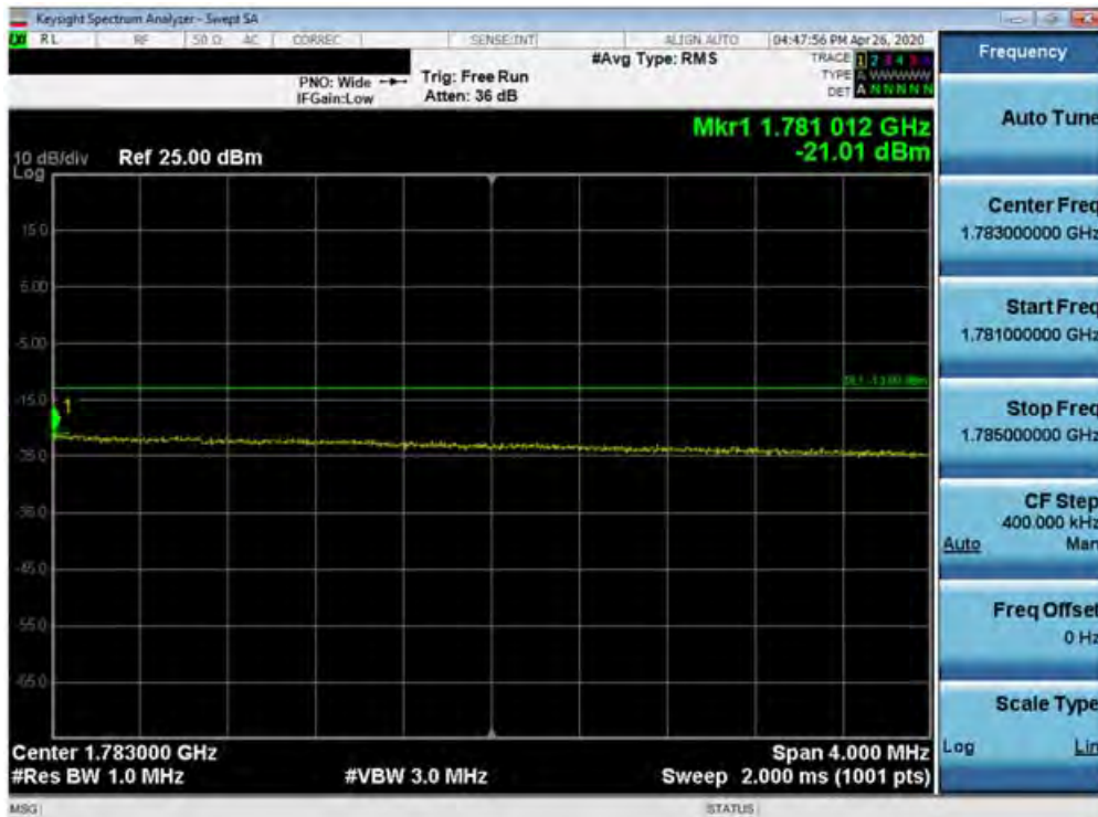
Plot 7-450. Upper Extended Band Edge Plot (Band 66 - 20.0MHz QPSK - Full RB Configuration)
