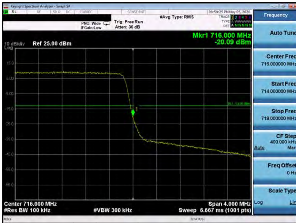
Plot 7-386. Upper Band Edge Plot (Band 12 - 3.0MHz QPSK - Full RB Configuration)
