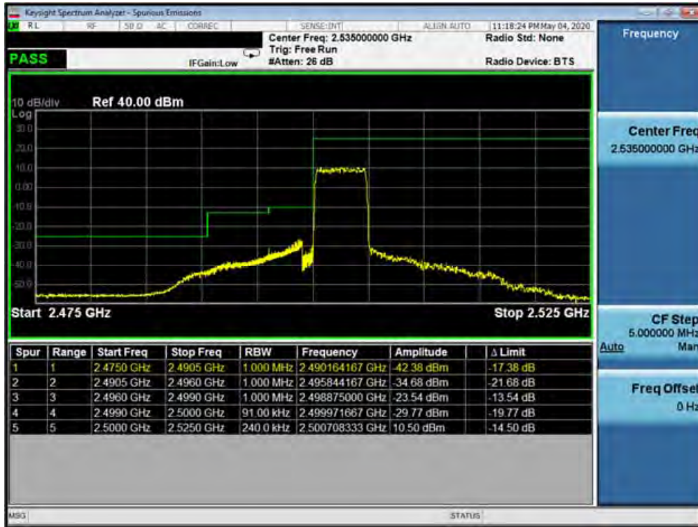
Plot 7-527. Lower ACP Plot (Band 7 - 5.0MHz QPSK - Full RB Configuration)
