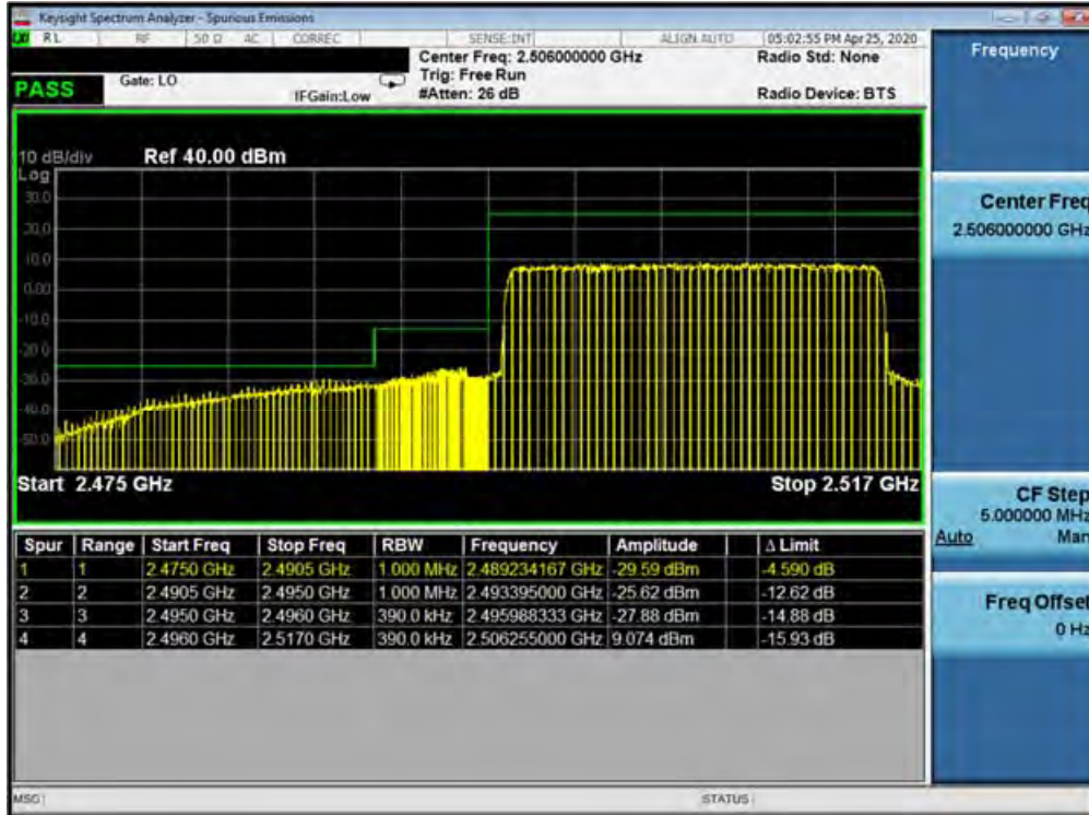
Plot 7-541. Lower ACP Plot at 2496 MHz (Band 41 (PC2) - 20.0MHz QPSK - Full RB Configuration)
