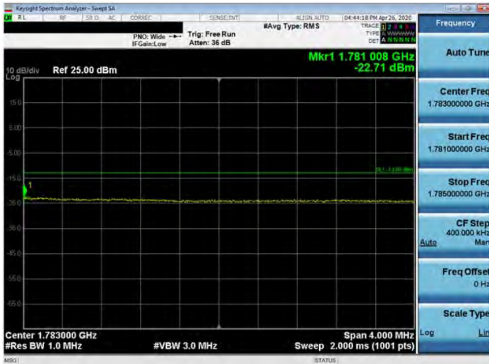
Plot 7-444. Upper Extended Band Edge Plot (Band 66 - 15.0MHz QPSK - Full RB Configuration)
