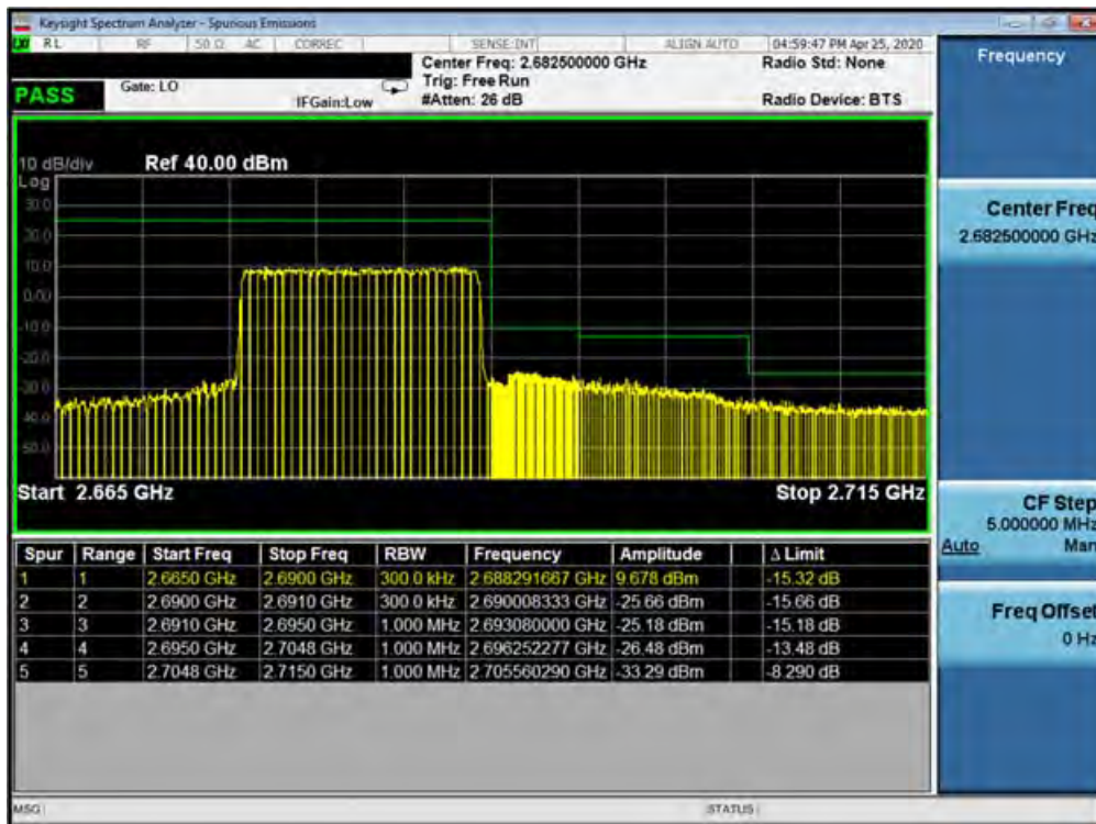
Plot 7-540. Upper ACP Plot (Band 41 (PC2) - 15.0MHz QPSK - Full RB Configuration)
