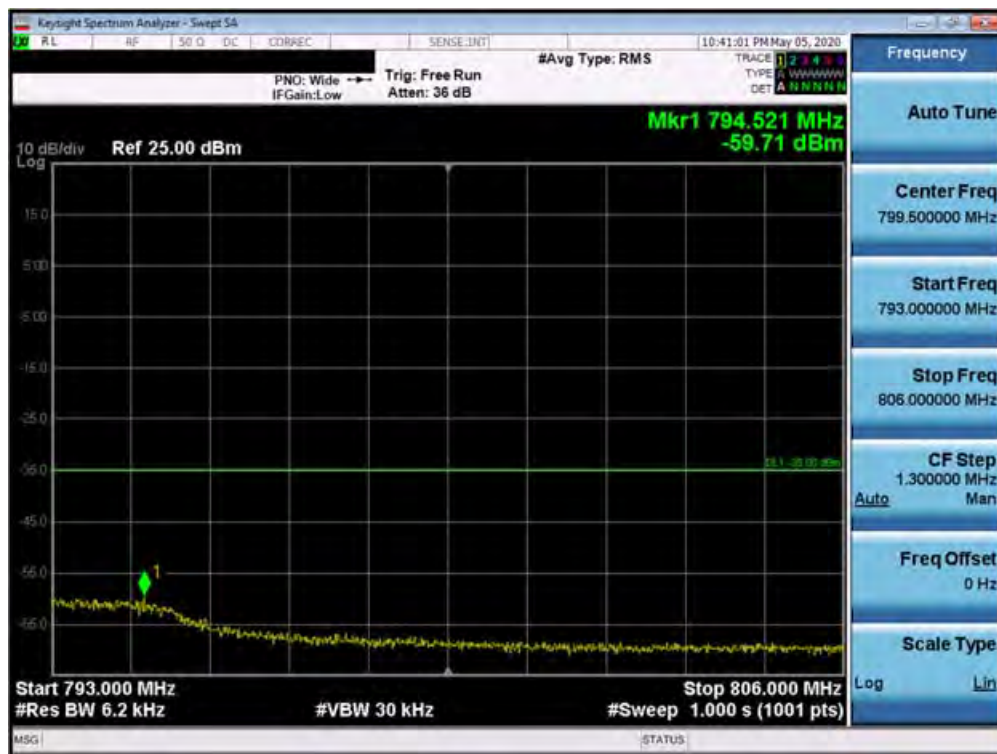
Plot 7-394. Upper Emission Mask Plot (Band 13 - 5.0MHz QPSK - Full RB Configuration)
