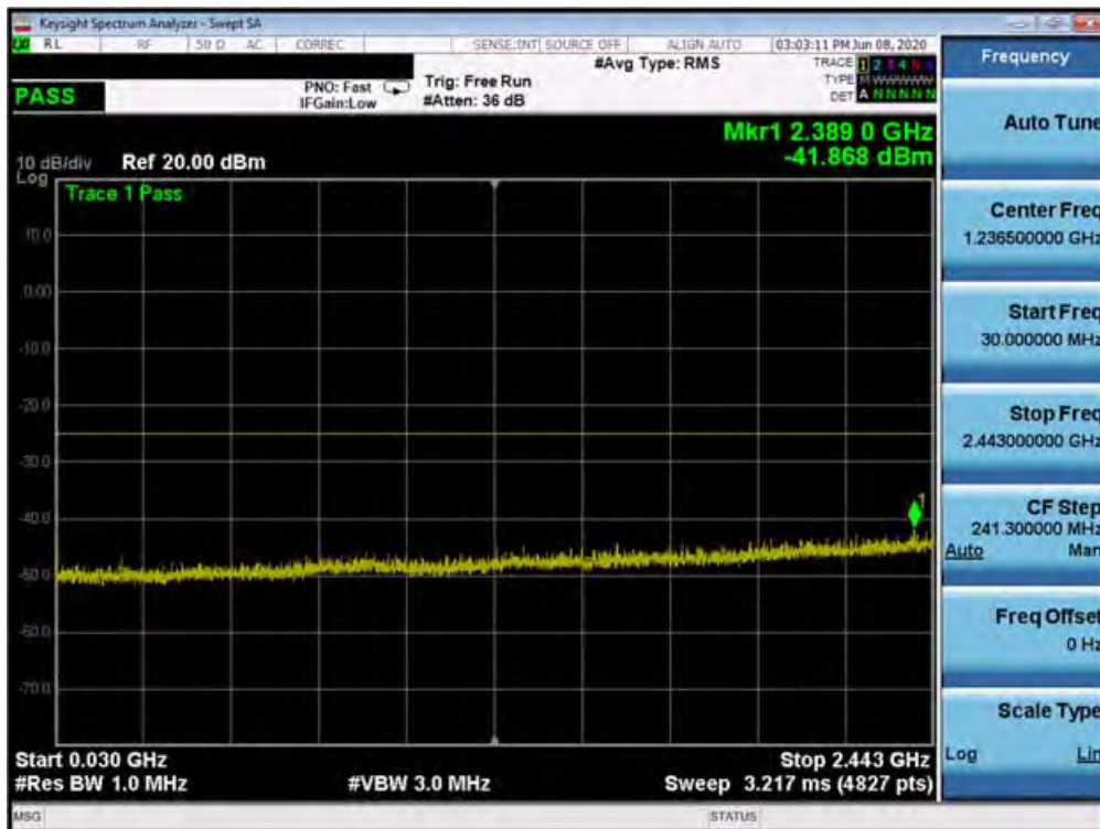
Plot 7-361. Conducted Spurious Plot (n41 - 100MHz DFT-s-OFDM-QPSK - RB Size 1, RB Offset 1 - Mid Channel)
