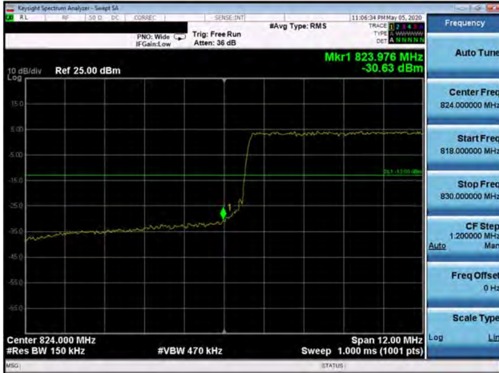
Plot 7-405. Lower Band Edge Plot (Band 26 - 15.0MHz QPSK - Full RB Configuration)
