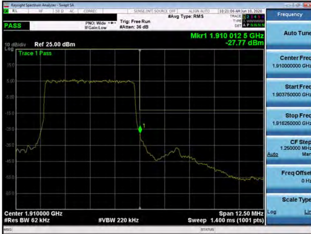
Plot 7-507. Upper Band Edge Plot (n25 - 5MHz DFT-s-OFDM-QPSK - Full RB Configuration)
