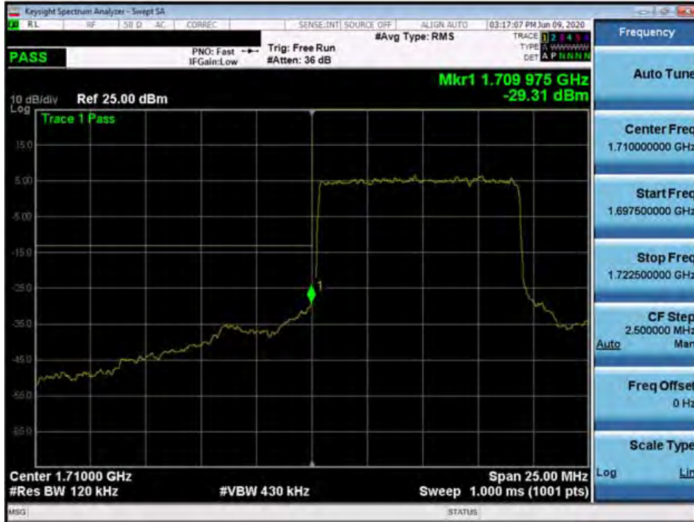
Plot 7-455. Lower Band Edge Plot (n66 - 10MHz DFT-s-OFDM-QPSK - Full RB Configuration)
