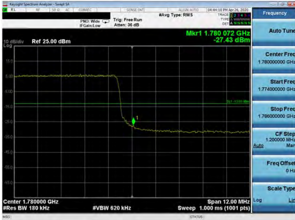
Plot 7-443. Upper Band Edge Plot (Band 66 - 15.0MHz QPSK - Full RB Configuration)
