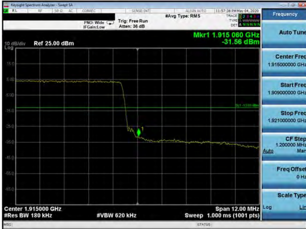
Plot 7-495. Upper Band Edge Plot (Band 25 - 15.0MHz QPSK - Full RB Configuration)
