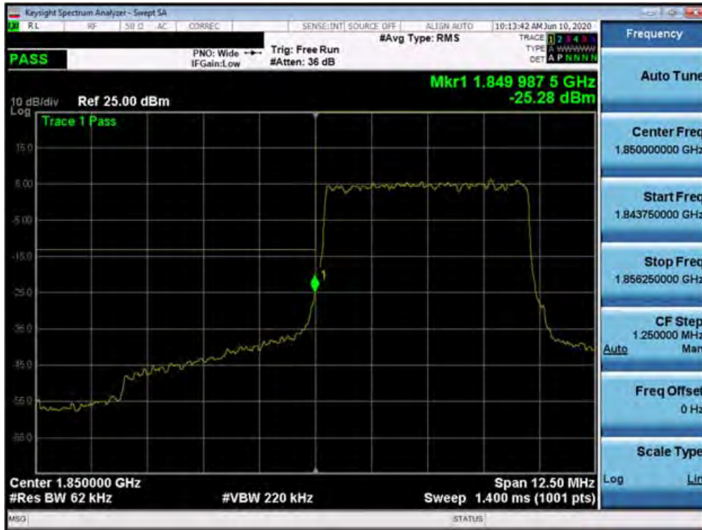
Plot 7-503. Lower Band Edge Plot (n25/2 - 5MHz DFT-s-OFDM-QPSK - Full RB Configuration)
