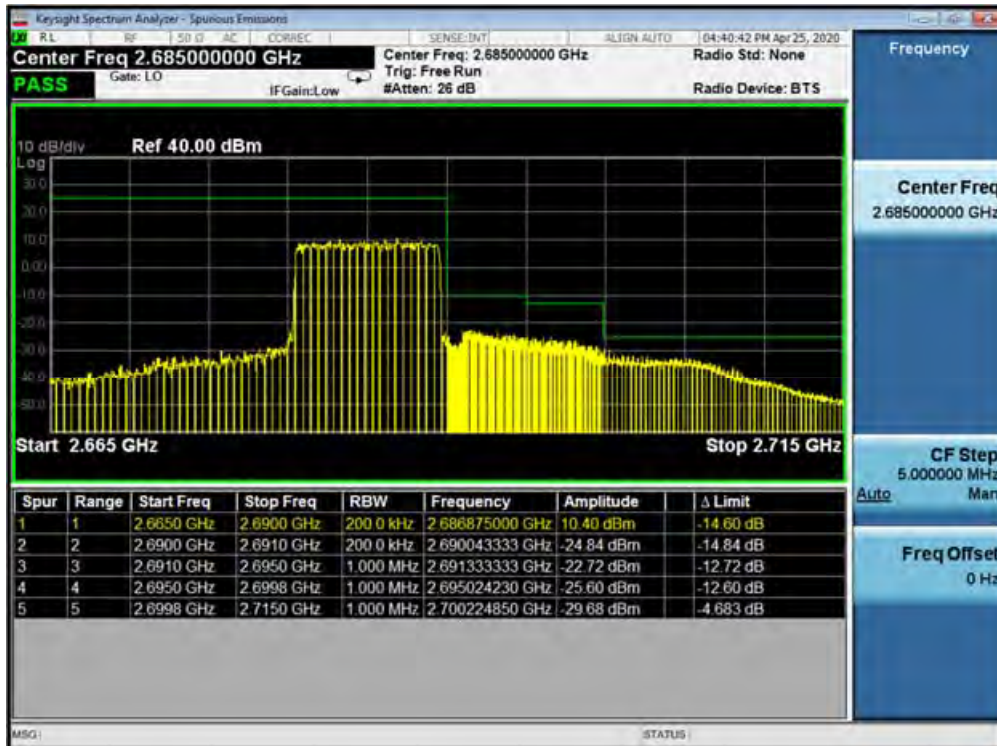
Plot 7-538. Upper ACP Plot (Band 41 (PC2) - 10.0MHz QPSK - Full RB Configuration)
