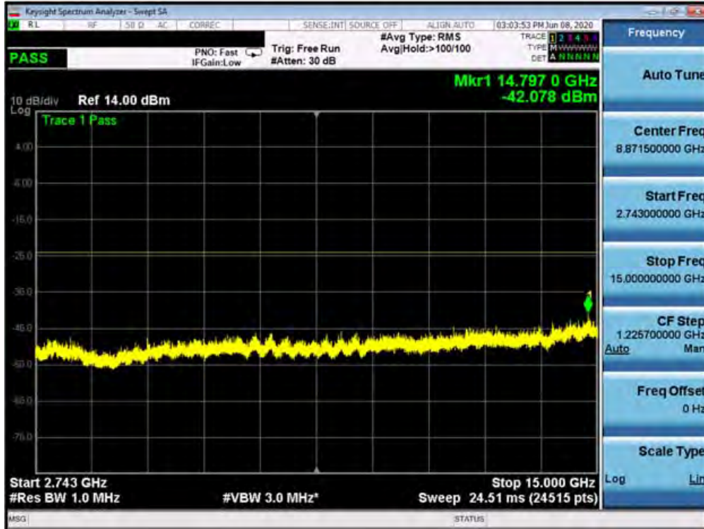
Plot 7-362. Conducted Spurious Plot (n41 - 100MHz DFT-s-OFDM-QPSK - RB Size 1, RB Offset 1 - Mid Channel)
