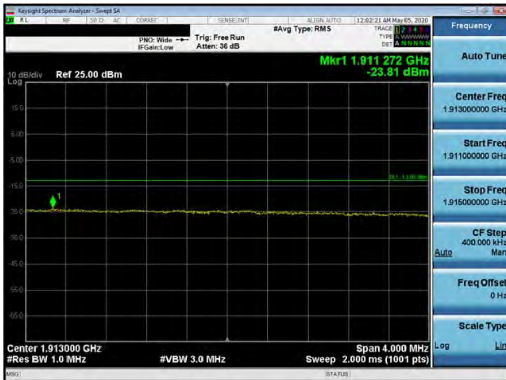
Plot 7-500. Upper Extended Band Edge Plot (Band 2 - 20.0MHz QPSK - Full RB Configuration)
