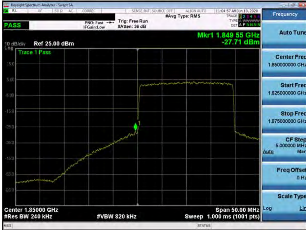
Plot 7-521. Lower Band Edge Plot (n25/2 - 20MHz DFT-s-OFDM-QPSK - Full RB Configuration)
