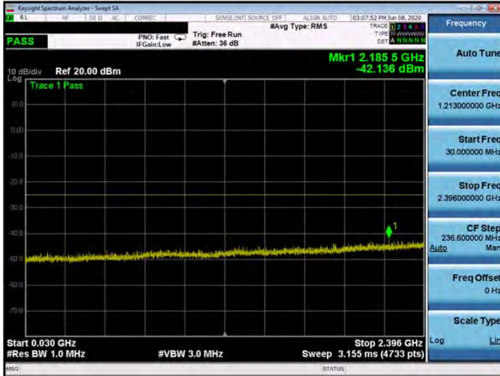
Plot 7-358. Conducted Spurious Plot (n41 - 100MHz DFT-s-OFDM-QPSK - RB Size 1, RB Offset 1 - Low Channel)
