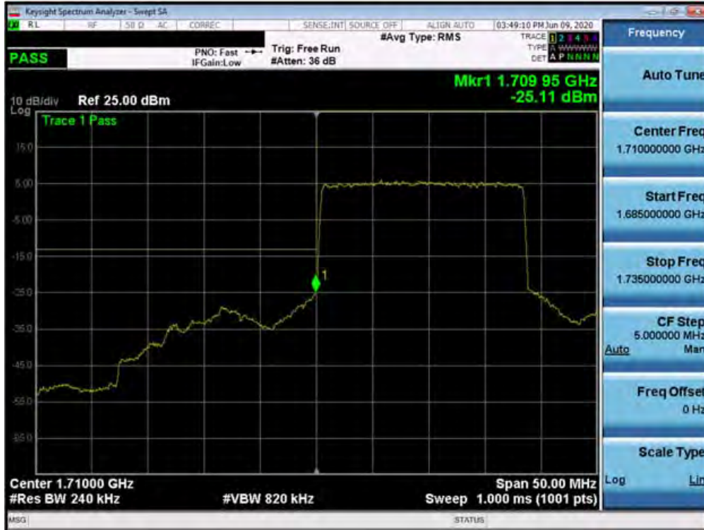
Plot 7-463. Lower Band Edge Plot (n66 - 20MHz DFT-s-OFDM-QPSK - Full RB Configuration)
