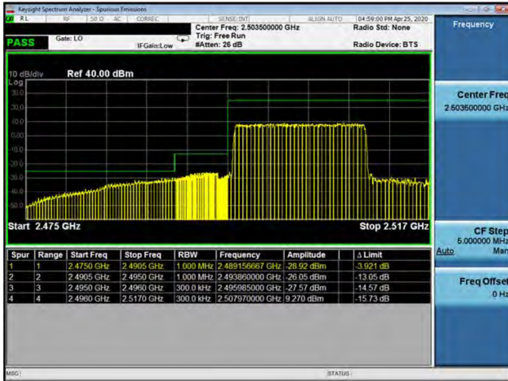
Plot 7-539. Lower ACP Plot at 2496 MHz (Band 41 (PC2) - 15.0MHz QPSK - Full RB Configuration)
