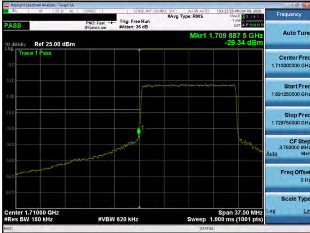
Plot 7-459. Lower Band Edge Plot (n66 - 15MHz DFT-s-OFDM-QPSK - Full RB Configuration)
