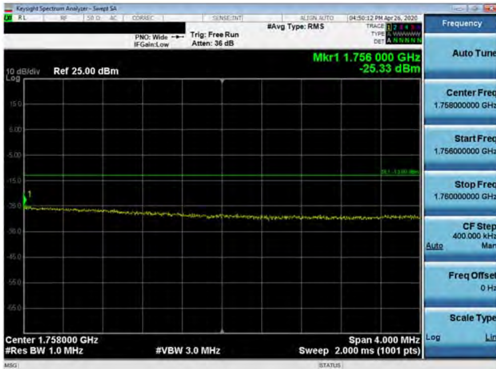
Plot 7-442. Upper Extended Band Edge Plot (Band 4 - 15.0MHz QPSK - Full RB Configuration)
