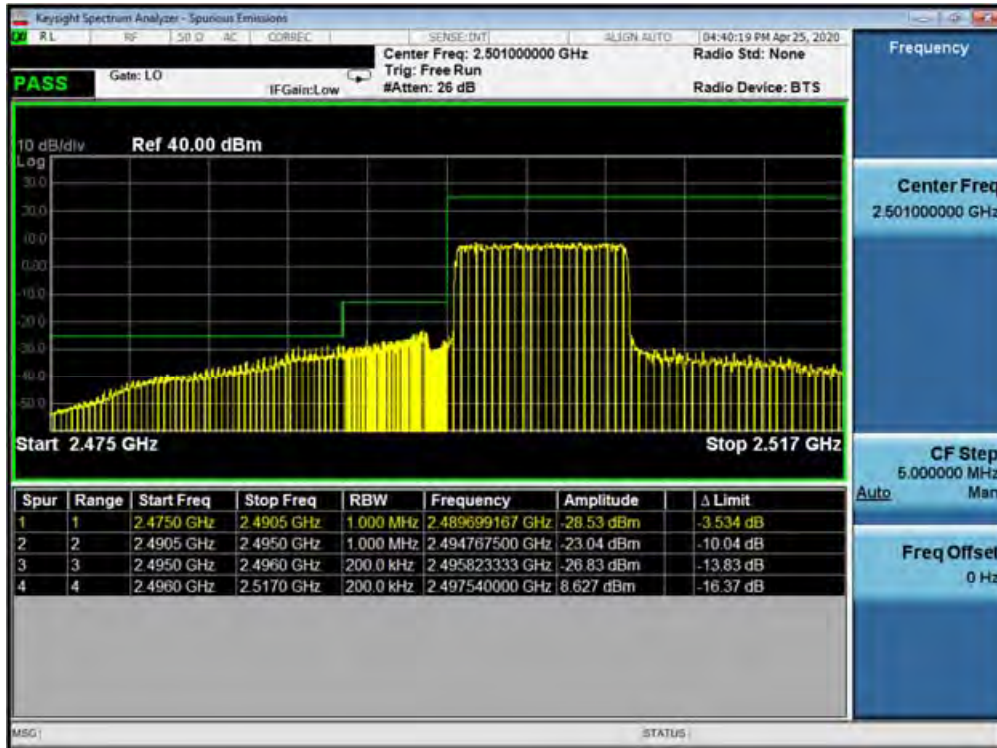
Plot 7-537. Lower ACP Plot at 2496 MHz (Band 41 (PC2) - 10.0MHz QPSK - Full RB Configuration)
