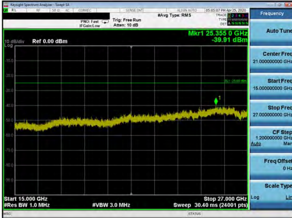
Plot 7-357. Conducted Spurious Plot (Band 41 (PC2) - 20.0MHz QPSK - RB Size 1, RB Offset 0 - High Channel)
