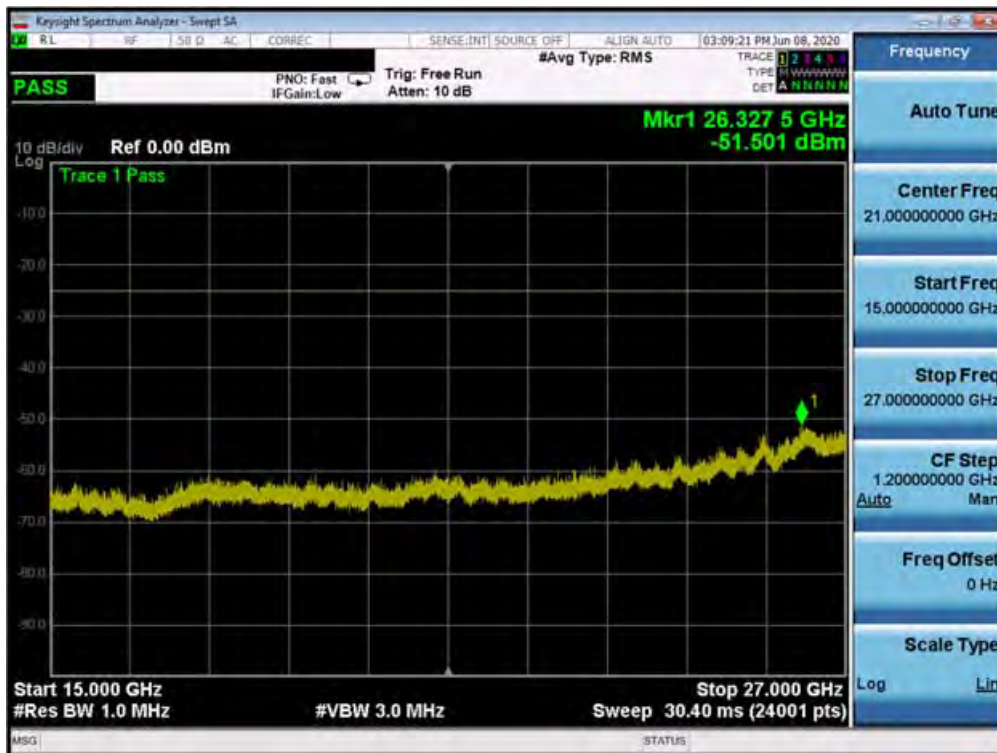
Plot 7-360. Conducted Spurious Plot (n41 - 100MHz DFT-s-OFDM-QPSK - RB Size 1, RB Offset 1 - Low Channel)
