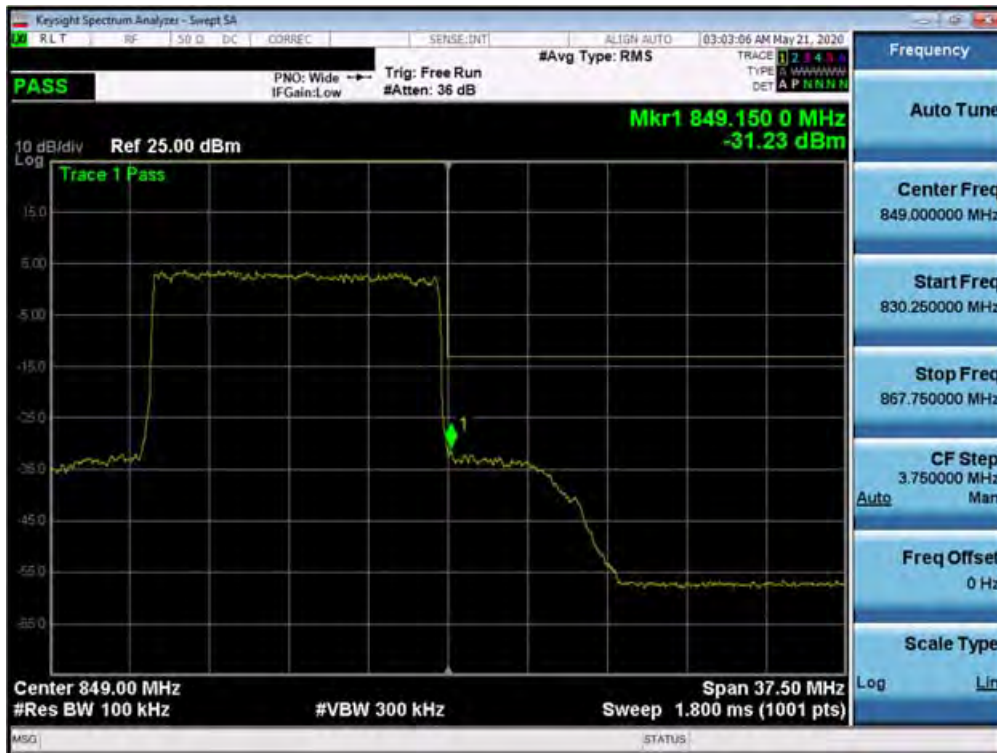
Plot 7-412. Upper Band Edge Plot (n5 – 15.0MHz DFT-s-OFDM BPSK - Full RB Configuration)
