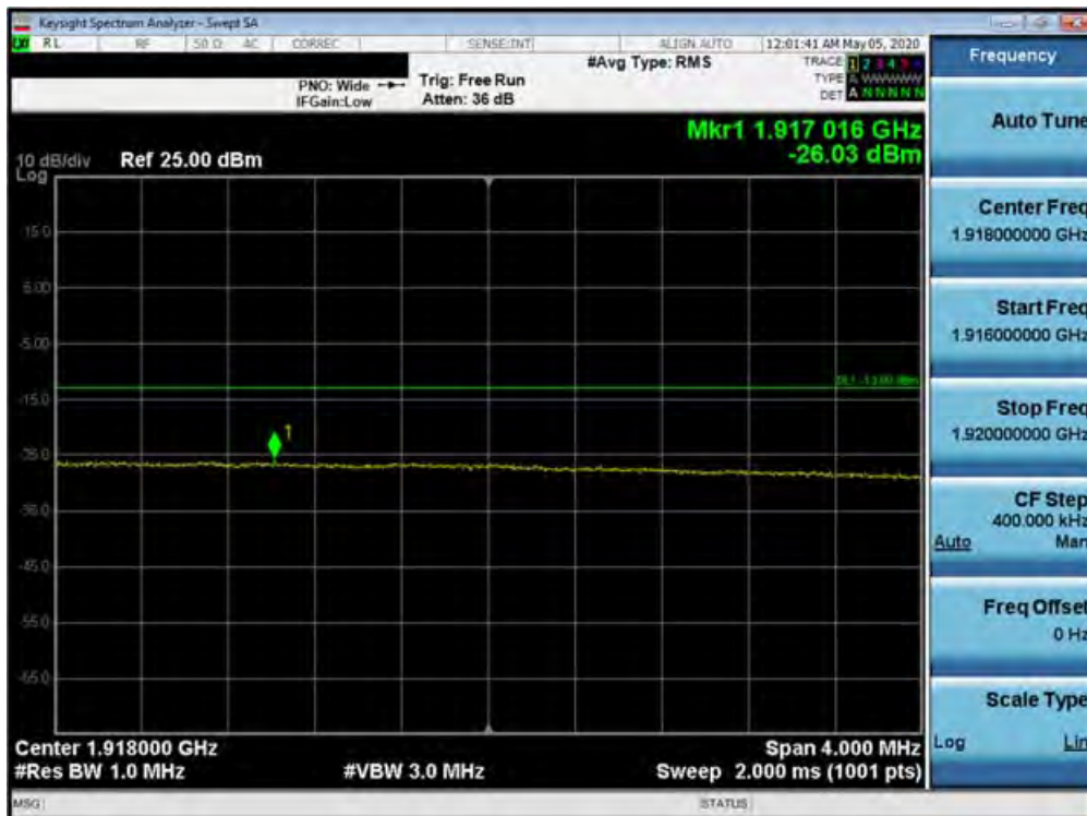
Plot 7-502. Upper Extended Band Edge Plot (Band 25 - 20.0MHz QPSK - Full RB Configuration)
