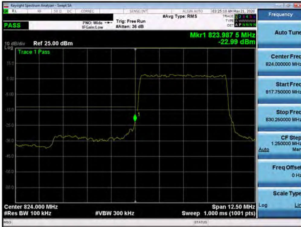
Plot 7-407. Lower Band Edge Plot (n5 – 5.0MHz DFT-s-OFDM BPSK - Full RB Configuration)
