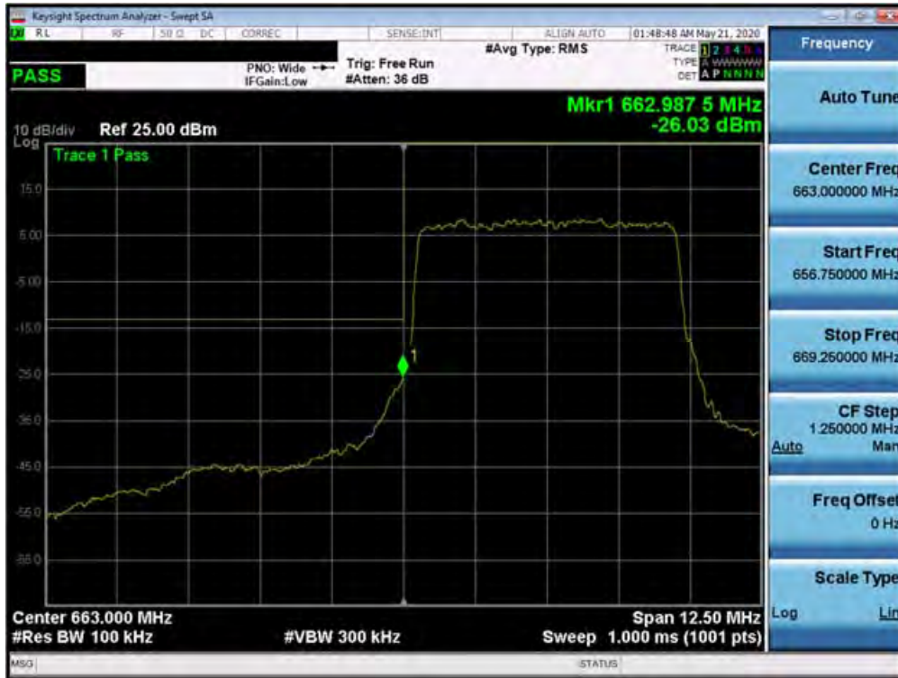
Plot 7-375. Lower Band Edge Plot (n71 - 5MHz DFT-s-OFDM-QPSK - Full RB Configuration)
