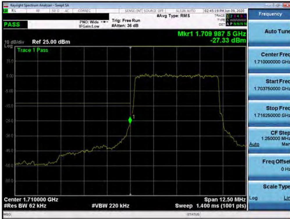
Plot 7-451. Lower Band Edge Plot (n66 - 5MHz DFT-s-OFDM-QPSK - Full RB Configuration)
