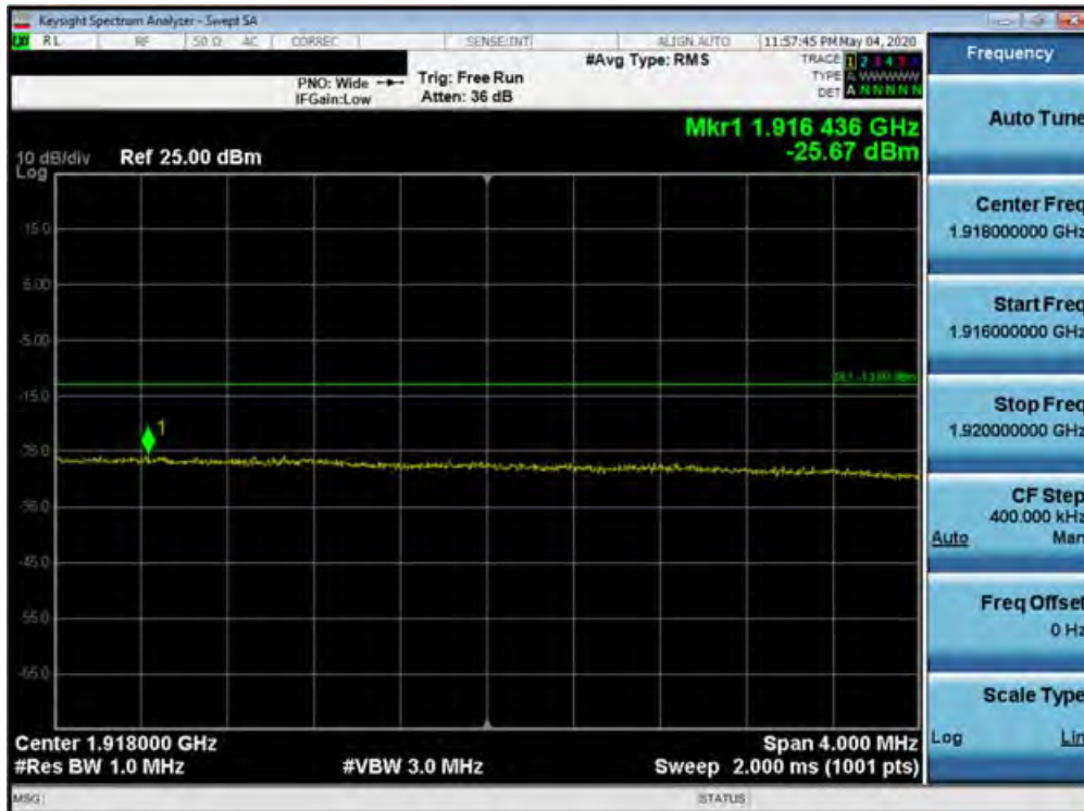
Plot 7-496. Upper Extended Band Edge Plot (Band 25 - 15.0MHz QPSK - Full RB Configuration)
