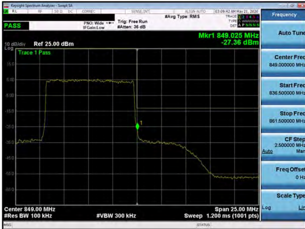
Plot 7-410. Upper Band Edge Plot (n5 – 10.0MHz DFT-s-OFDM BPSK - Full RB Configuration)
