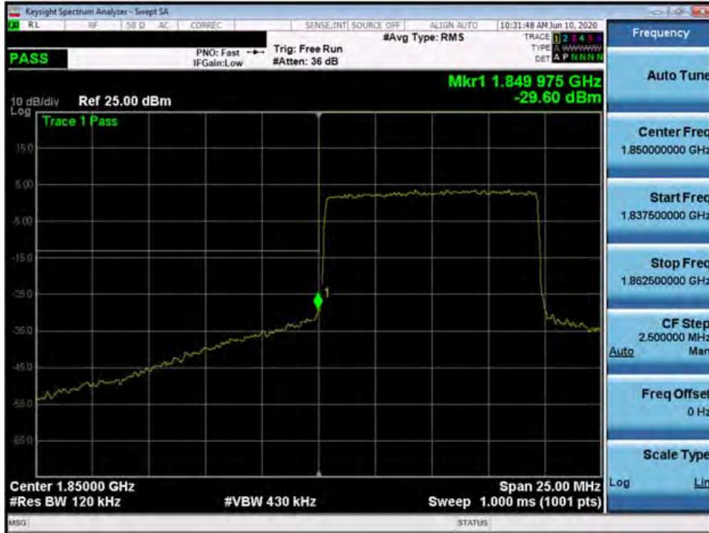
Plot 7-509. Lower Band Edge Plot (n25/2 - 10MHz DFT-s-OFDM-QPSK - Full RB Configuration)
