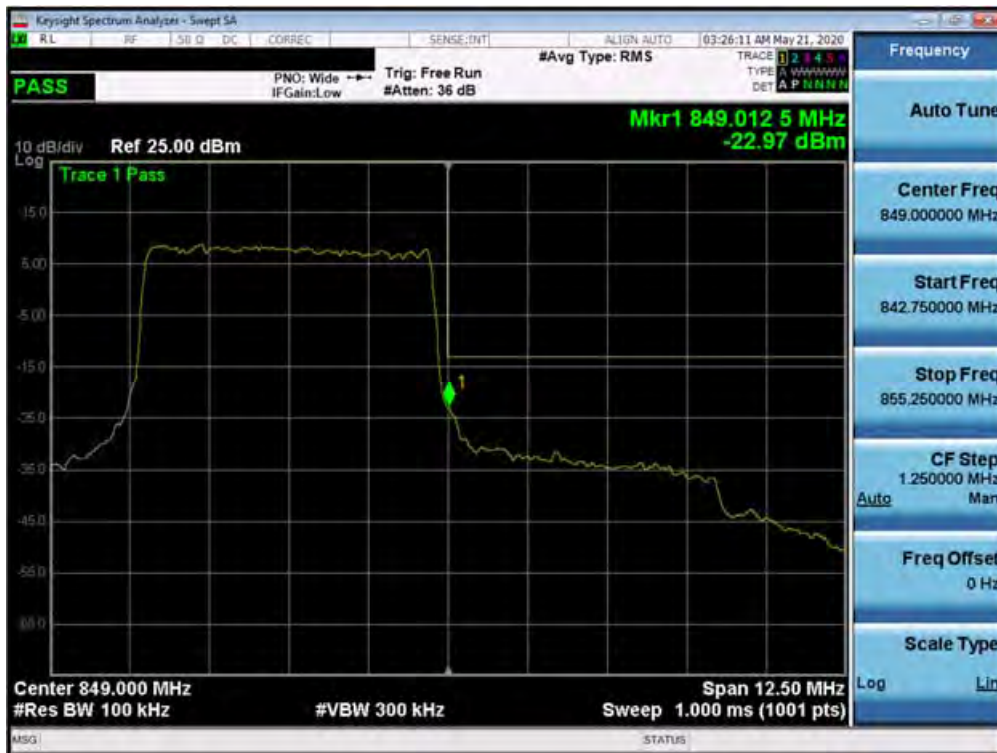
Plot 7-408. Upper Band Edge Plot (n5 – 5.0MHz DFT-s-OFDM BPSK - Full RB Configuration)
