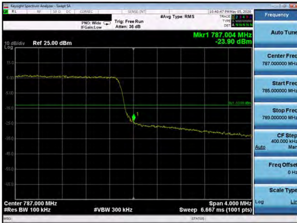
Plot 7-393. Upper Band Edge Plot (Band 13 - 5.0MHz QPSK - Full RB Configuration)
