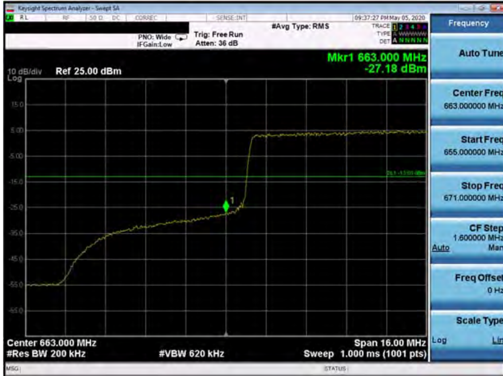
Plot 7-373. Lower Band Edge Plot (Band 71 - 20.0MHz QPSK - Full RB Configuration)
