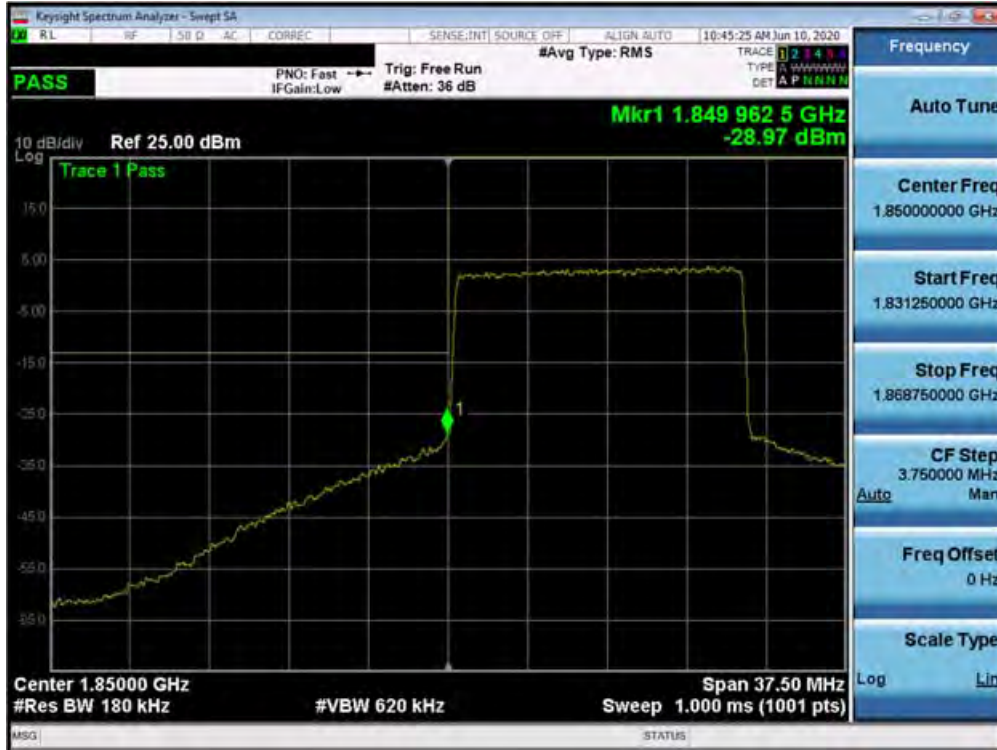
Plot 7-515. Lower Band Edge Plot (n25/2 - 15MHz DFT-s-OFDM-QPSK - Full RB Configuration)
