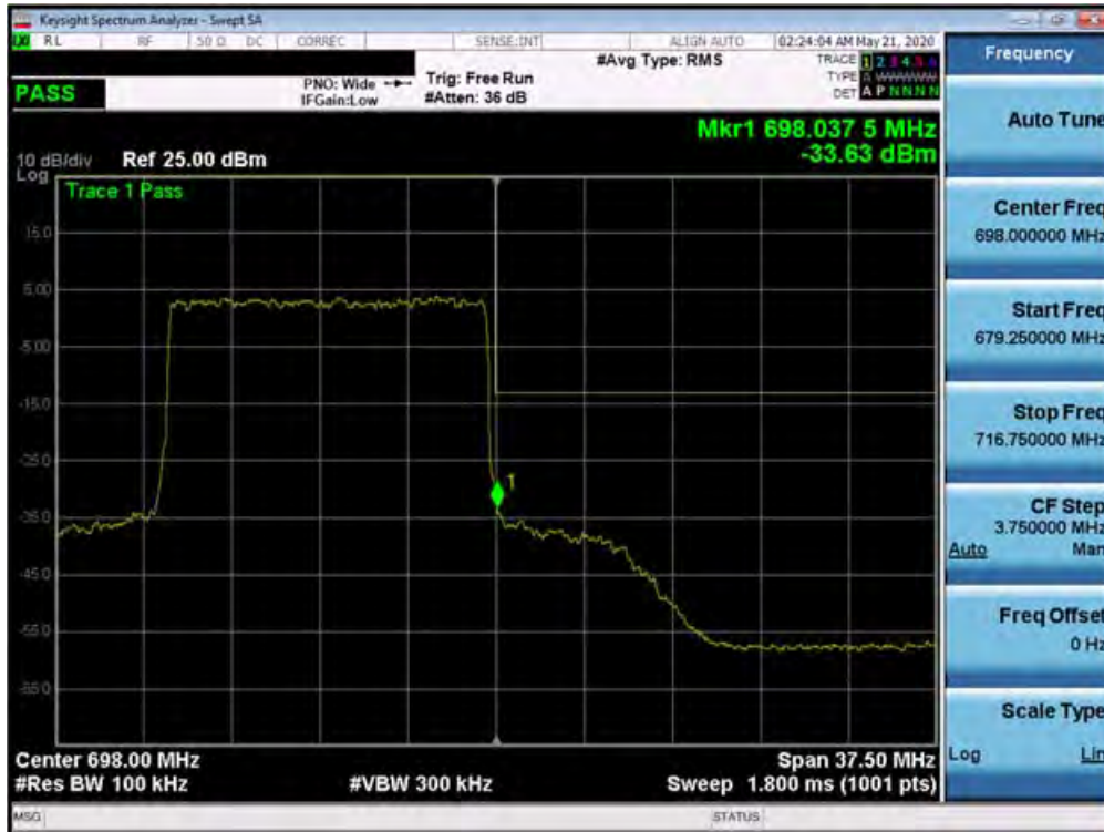
Plot 7-380. Upper Band Edge Plot (n71 - 15MHz DFT-s-OFDM-QPSK - Full RB Configuration)
