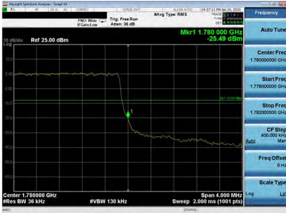
Plot 7-425. Upper Band Edge Plot (Band 66 - 3.0MHz QPSK - Full RB Configuration)
