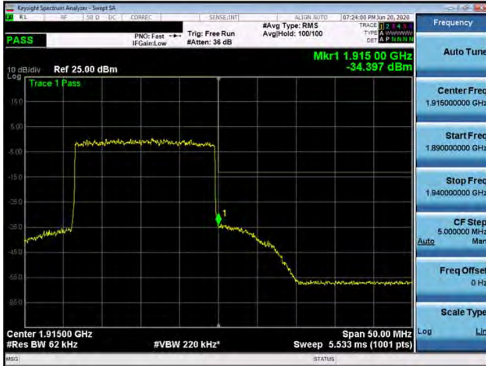
Plot 7-525. Upper Band Edge Plot (n25 - 20MHz DFT-s-OFDM-QPSK - Full RB Configuration)
