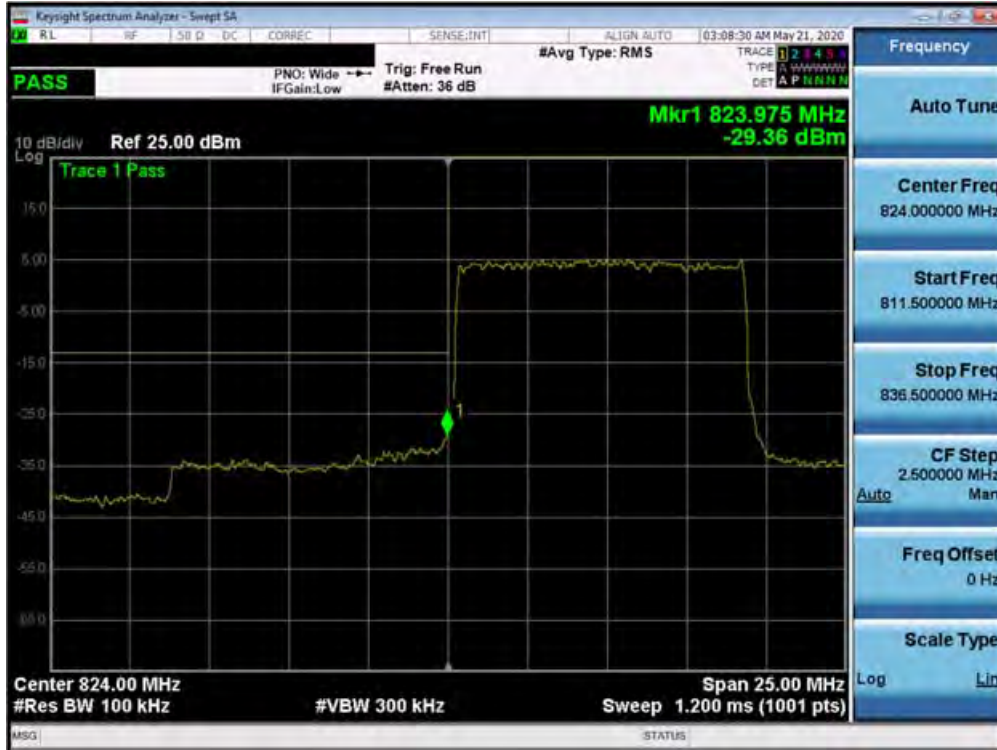
Plot 7-409. Lower Band Edge Plot (n5 – 10.0MHz DFT-s-OFDM BPSK - Full RB Configuration)
