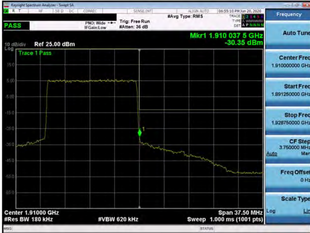
Plot 7-517. Upper Band Edge Plot (n2 - 15MHz DFT-s-OFDM-QPSK - Full RB Configuration)
