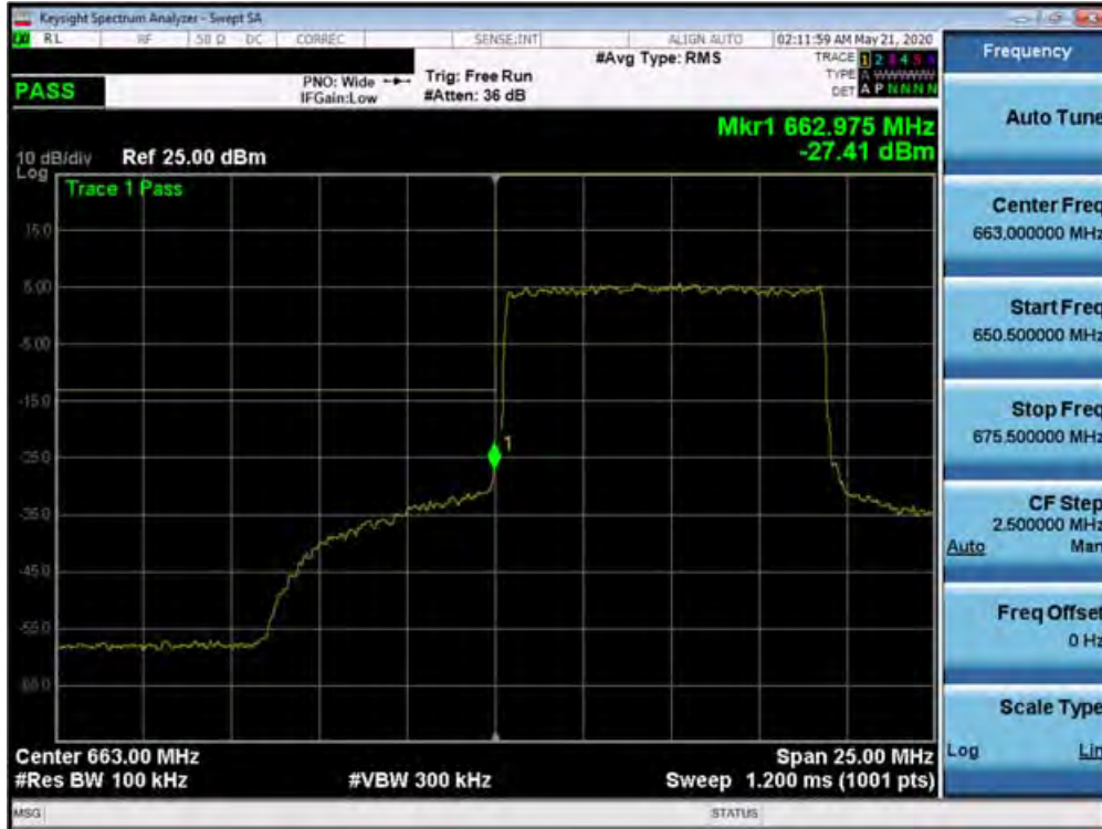
Plot 7-377. Lower Band Edge Plot (n71 - 10MHz DFT-s-OFDM-QPSK - Full RB Configuration)
