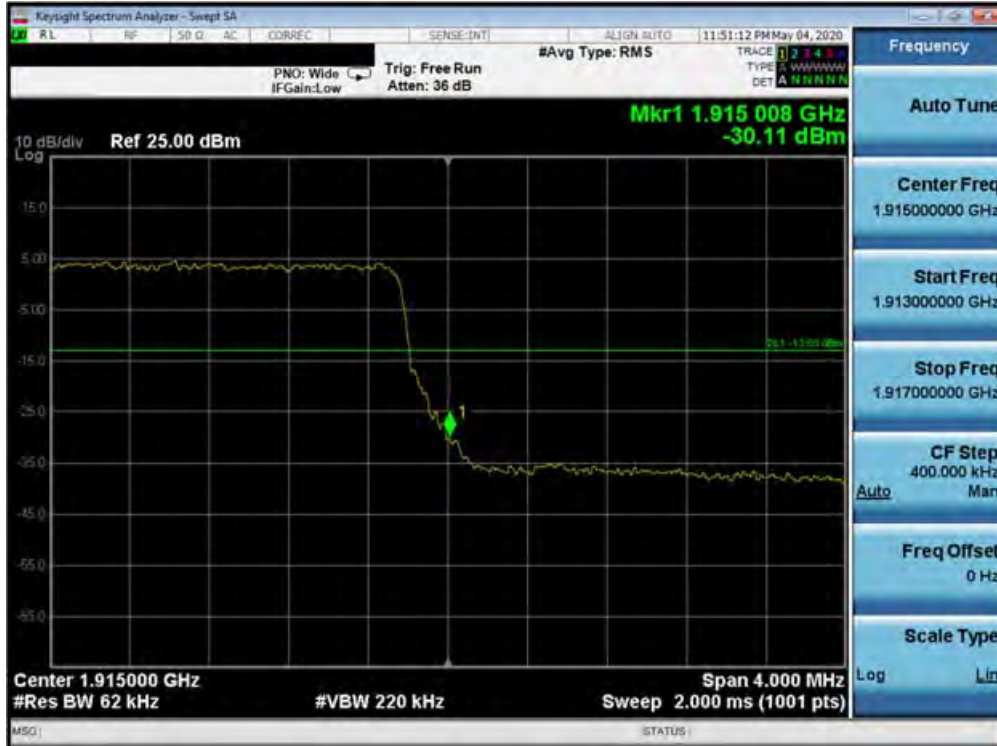
Plot 7-483. Upper Band Edge Plot (Band 25 - 5.0MHz QPSK - Full RB Configuration)
