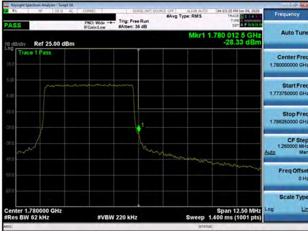
Plot 7-453. Upper Band Edge Plot (n66 - 5MHz DFT-s-OFDM-QPSK - Full RB Configuration)
