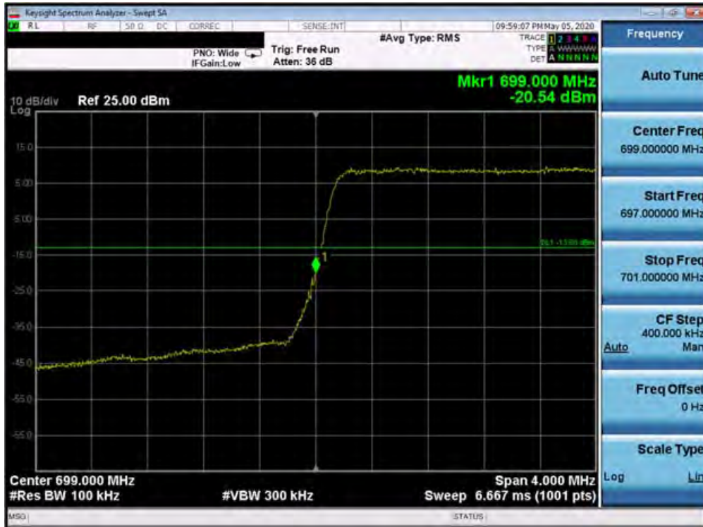
Plot 7-385. Lower Band Edge Plot (Band 12 - 3.0MHz QPSK - Full RB Configuration)
