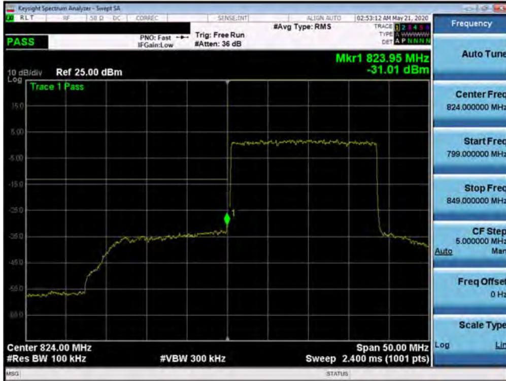
Plot 7-413. Lower Band Edge Plot (n5 – 20.0MHz DFT-s-OFDM BPSK - Full RB Configuration)
