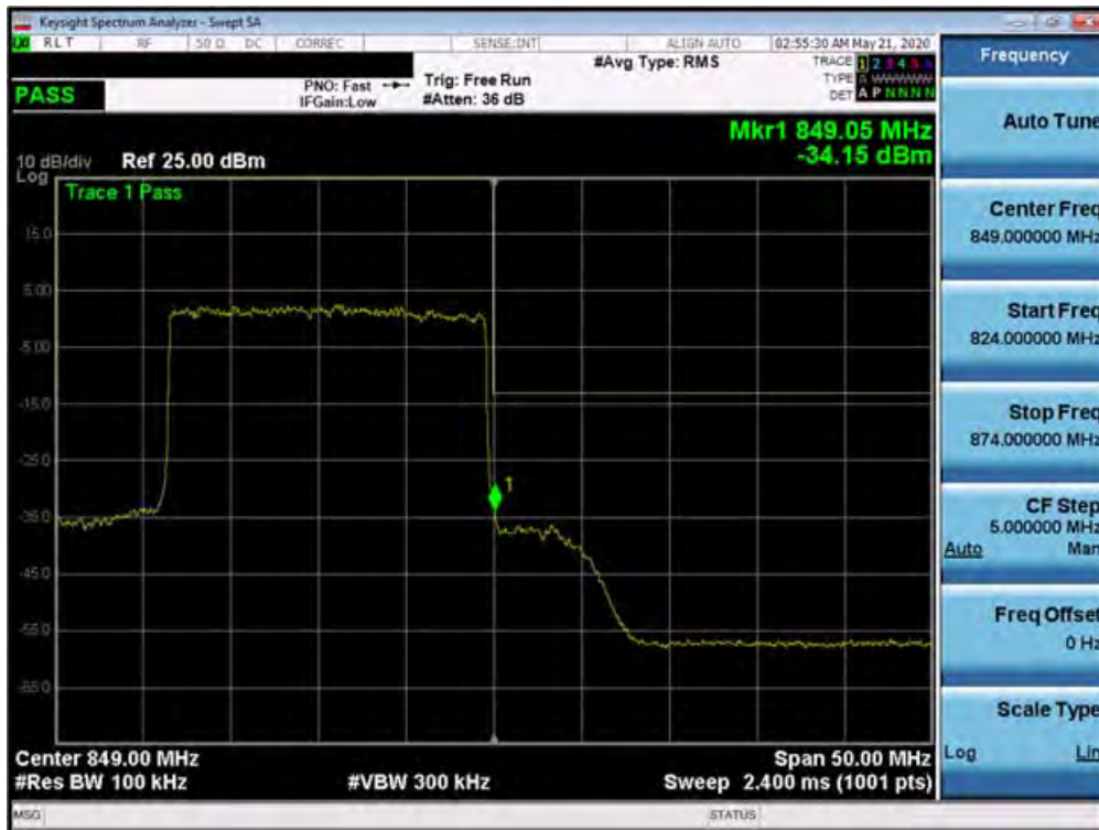
Plot 7-414. Upper Band Edge Plot (n5 – 20.0MHz DFT-s-OFDM BPSK - Full RB Configuration)
