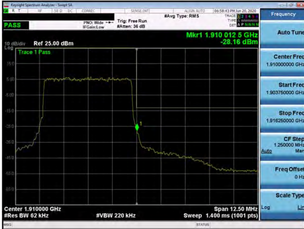
Plot 7-505. Upper Band Edge Plot (n2 - 5MHz DFT-s-OFDM-QPSK - Full RB Configuration)
