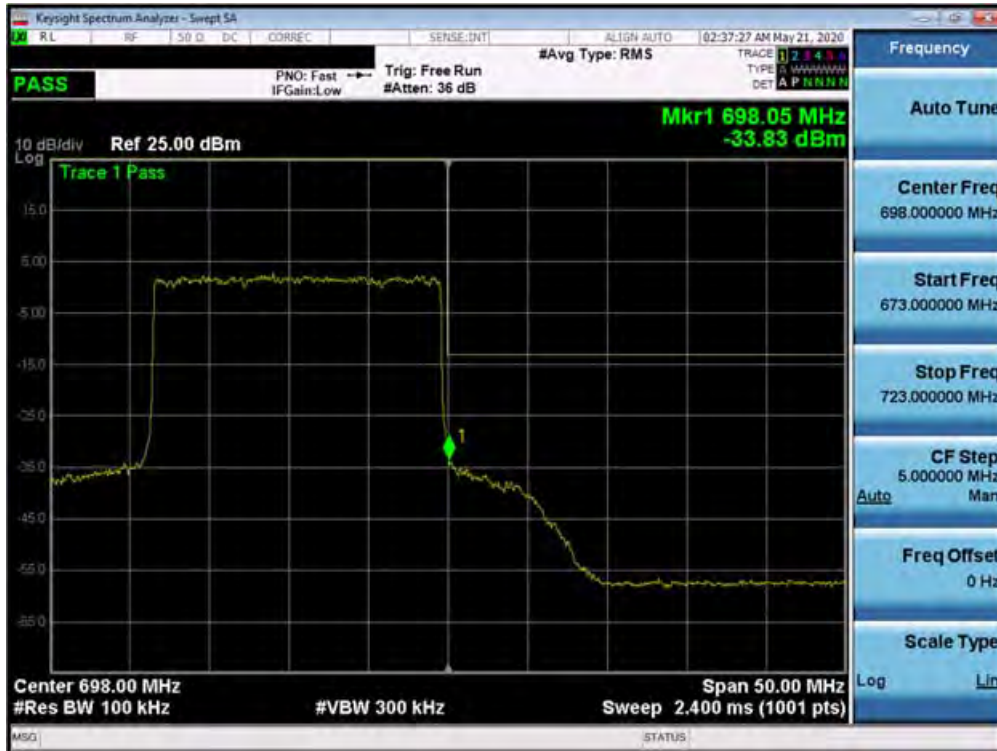
Plot 7-382. Upper Band Edge Plot (n71 - 20MHz DFT-s -OFDM-QPSK - Full RB Configuration)
