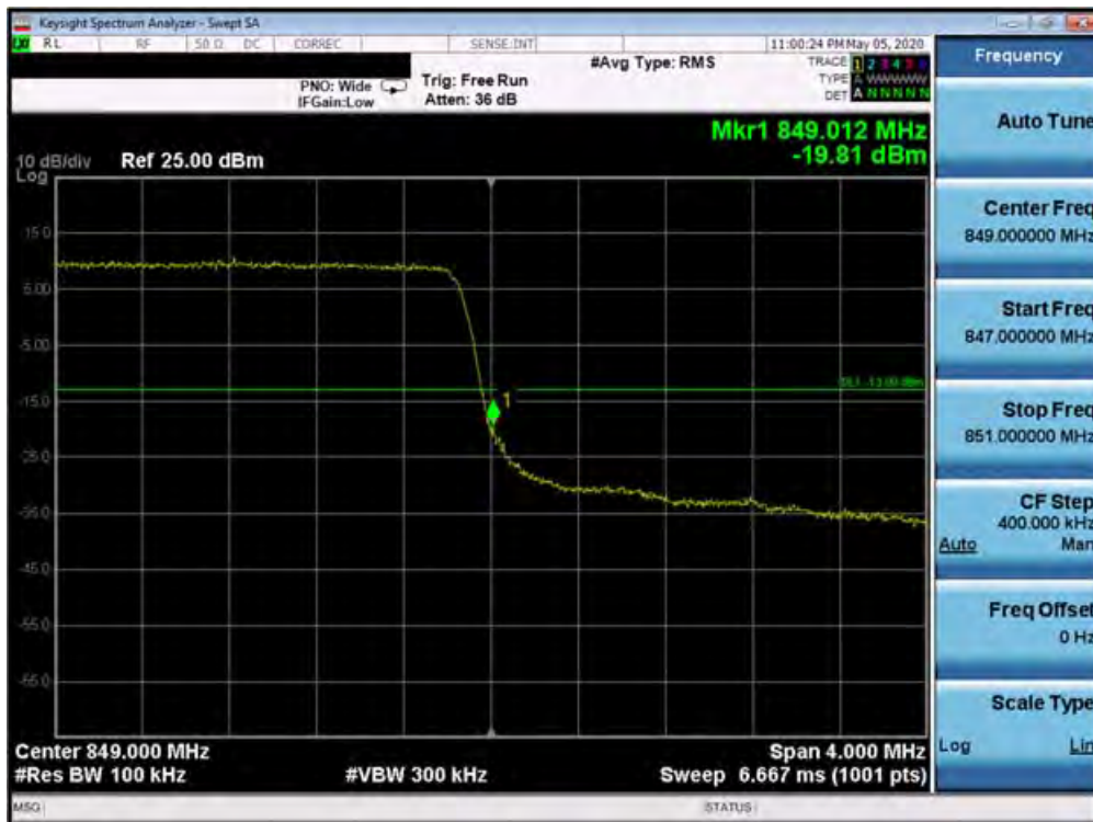
Plot 7-400. Upper Band Edge Plot (Band 26/5 - 3.0MHz QPSK - Full RB Configuration)
