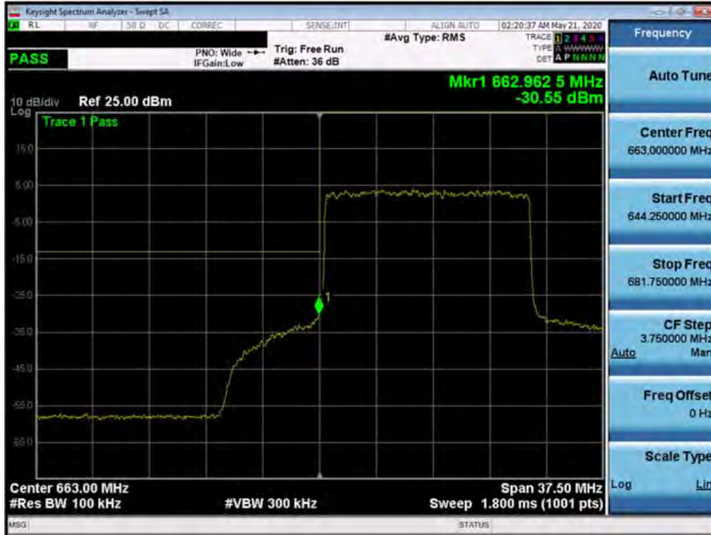
Plot 7-379. Lower Band Edge Plot (n71 - 15MHz DFT-s-OFDM-QPSK - Full RB Configuration)
