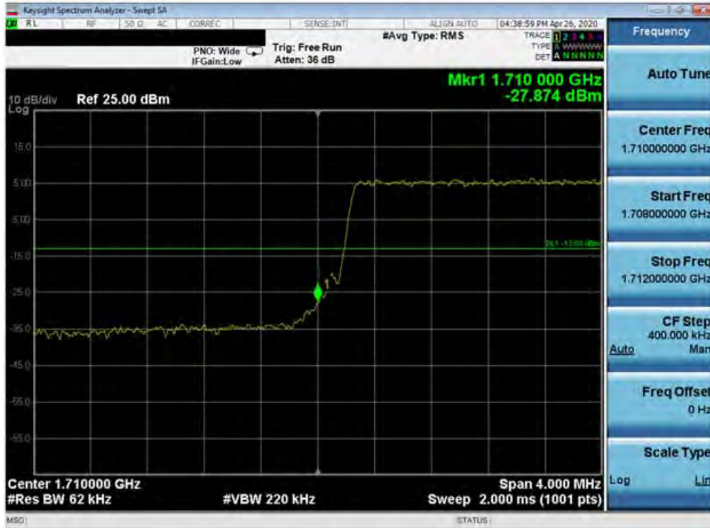
Plot 7-427. Lower Band Edge Plot (Band 66/4 - 5.0MHz QPSK - Full RB Configuration)
