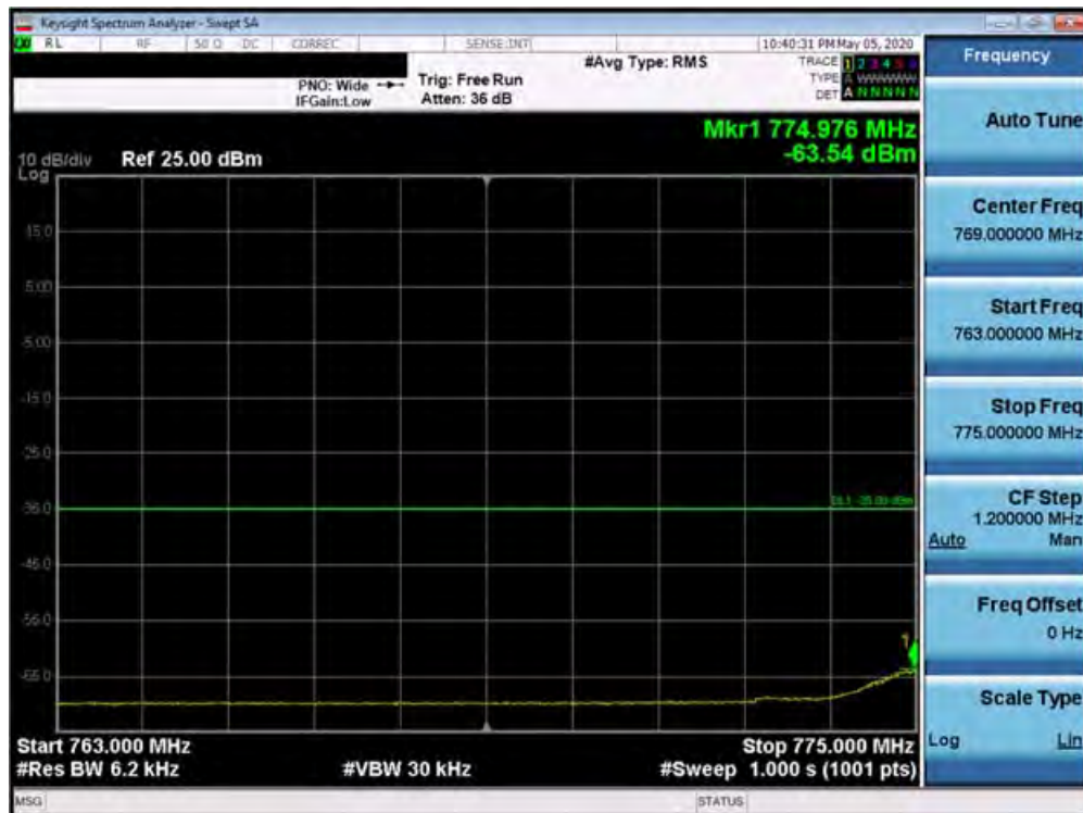
Plot 7-392. Lower Emission Mask Plot (Band 13 - 5.0MHz QPSK - Full RB Configuration)
