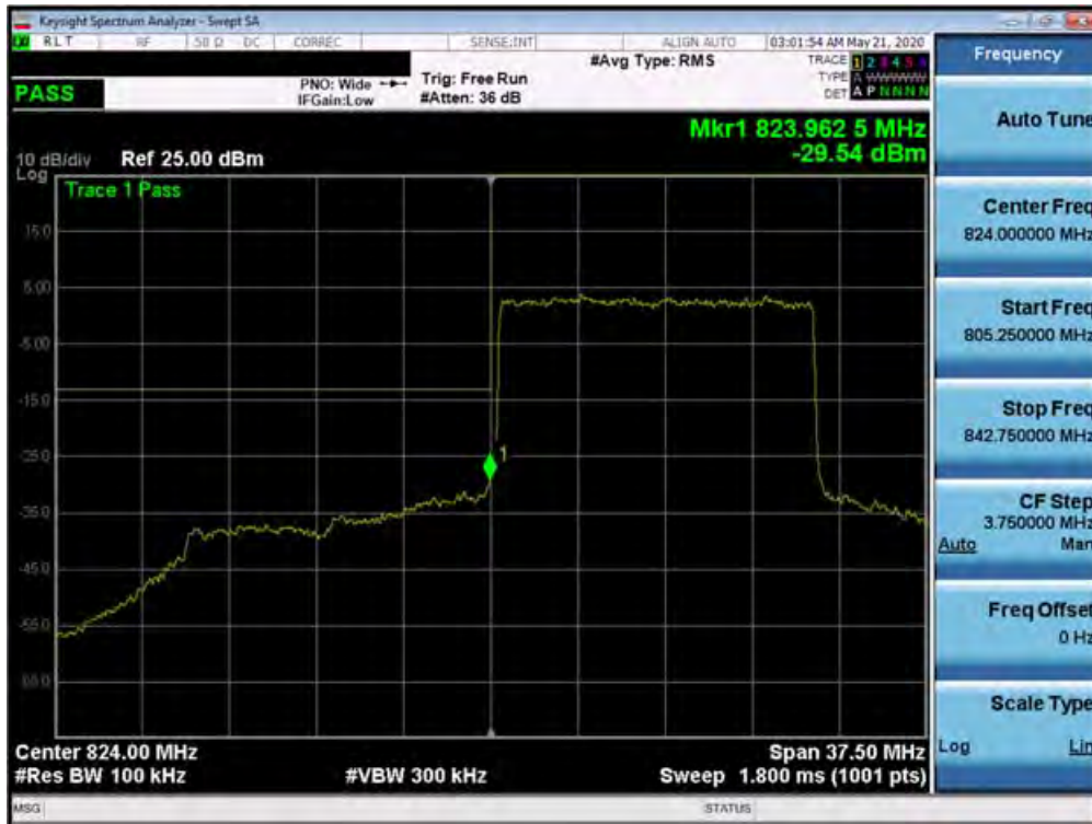
Plot 7-411. Lower Band Edge Plot (n5 – 15.0MHz DFT-s-OFDM BPSK - Full RB Configuration)
