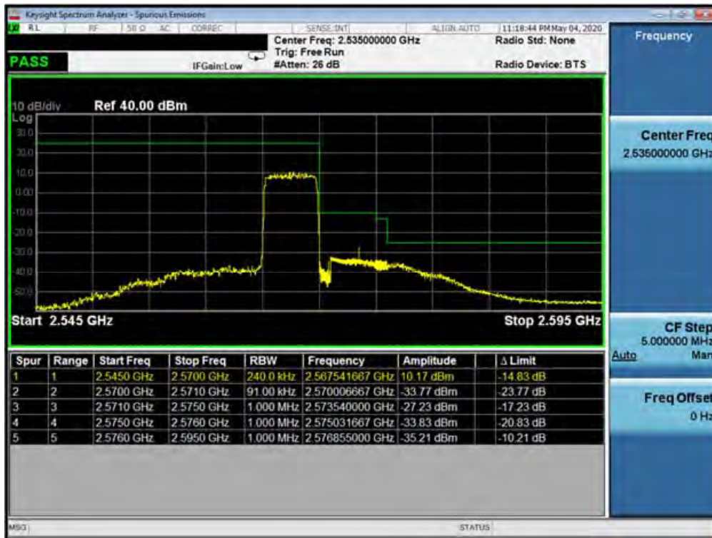
Plot 7-528. Higher ACP Plot (Band 7 - 5.0MHz QPSK - Full RB Configuration)
