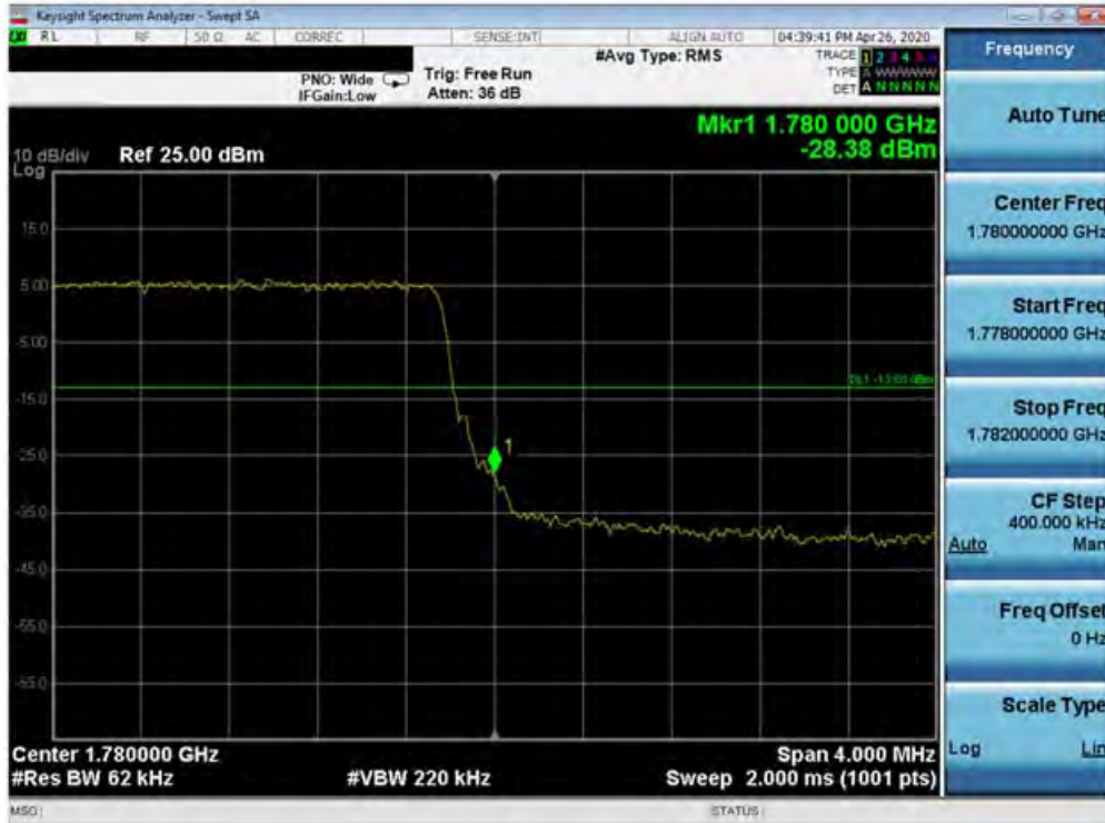
Plot 7-431. Upper Band Edge Plot (Band 66 - 5.0MHz QPSK - Full RB Configuration)
