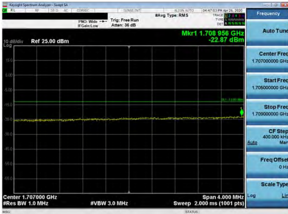
Plot 7-446. Lower Extended Band Edge Plot (Band 66/4 - 20.0MHz QPSK - Full RB Configuration)
