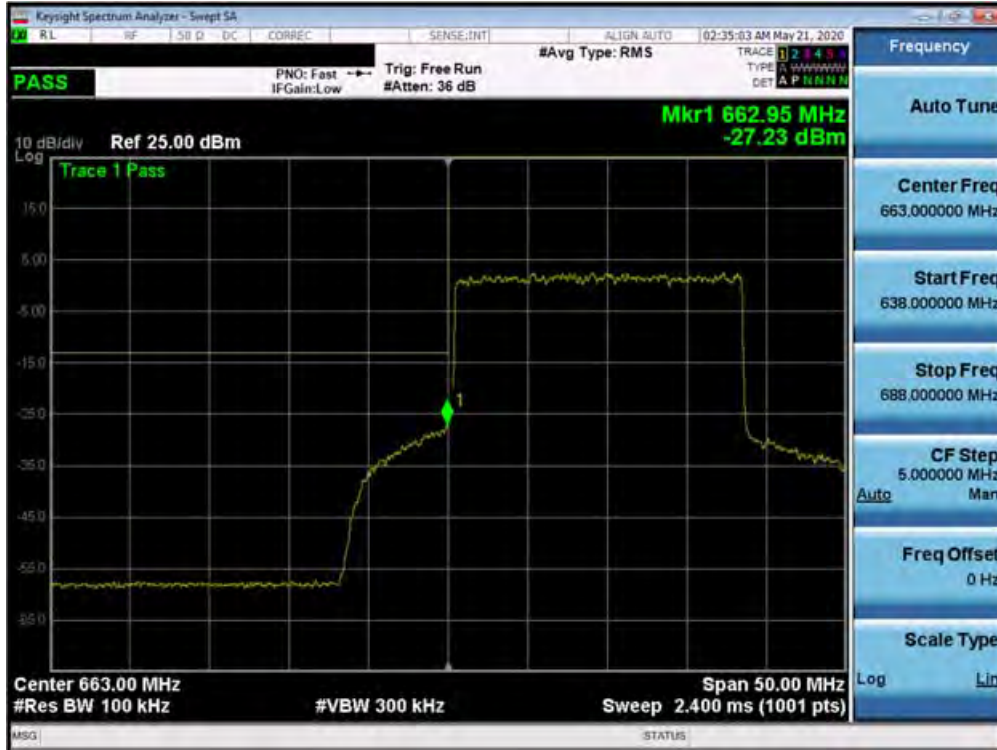
Plot 7-381. Lower Band Edge Plot (n71 - 20MHz DFT-s -OFDM-QPSK - Full RB Configuration)
