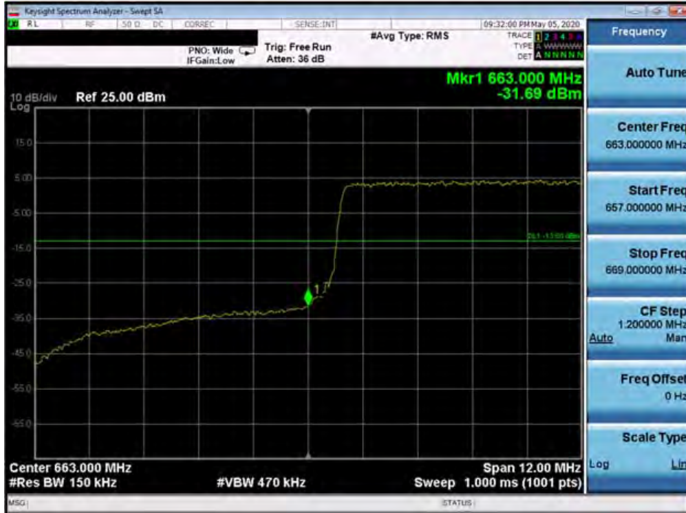
Plot 7-371. Lower Band Edge Plot (Band 71 - 15.0MHz QPSK - Full RB Configuration)
