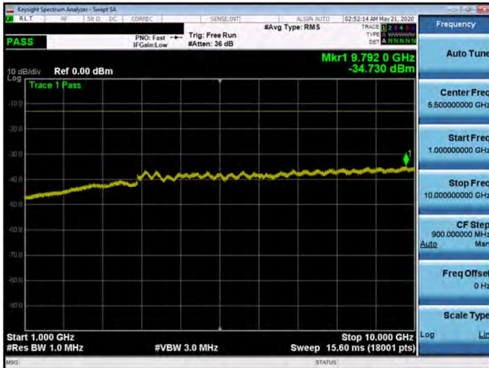
Plot 7-300. Conducted Spurious Plot (n5 - 20.0MHz DFT-s-OFDM BPSK - RB Size 1, RB Offset 0 - Mid Channel)
