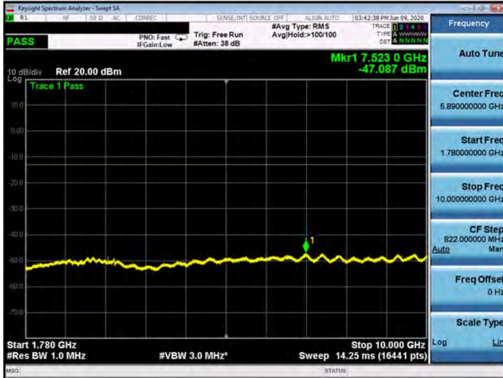
Plot 7-317. Conducted Spurious Plot (n66 - 20MHz DFT-s-OFDM-QPSK - RB Size 1, RB Offset 1 - Mid Channel)
