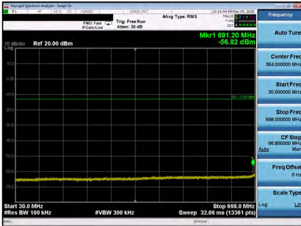
Plot 7-280. Conducted Spurious Plot (Band 12 - 10.0MHz QPSK - RB Size 1, RB Offset 0 - High Channel)
