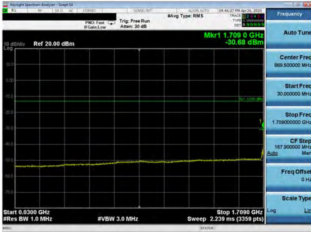
Plot 7-304. Conducted Spurious Plot (Band 66/4 - 20.0MHz QPSK - RB Size 1, RB Offset 0 - Low Channel)
