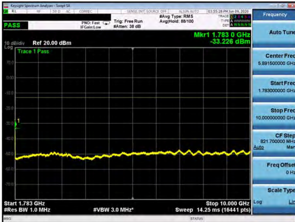
Plot 7-320. Conducted Spurious Plot (n66 - 20MHz DFT-s-OFDM-QPSK - RB Size 1, RB Offset 1 - High Channel)
