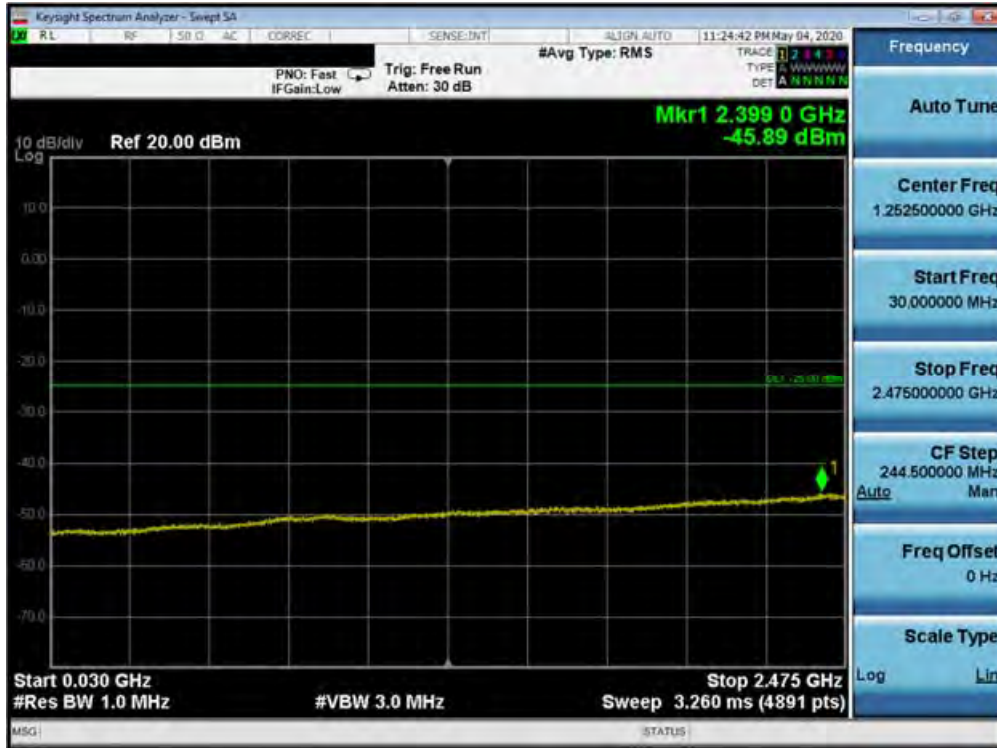
Plot 7-340. Conducted Spurious Plot (Band 7 - 20.0MHz QPSK - RB Size 1, RB Offset 0 - Low Channel)
