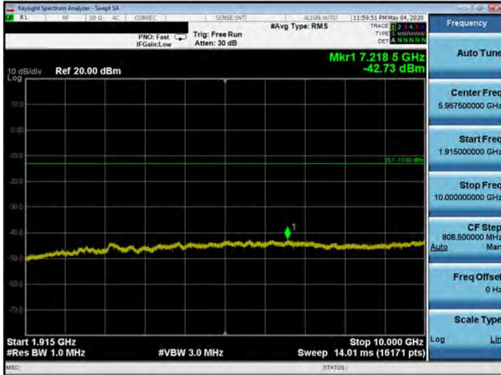
Plot 7-326. Conducted Spurious Plot (Band 25/2 - 20.0MHz QPSK - RB Size 1, RB Offset 0 - Mid Channel)
