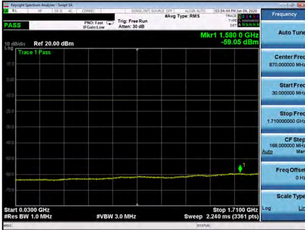
Plot 7-319. Conducted Spurious Plot (n66 - 20MHz DFT-s-OFDM-QPSK - RB Size 1, RB Offset 1 - High Channel)
