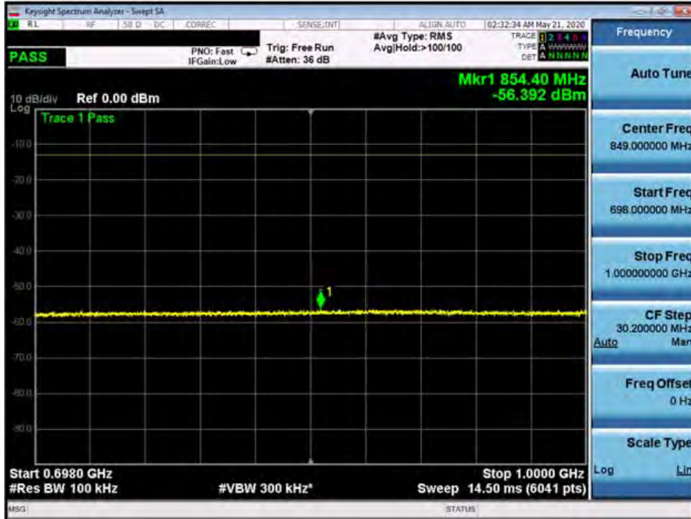
Plot 7-269. Conducted Spurious Plot (n71 - 20MHz DFT-s-OFDM-QPSK - RB Size 1, RB Offset 1 - Mid Channel)
