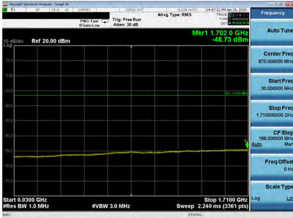
Plot 7-310. Conducted Spurious Plot (Band 66/4 - 20.0MHz QPSK - RB Size 1, RB Offset 0 - High Channel)
