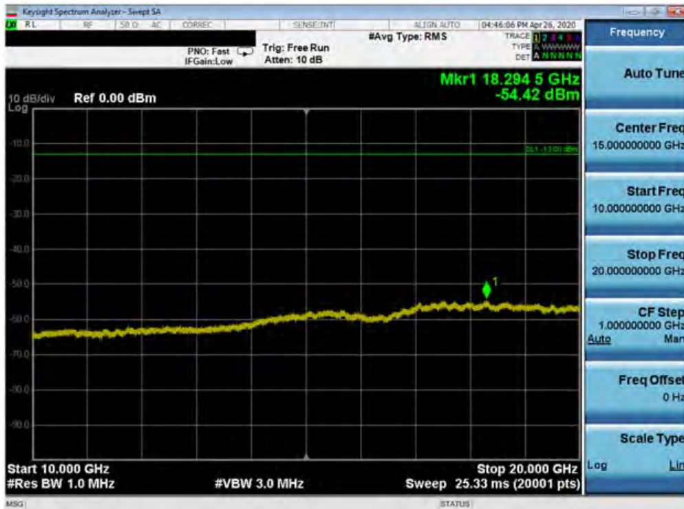
Plot 7-309. Conducted Spurious Plot (Band 66/4 - 20.0MHz QPSK - RB Size 1, RB Offset 0 - Mid Channel)
