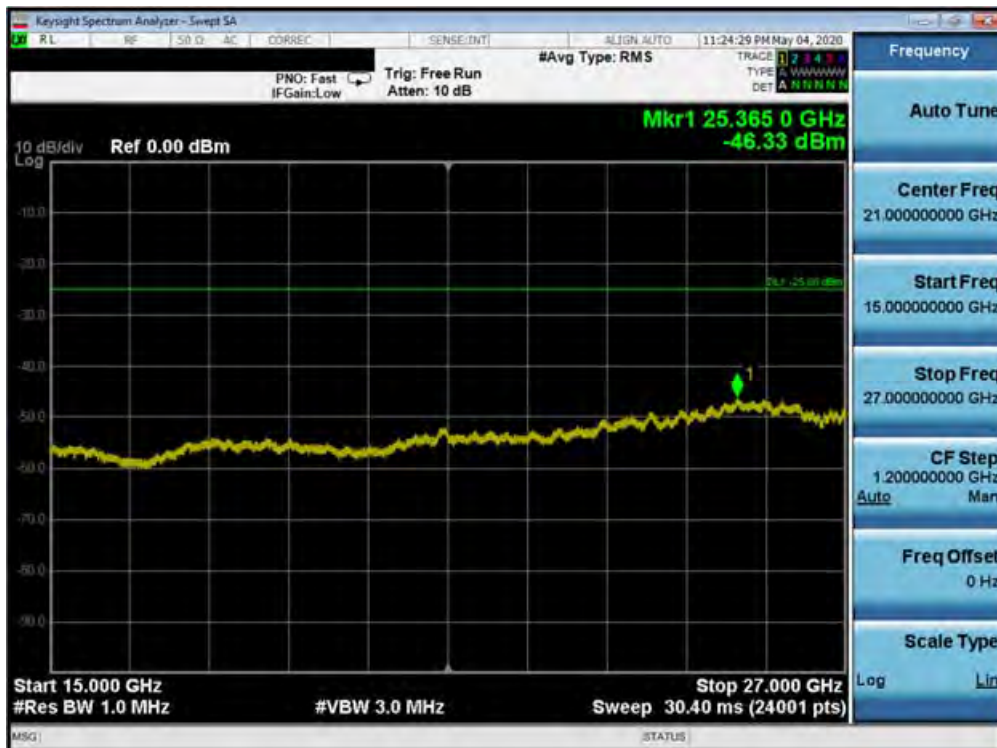
Plot 7-345. Conducted Spurious Plot (Band 7 - 20.0MHz QPSK - RB Size 1, RB Offset 0 - Mid Channel)
