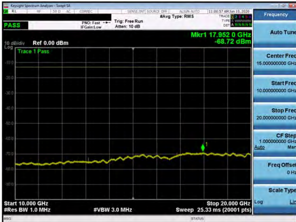
Plot 7-336. Conducted Spurious Plot (n25/2 - 20MHz DFT-s-OFDM-QPSK - RB Size 1, RB Offset 1 - Mid Channel)
