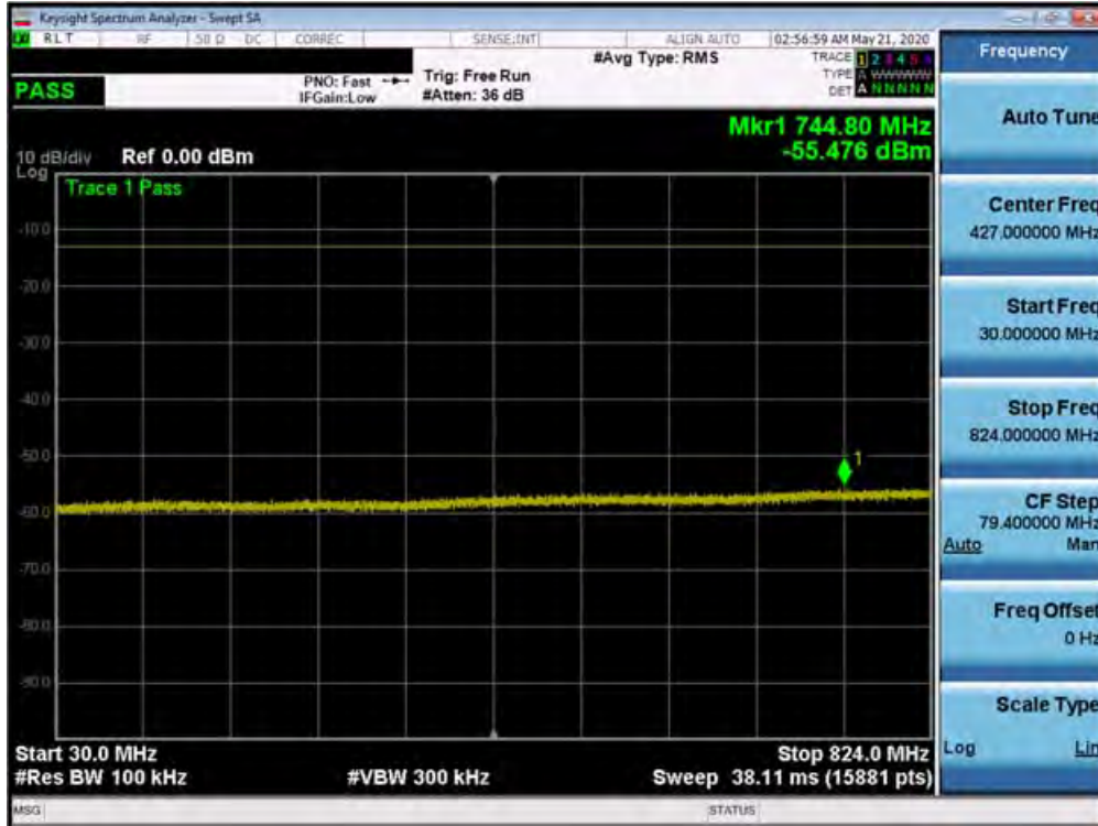
Plot 7-301. Conducted Spurious Plot (n5 - 20.0MHz DFT-s-OFDM BPSK - RB Size 1, RB Offset 0 - High Channel)
