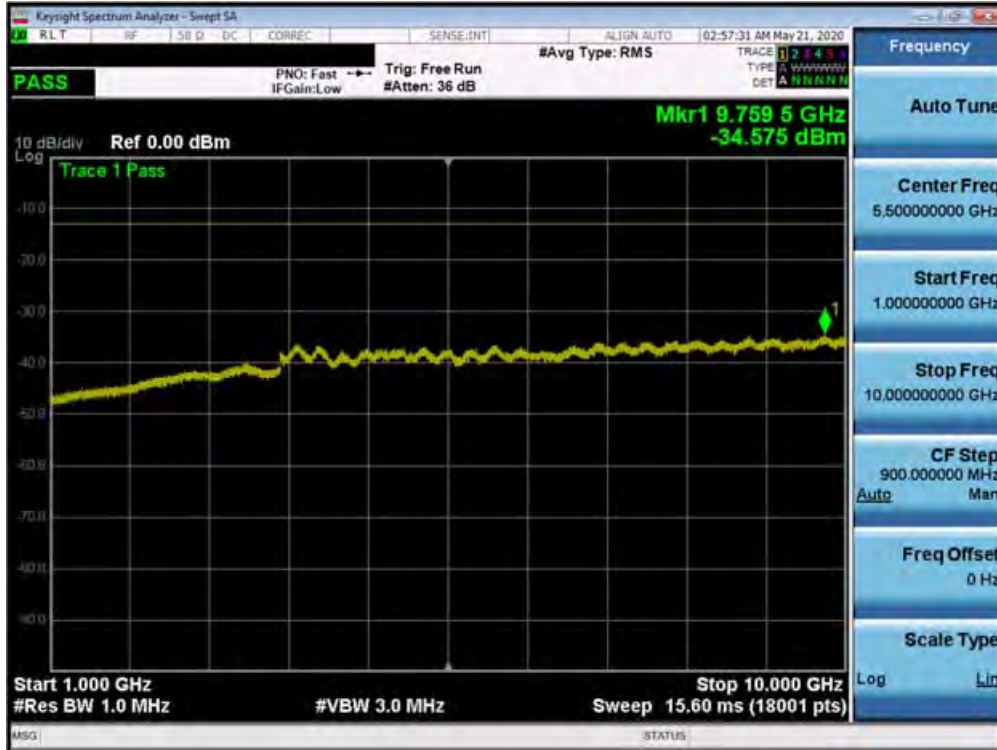
Plot 7-303. Conducted Spurious Plot (n5 - 20.0MHz DFT-s-OFDM BPSK - RB Size 1, RB Offset 0 - High Channel)
