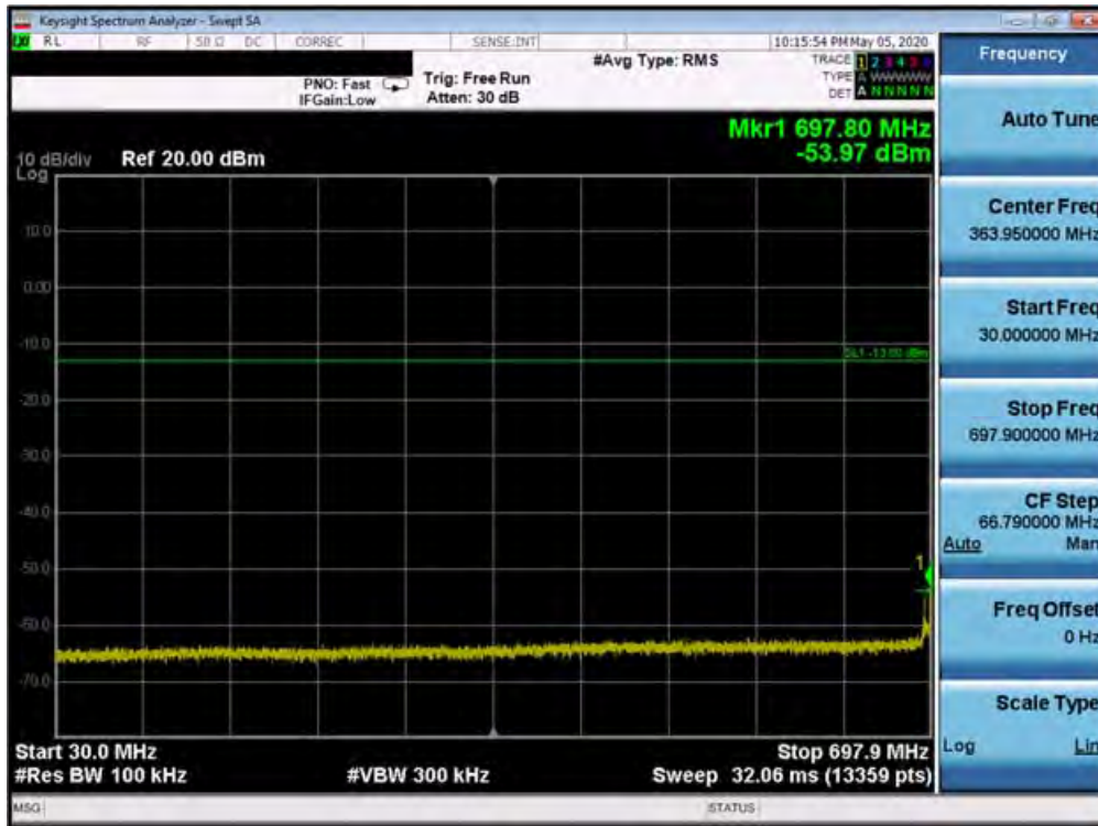
Plot 7-274. Conducted Spurious Plot (Band 12 - 10.0MHz QPSK - RB Size 1, RB Offset 0 - Low Channel)
