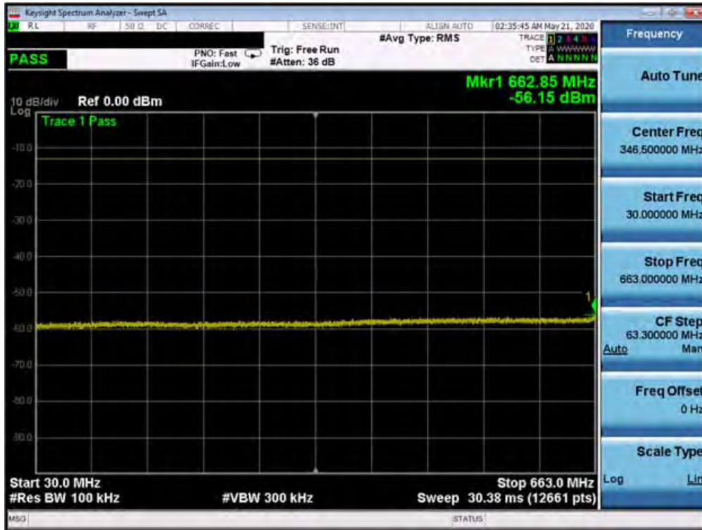
Plot 7-265. Conducted Spurious Plot (n71 - 20MHz DFT-s-OFDM-QPSK - RB Size 1, RB Offset 1 - Low Channel)
