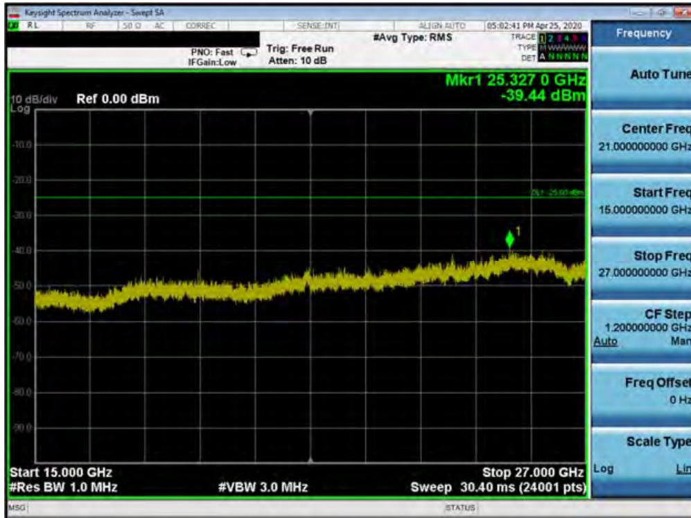
Plot 7-351. Conducted Spurious Plot (Band 41 (PC2) - 20.0MHz QPSK - RB Size 1, RB Offset 0 - Low Channel)
