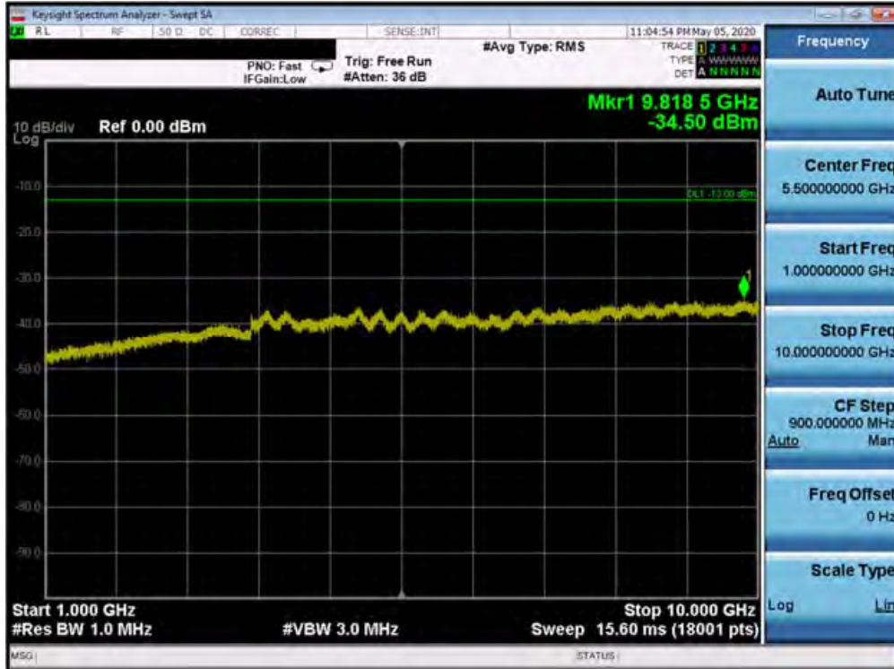
Plot 7-294. Conducted Spurious Plot (Band 26/5 - 10.0MHz QPSK - RB Size 1, RB Offset 0 - High Channel)
