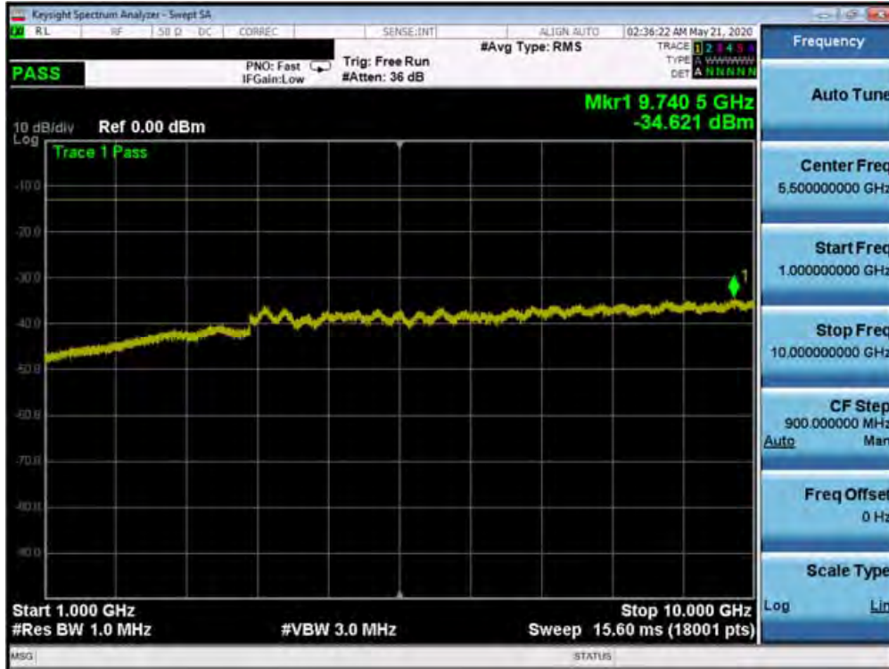
Plot 7-267. Conducted Spurious Plot (n71 - 20MHz DFT-s-OFDM-QPSK - RB Size 1, RB Offset 1 - Low Channel)
