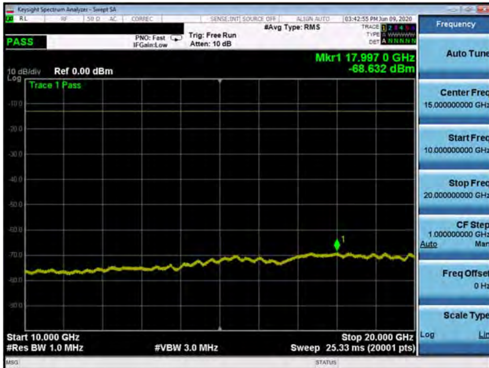
Plot 7-318. Conducted Spurious Plot (n66 - 20MHz DFT-s-OFDM-QPSK - RB Size 1, RB Offset 1 - Mid Channel)
