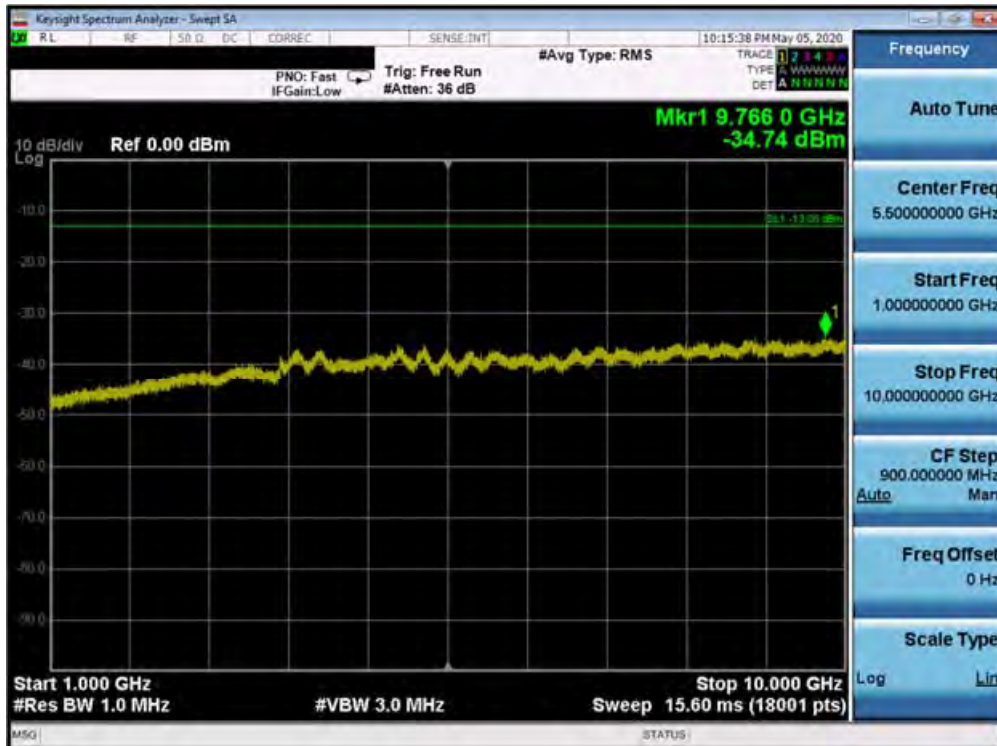
Plot 7-279. Conducted Spurious Plot (Band 12 - 10.0MHz QPSK - RB Size 1, RB Offset 0 - Mid Channel)
