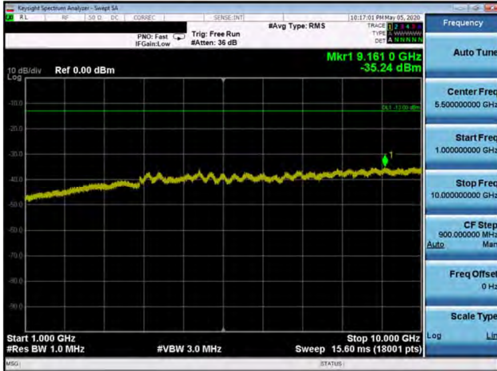
Plot 7-282. Conducted Spurious Plot (Band 12 - 10.0MHz QPSK - RB Size 1, RB Offset 0 - High Channel)
