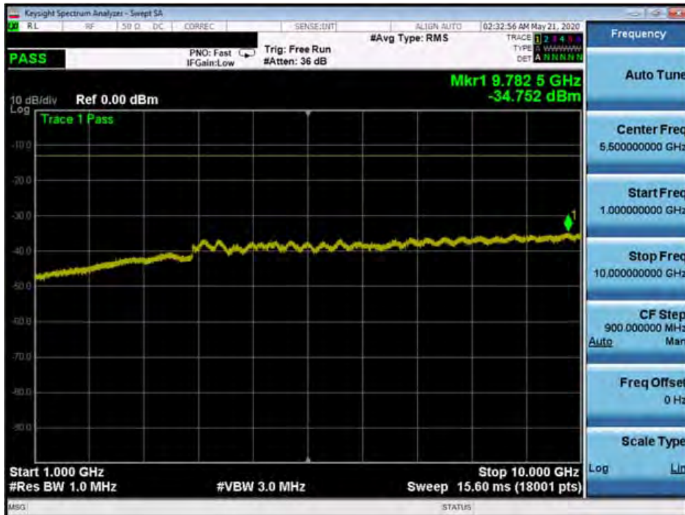
Plot 7-270. Conducted Spurious Plot (n71 - 20MHz DFT-s-OFDM-QPSK - RB Size 1, RB Offset 1 - Mid Channel)
