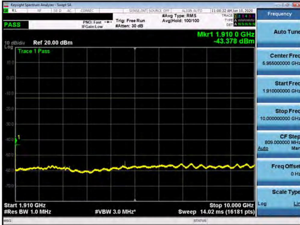
Plot 7-335. Conducted Spurious Plot (n25/2 - 20MHz DFT-s-OFDM-QPSK - RB Size 1, RB Offset 1 - Mid Channel)
