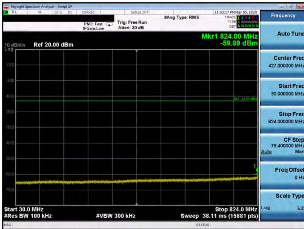
Plot 7-289. Conducted Spurious Plot (Band 26/5 - 10.0MHz QPSK - RB Size 1, RB Offset 0 - Mid Channel)
