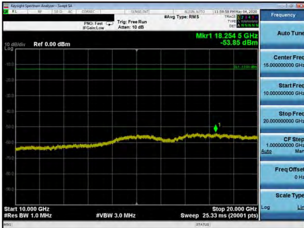
Plot 7-327. Conducted Spurious Plot (Band 25/2 - 20.0MHz QPSK - RB Size 1, RB Offset 0 - Mid Channel)
