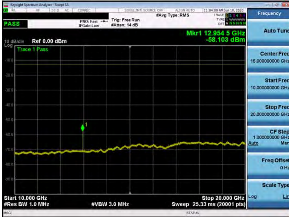
Plot 7-333. Conducted Spurious Plot (n25/2 - 20MHz DFT-s-OFDM-QPSK - RB Size 1, RB Offset 1 - Low Channel)
