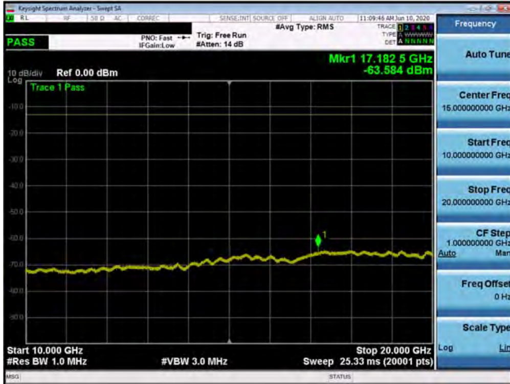
Plot 7-339. Conducted Spurious Plot (n25/2 - 20MHz DFT-s-OFDM-QPSK - RB Size 1, RB Offset 1 - High Channel)
