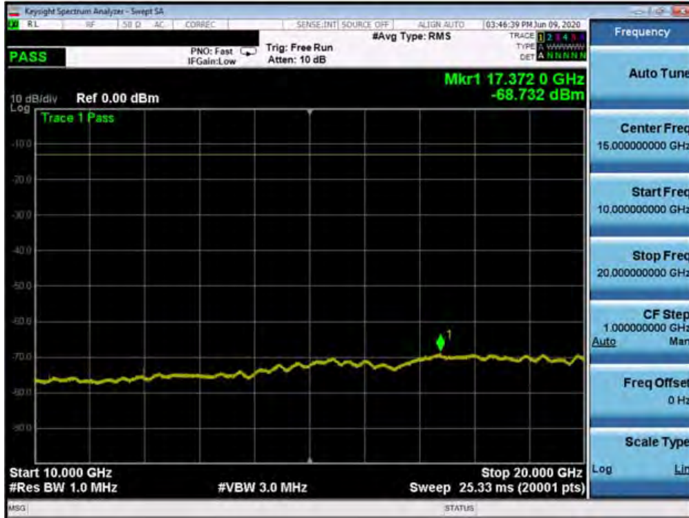
Plot 7-315. Conducted Spurious Plot (n66 - 20MHz DFT-s-OFDM-QPSK - RB Size 1, RB Offset 1 - Low Channel)
