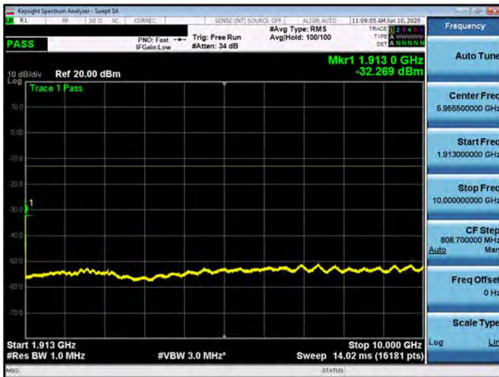
Plot 7-338. Conducted Spurious Plot (n25/2 - 20MHz DFT-s-OFDM-QPSK - RB Size 1, RB Offset 1 - High Channel)
