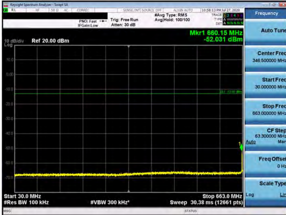
Plot 7-271. Conducted Spurious Plot (n71 - 20MHz DFT-s-OFDM-QPSK - RB Size 1, RB Offset 1 - High Channel)
