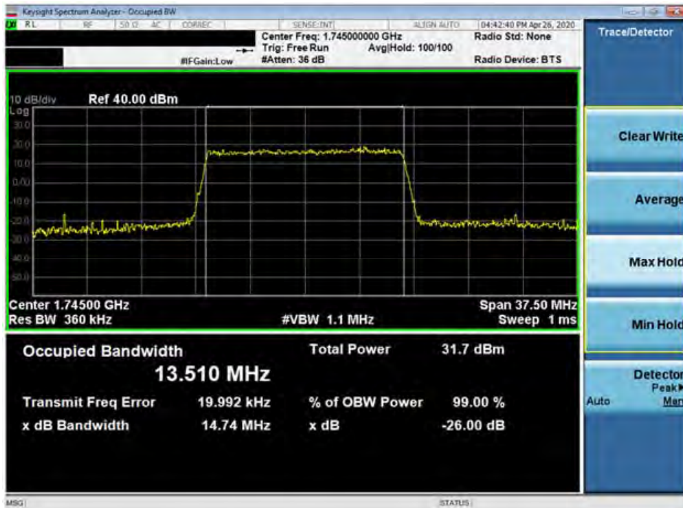
Plot 7-118. Occupied Bandwidth Plot (Band 66/4 - 15.0MHz 16-QAM - Full RB Configuration)
