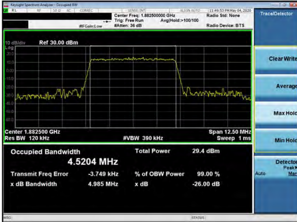
Plot 7-155. Occupied Bandwidth Plot (Band 25/2 - 5.0MHz 64-QAM - Full RB Configuration)
