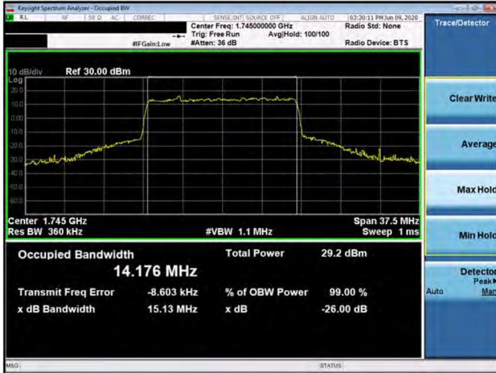
Plot 7-137. Occupied Bandwidth Plot (n66 15MHz 16QAM-CP-OFDM - Full RB Configuration)
