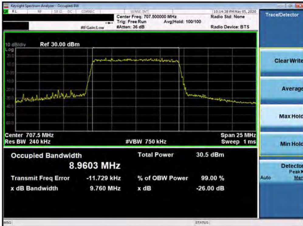
Plot 7-50. Occupied Bandwidth Plot (Band 12 - 10.0MHz 16-QAM - Full RB Configuration)
