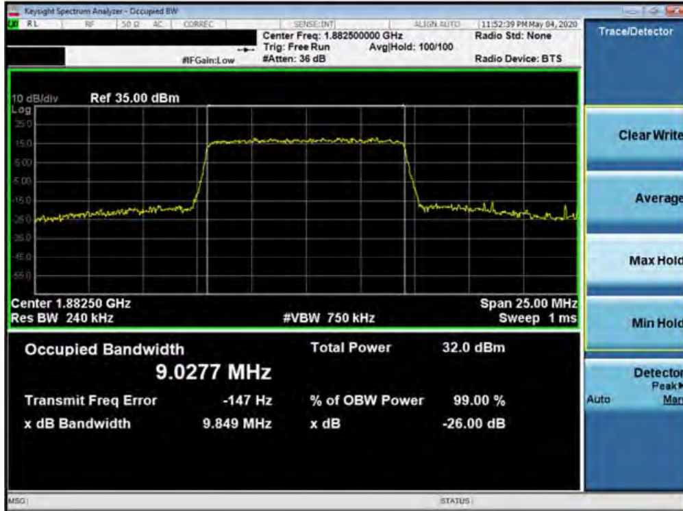
Plot 7-157. Occupied Bandwidth Plot (Band 25/2 - 10.0MHz QPSK - Full RB Configuration)
