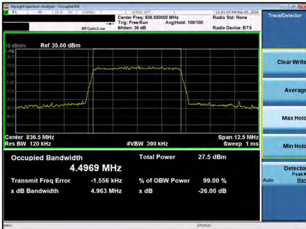
Plot 7-72. Occupied Bandwidth Plot (Band 26/5 - 5.0MHz 256-QAM - Full RB Configuration)
