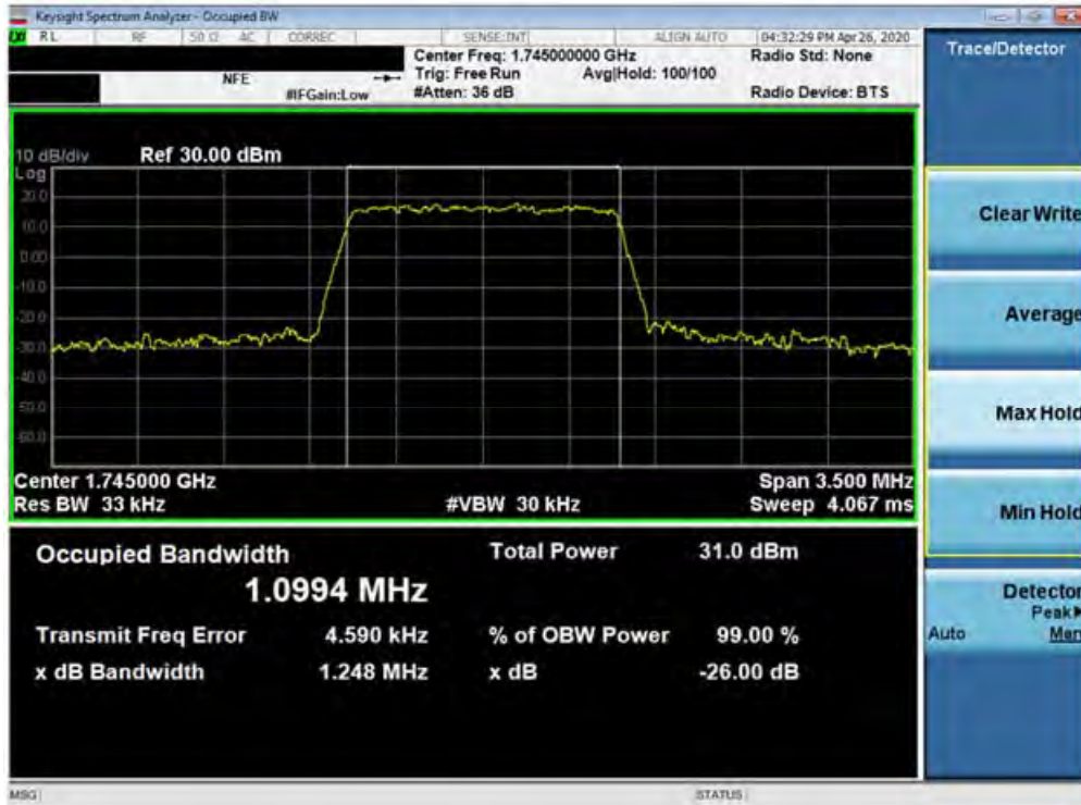
Plot 7-102. Occupied Bandwidth Plot (Band 66/4 - 1.4MHz 16-QAM - Full RB Configuration)
