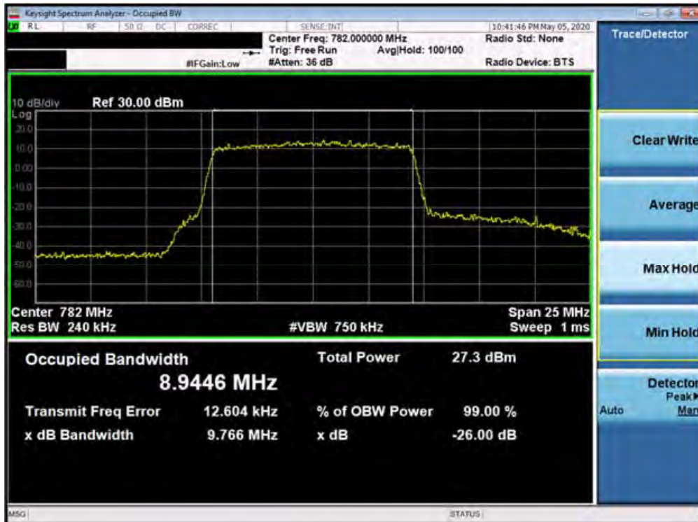
Plot 7-60. Occupied Bandwidth Plot (Band 13 - 10.0MHz 256-QAM - Full RB Configuration)
