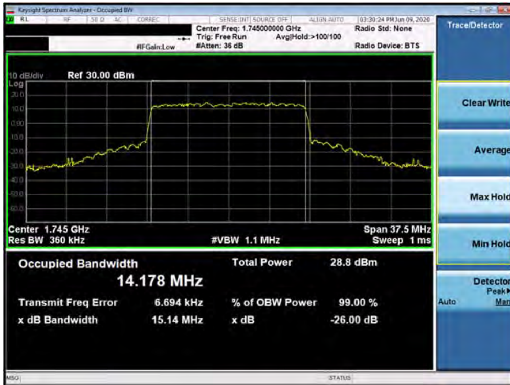
Plot 7-138. Occupied Bandwidth Plot (n66 15MHz 64QAM-CP-OFDM- Full RB Configuration)
