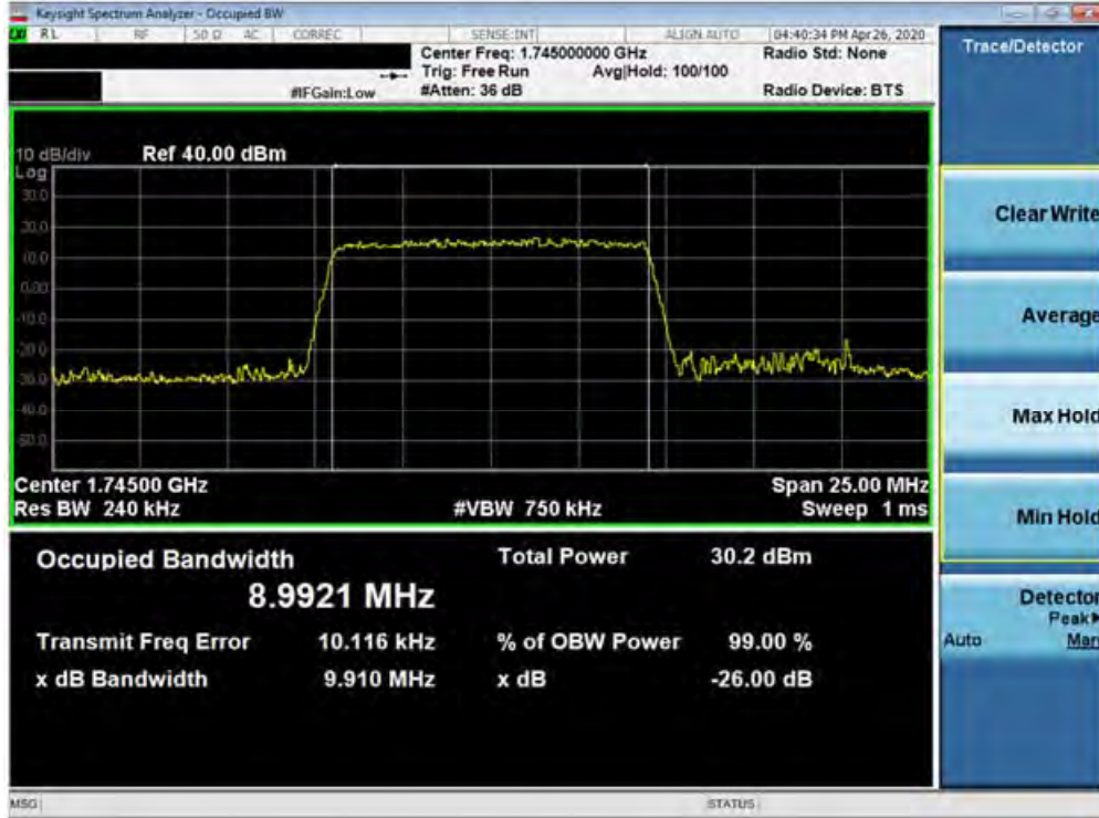
Plot 7-115. Occupied Bandwidth Plot (Band 66/4 - 10.0MHz 64-QAM - Full RB Configuration)
