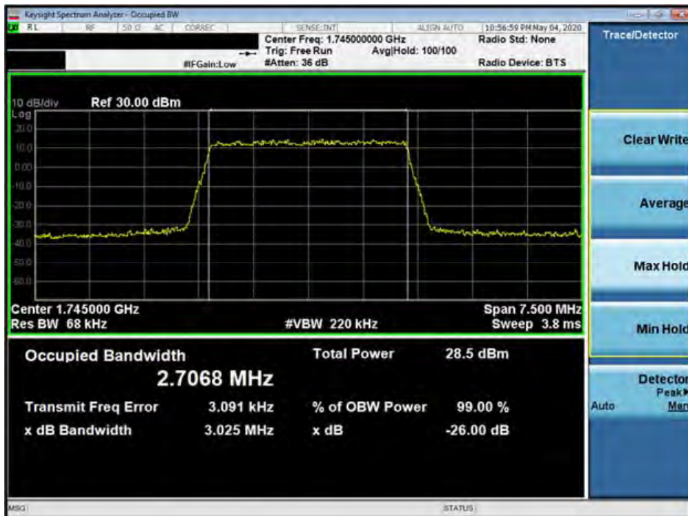
Plot 7-108. Occupied Bandwidth Plot (Band 66/4 - 3.0MHz 256-QAM - Full RB Configuration)
