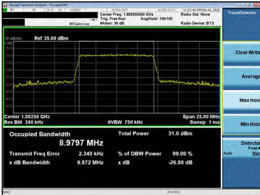
Plot 7-158. Occupied Bandwidth Plot (Band 25/2 - 10.0MHz 16-QAM - Full RB Configuration)
