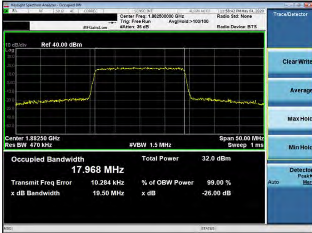
Plot 7-165. Occupied Bandwidth Plot (Band 25/2 - 20.0MHz QPSK - Full RB Configuration)
