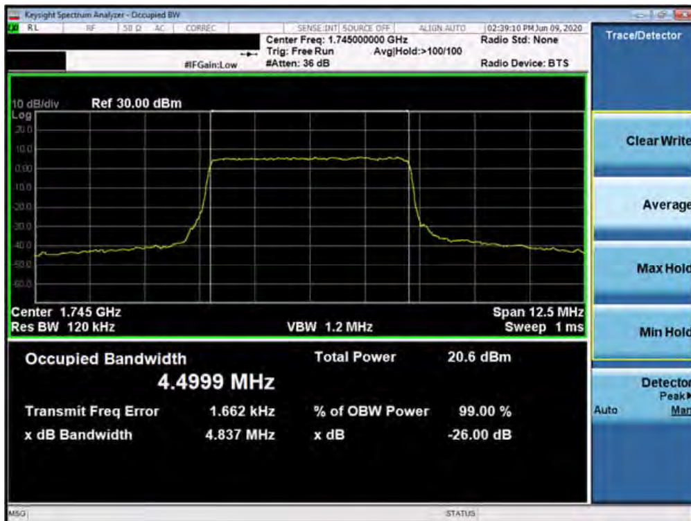
Plot 7-128. Occupied Bandwidth Plot (n66 5MHz 64QAM-CP-OFDM- Full RB Configuration)
