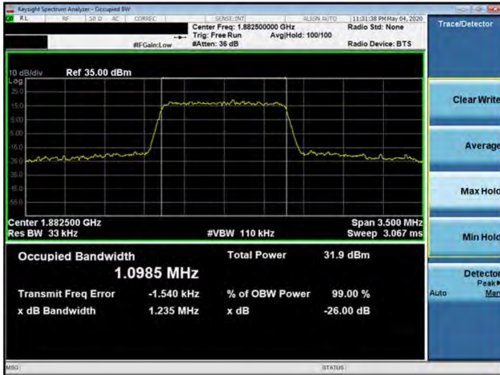
Plot 7-145. Occupied Bandwidth Plot (Band 25/2 - 1.4MHz QPSK - Full RB Configuration)
