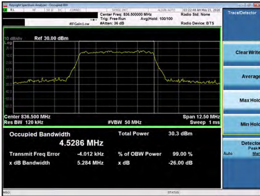
Plot 7-84. Occupied Bandwidth Plot (n5 5MHz 64QAM-CP-OFDM- Full RB Configuration)
