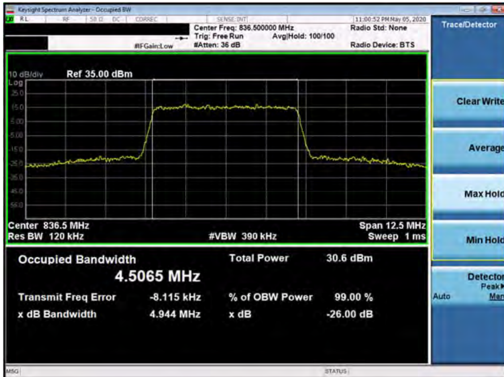
Plot 7-70. Occupied Bandwidth Plot (Band 26/5 - 5.0MHz 16-QAM - Full RB Configuration)
