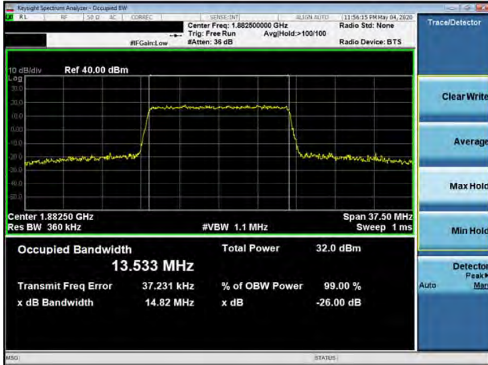
Plot 7-161. Occupied Bandwidth Plot (Band 25/2 - 15.0MHz QPSK - Full RB Configuration)
