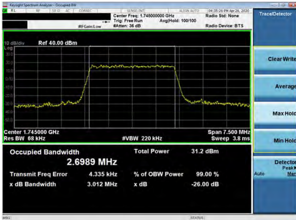
Plot 7-106. Occupied Bandwidth Plot (Band 66/4 - 3.0MHz 16-QAM - Full RB Configuration)
