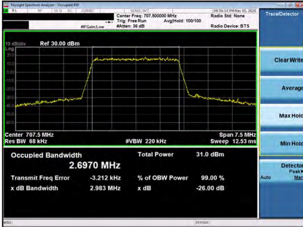
Plot 7-41. Occupied Bandwidth Plot (Band 12 - 3.0MHz QPSK - Full RB Configuration)
