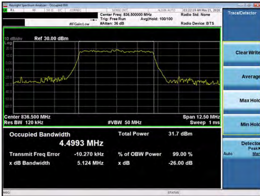
Plot 7-82. Occupied Bandwidth Plot (n5 5MHz QPSK-CP-OFDM - Full RB Configuration)
