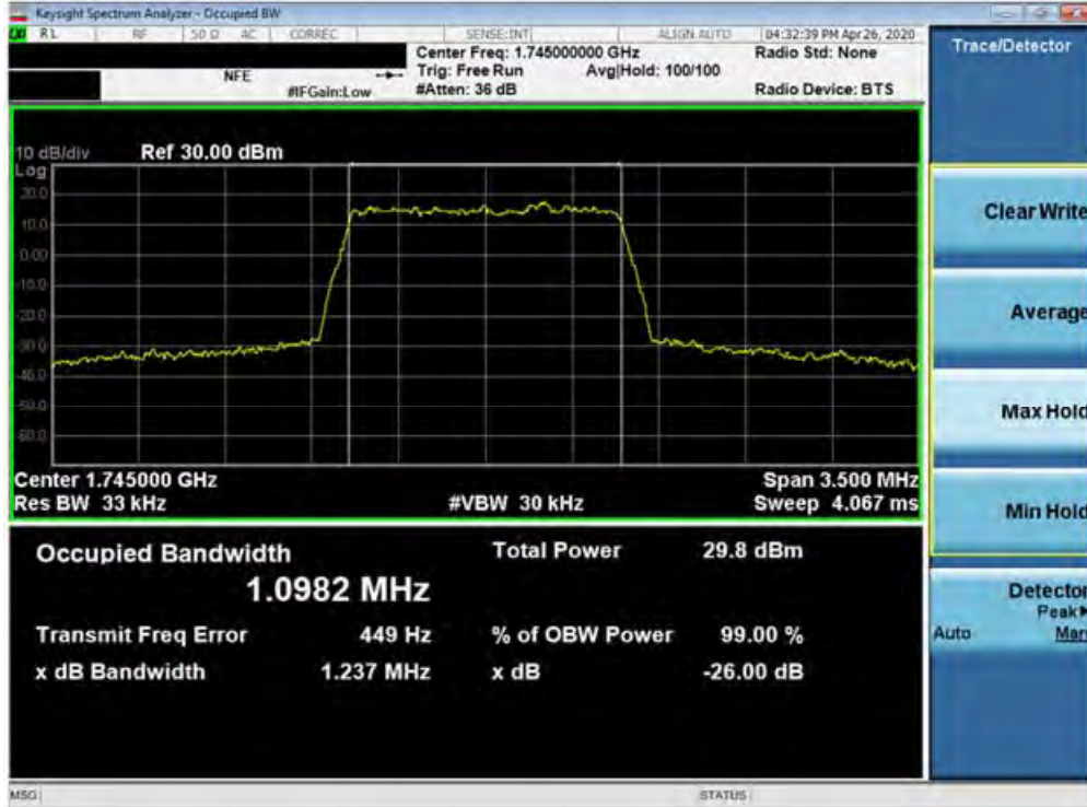
Plot 7-103. Occupied Bandwidth Plot (Band 66/4 - 1.4MHz 64-QAM - Full RB Configuration)
