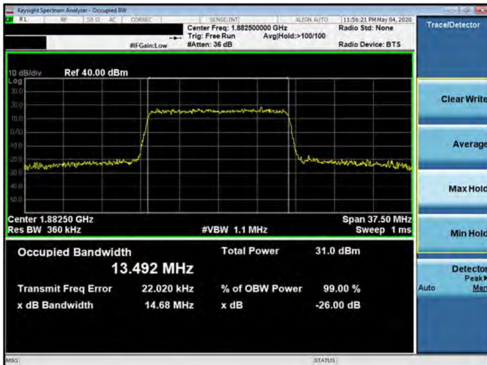
Plot 7-162. Occupied Bandwidth Plot (Band 25/2 - 15.0MHz 16-QAM - Full RB Configuration)
