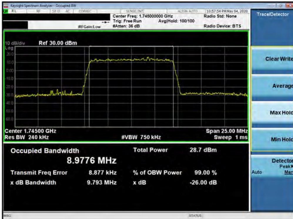
Plot 7-116. Occupied Bandwidth Plot (Band 66/4 - 10.0MHz 256-QAM - Full RB Configuration)
