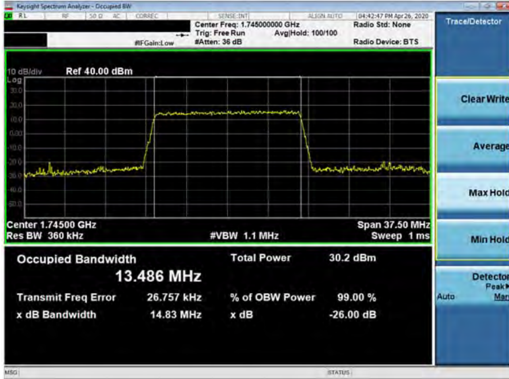
Plot 7-119. Occupied Bandwidth Plot (Band 66/4 - 15.0MHz 64-QAM - Full RB Configuration)
