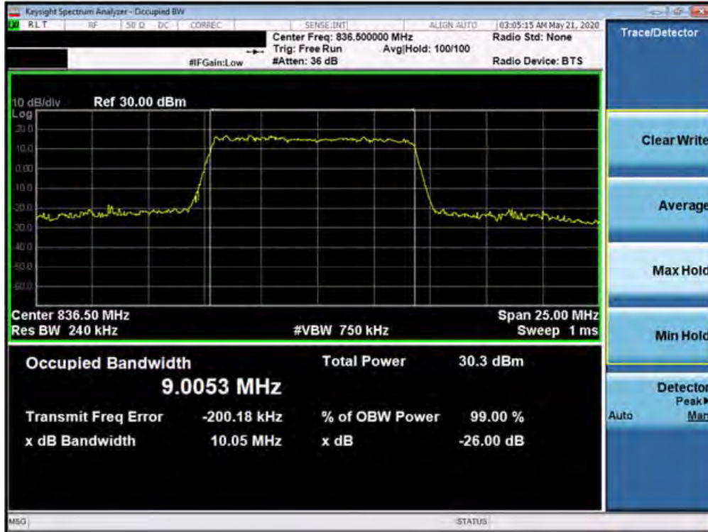
Plot 7-89. Occupied Bandwidth Plot (n5 10MHz 64QAM-CP-OFDM- Full RB Configuration)
