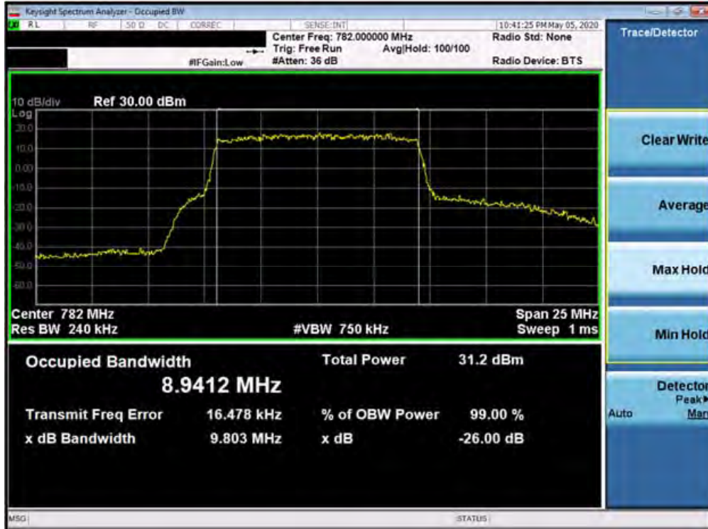
Plot 7-57. Occupied Bandwidth Plot (Band 13 - 10.0MHz QPSK - Full RB Configuration)
