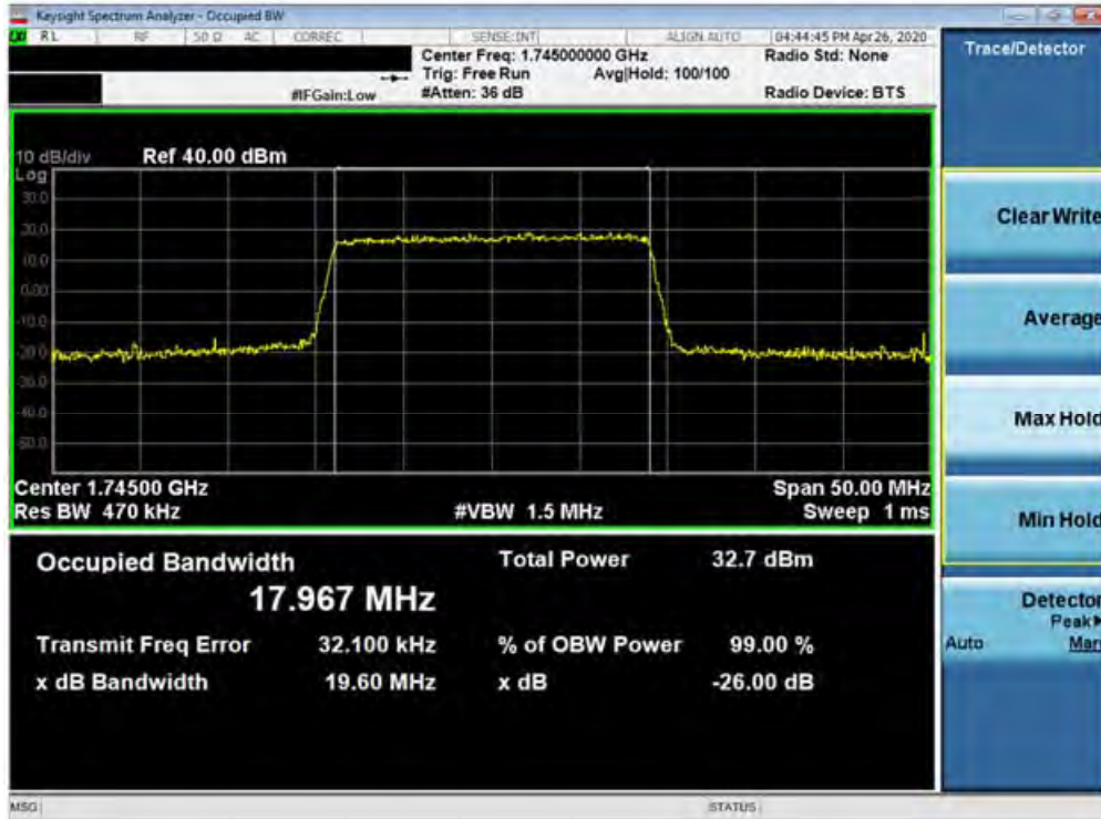
Plot 7-121. Occupied Bandwidth Plot (Band 66/4 - 20.0MHz QPSK - Full RB Configuration)
