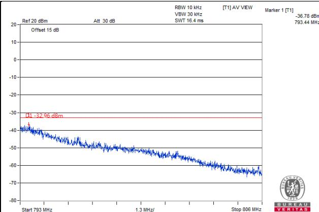
Note: For the 763 - 775 MHz and 793 - 805 MHz band, the FCC by a factor not less  $65 + 10\log(P[\text{watt}])$  in a 6.25 kHz band segment. Since it was not possible to set the resolution bandwidth to 6.25 kHz with the available equipment, a bandwidth of 10 kHz was used instead to show compliance. By using a 10 kHz bandwidth on the spectrum analyzer. And Limit line is -35 dBm.
