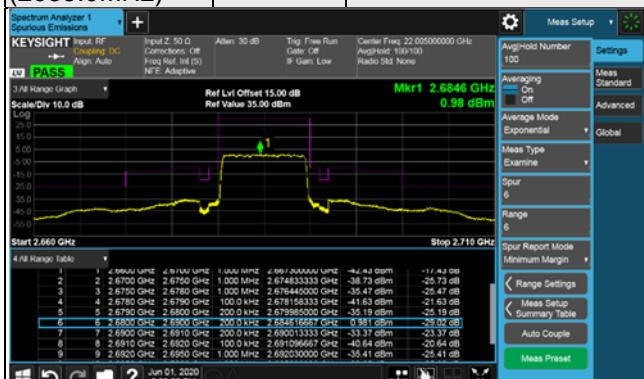
Note: By using a 100 kHz bandwidth on the spectrum analyzer, the correction factor is further improved by 10
