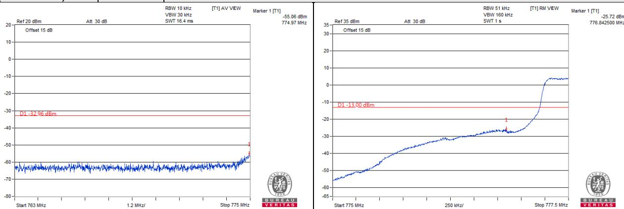
Note: For the 763 - 775 MHz and 793 - 805 MHz band, the FCC by a factor not less  $65+10\log(P[\text{watt}])$  in a 6.25 kHz band segment. Since it was not possible to set the resolution bandwidth to 6.25 kHz with the available equipment, a bandwidth of 10 kHz was used instead to show compliance. By using a 10 kHz bandwidth on the spectrum analyzer. And Limit line is -35 dBm.
