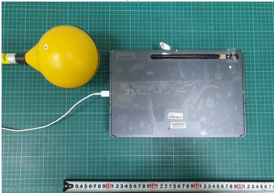
H-Field (Charging Mode - Bottom)
