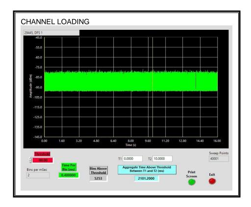
The level of traffic loading on the channel by the EUT is 21.01%.
