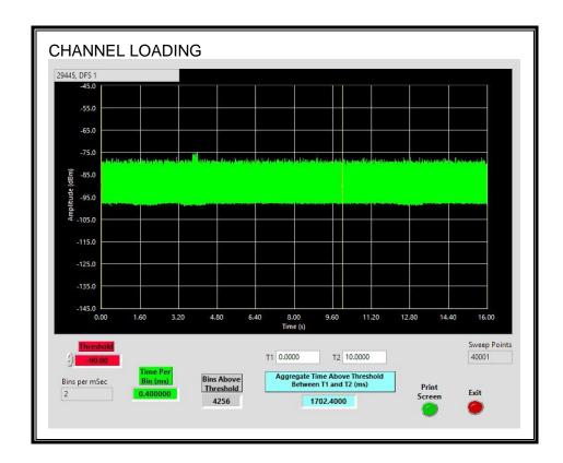
The level of traffic loading on the channel by the EUT is 17.02%.
