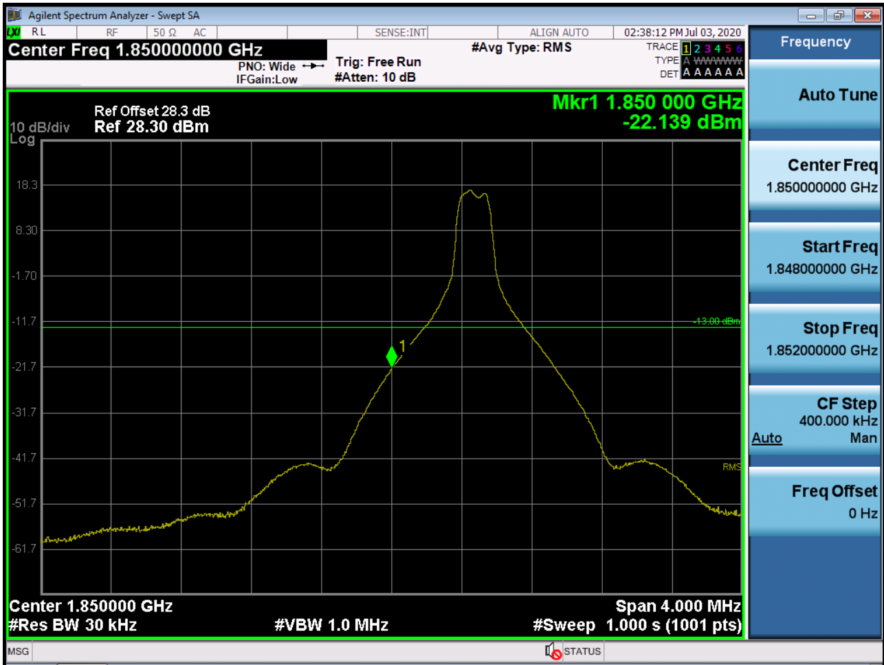
Sub6 n25(2). Lower Band Edge Plot (15M BW Ch.371500 BPSK_RB1_Offset 0)
