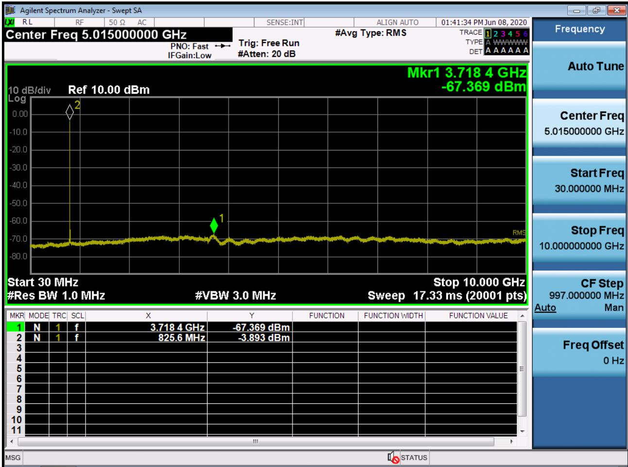
BAND 26. Conducted Spurious (26915ch\_15MHz\_QPSK\_RB 1\_0)
