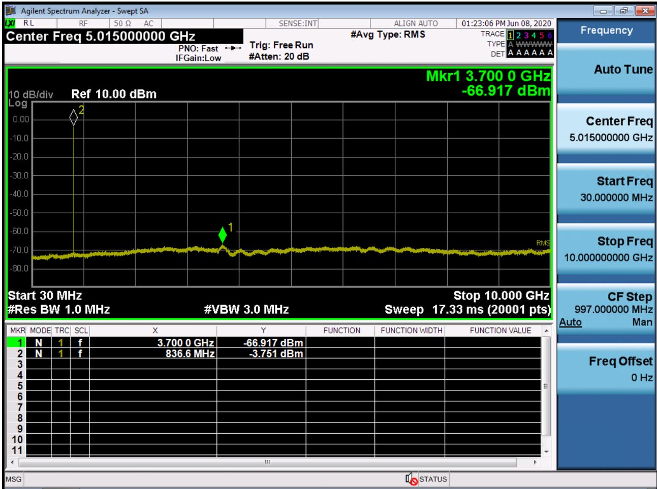
BAND5/ 26. Conducted Spurious Plot (27033ch\_1.4MHz\_QPSK\_RB 1\_0)
