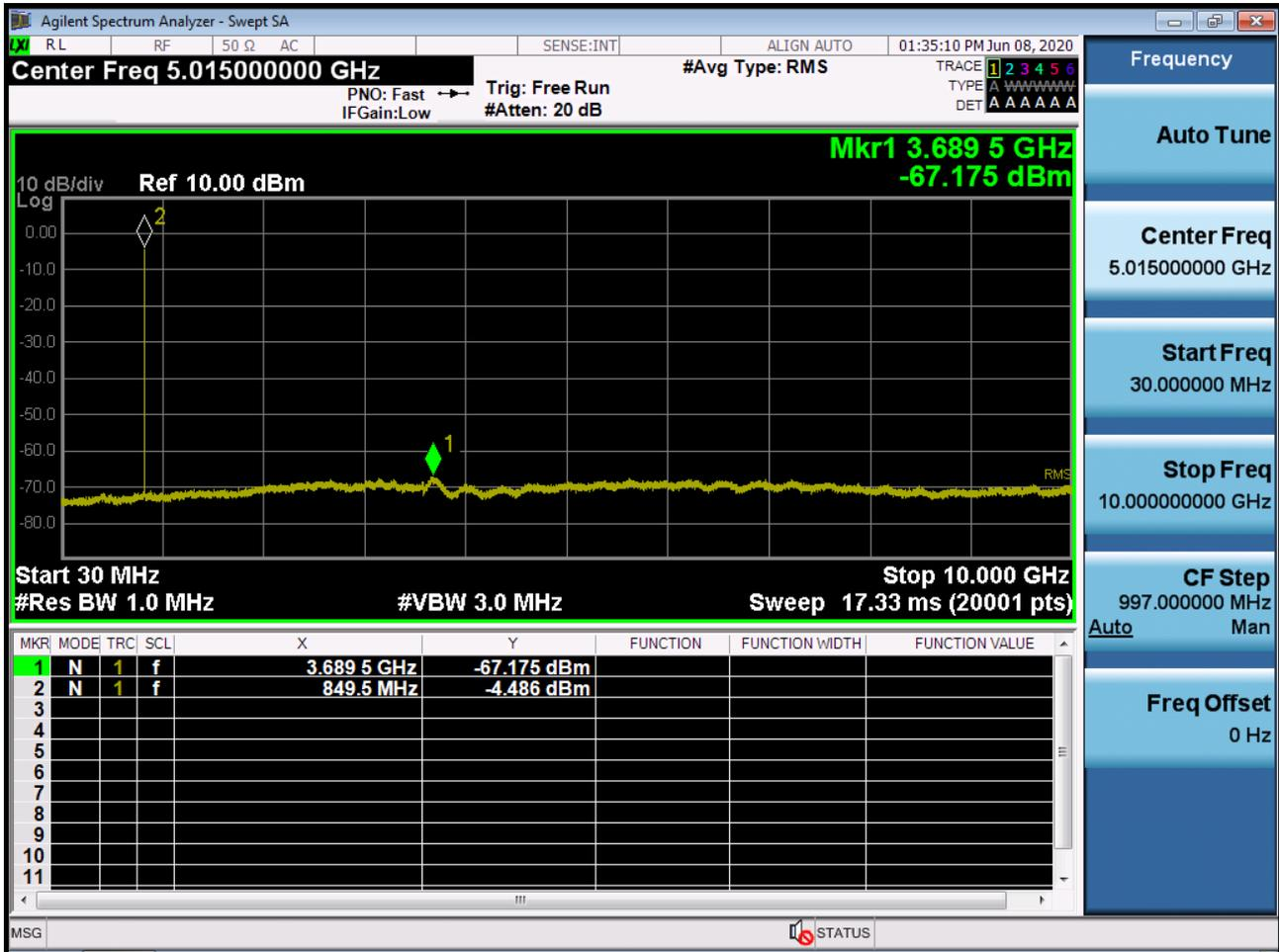
BAND5/ 26. Conducted Spurious Plot (26840ch\_10MHz\_QPSK\_RB 1\_0)
