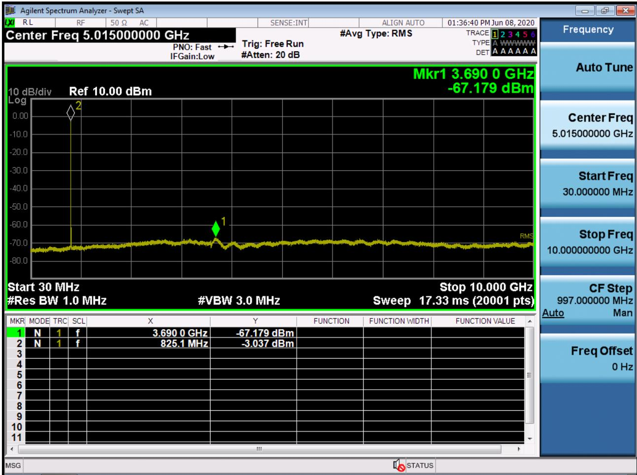
BAND5/ 26. Conducted Spurious Plot (26915ch\_10MHz\_QPSK\_RB 1\_0)
