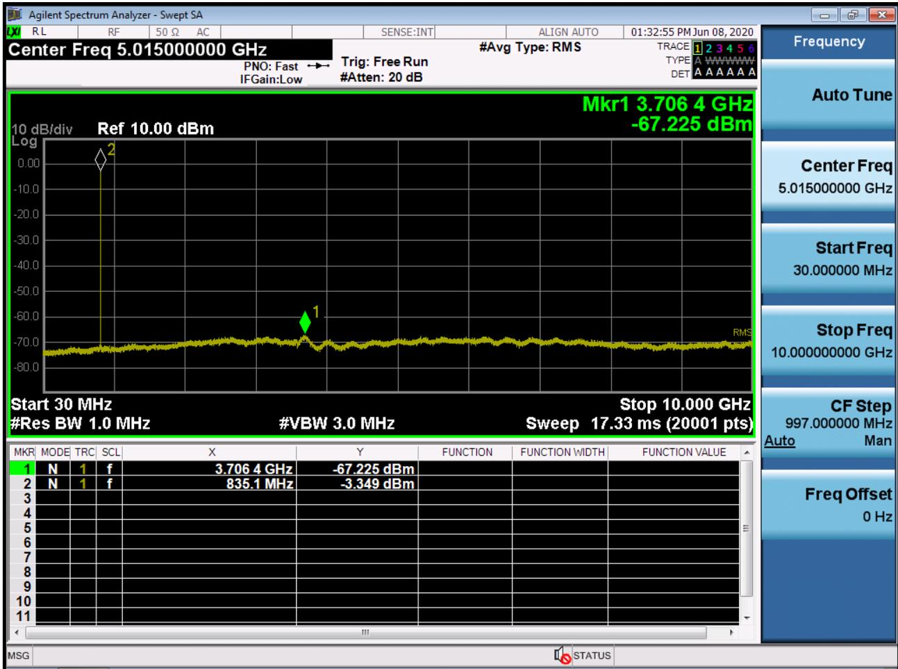
BAND5/ 26. Conducted Spurious Plot (27015ch\_5MHz\_QPSK\_RB 1\_0)
