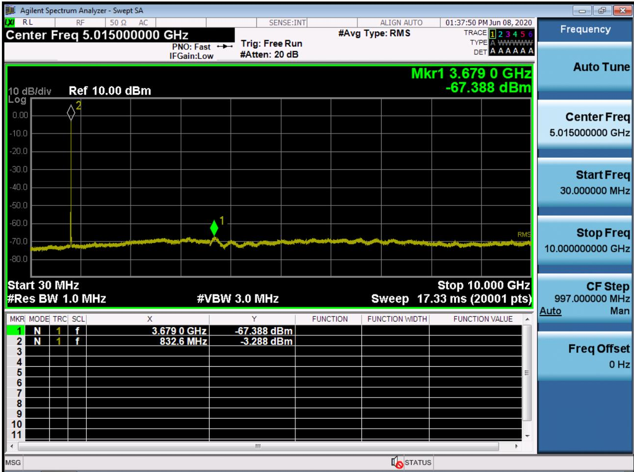
BAND5/ 26. Conducted Spurious Plot (26990ch\_10MHz\_QPSK\_RB 1\_0)
