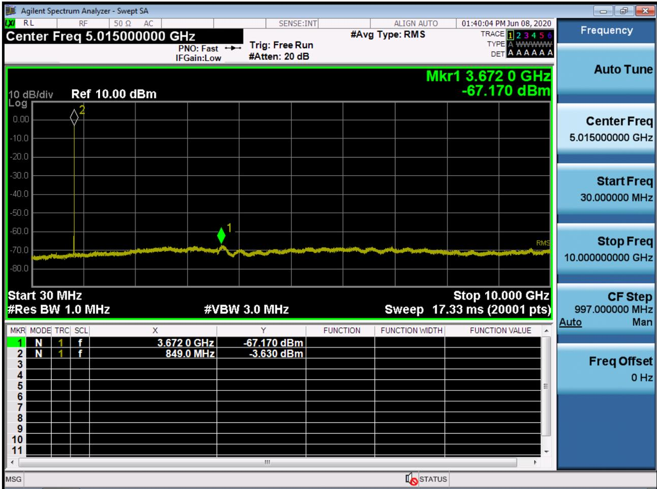
BAND 26. Conducted Spurious (26865ch\_15MHz\_QPSK\_RB 1\_0)
