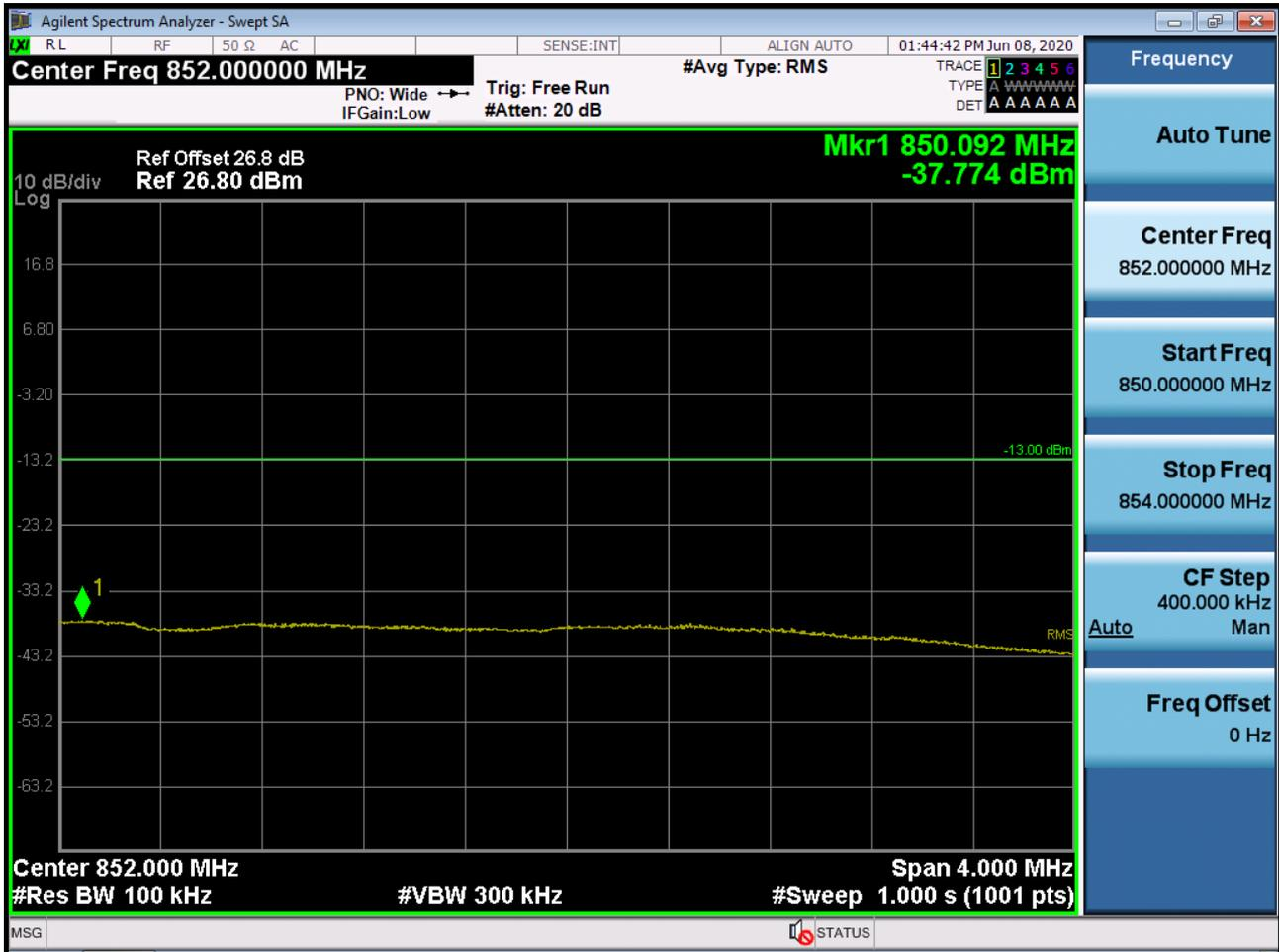
BAND5/ 26. Conducted Spurious Plot (26915ch\_1.4MHz\_QPSK\_RB 1\_0)
