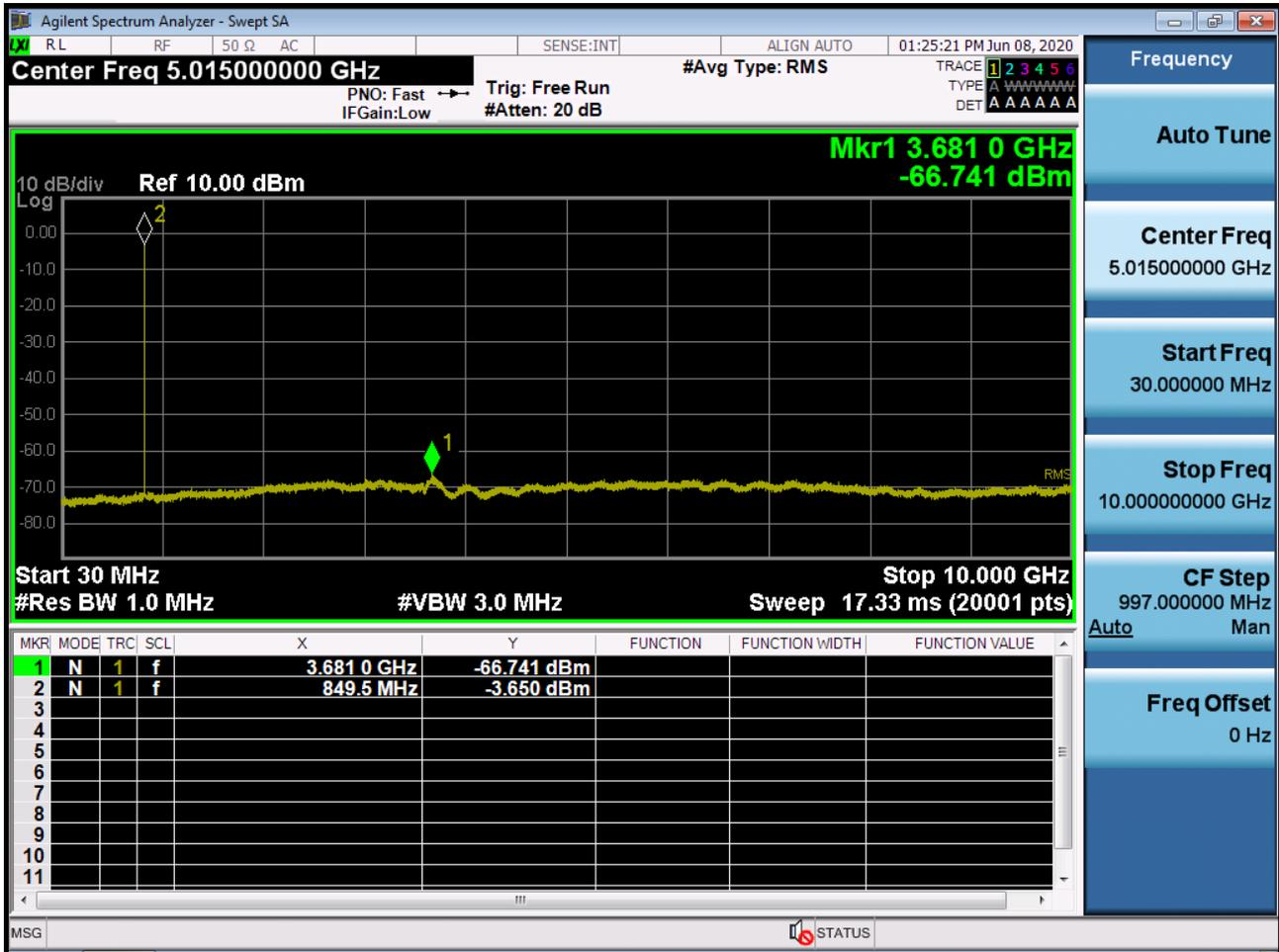
BAND5/ 26. Conducted Spurious Plot (26915ch\_3MHz\_QPSK\_RB 1\_0)
