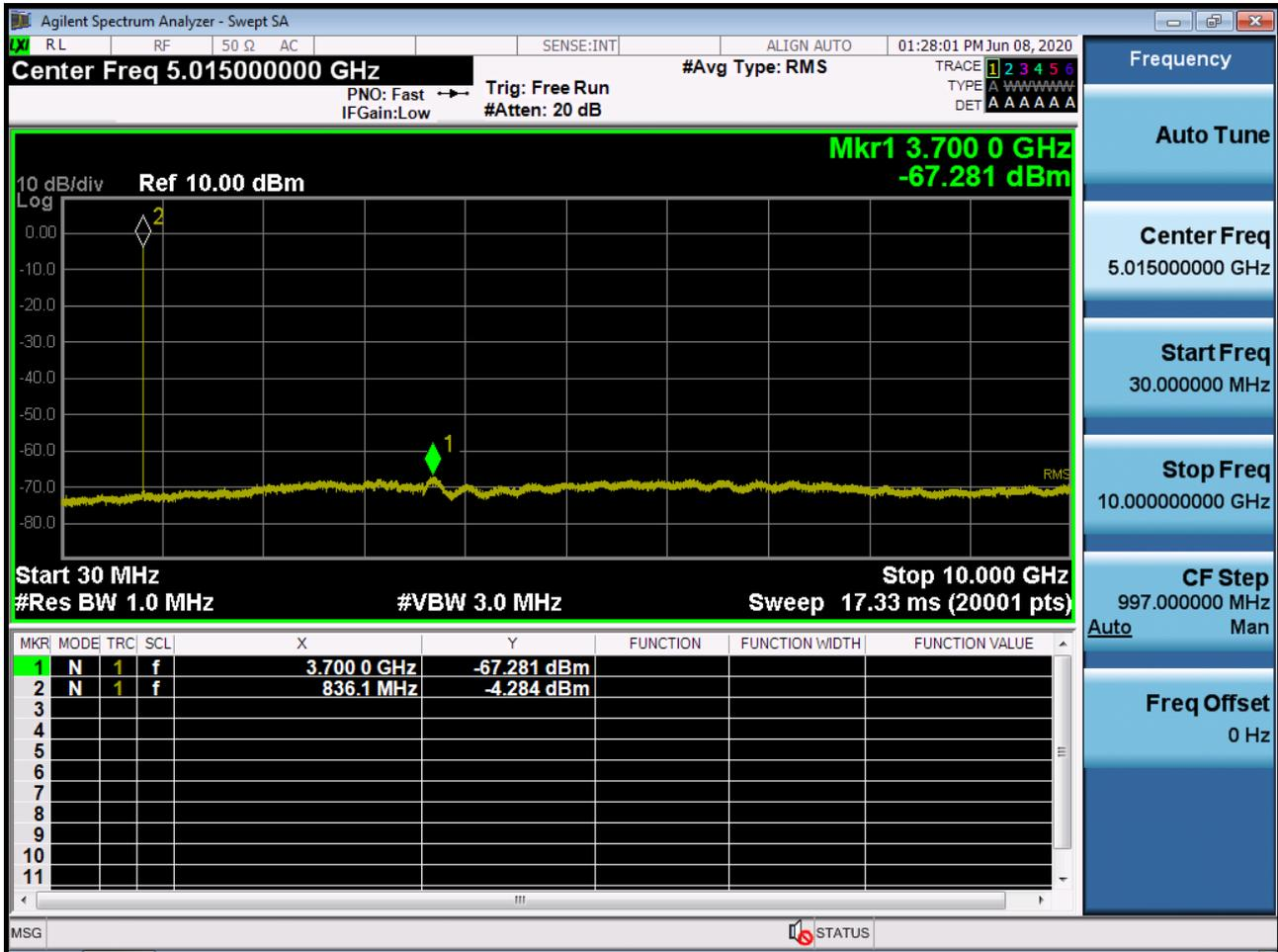
BAND5/ 26. Conducted Spurious Plot (26915ch\_5MHz\_QPSK\_RB 1\_0)
