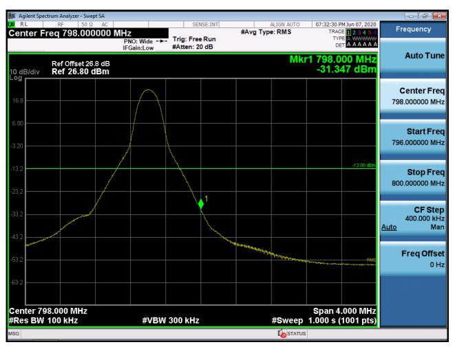
BAND 14 Upper Band Edge Plot (10M BW Ch.23330 QPSK\_RB1\_Offset\_49)
