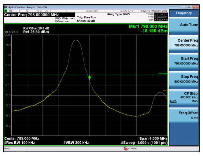
BAND 14 Upper Band Edge Plot (5M BW Ch.23355 QPSK\_RB1\_Offset 24)
