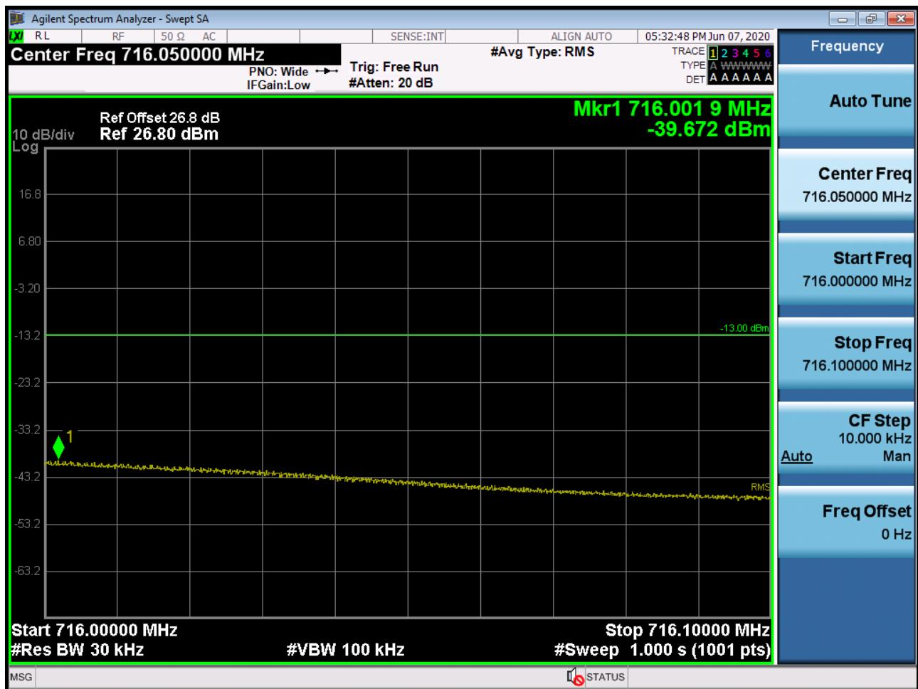
BAND 12. Upper Band Edge Plot (10M BW Ch.23130 QPSK\_RB1\_Offset 49)\_2
