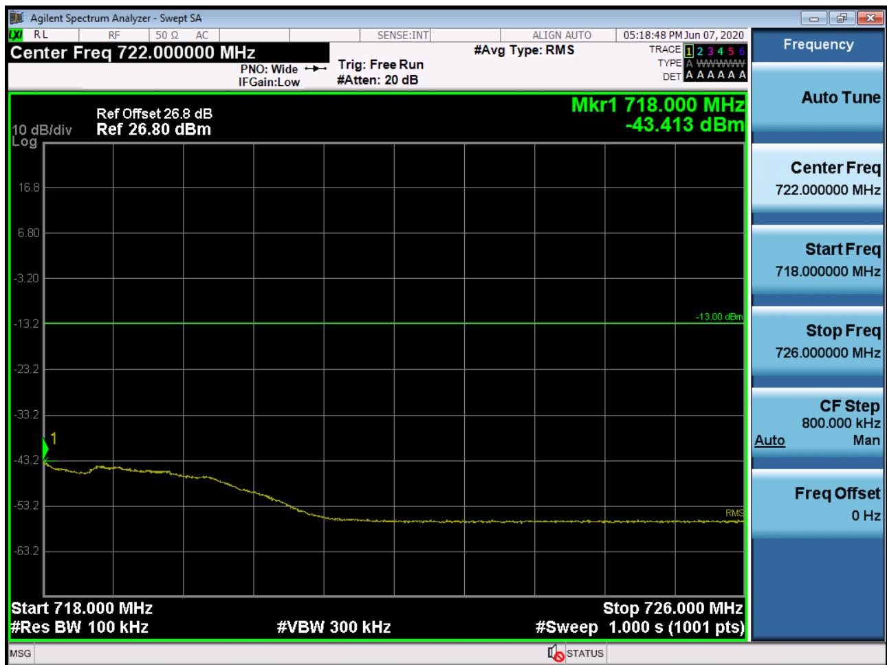
BAND 12. Upper Band Edge Plot (5M BW Ch.23155 QPSK\_RB1\_Offset 24)\_1
