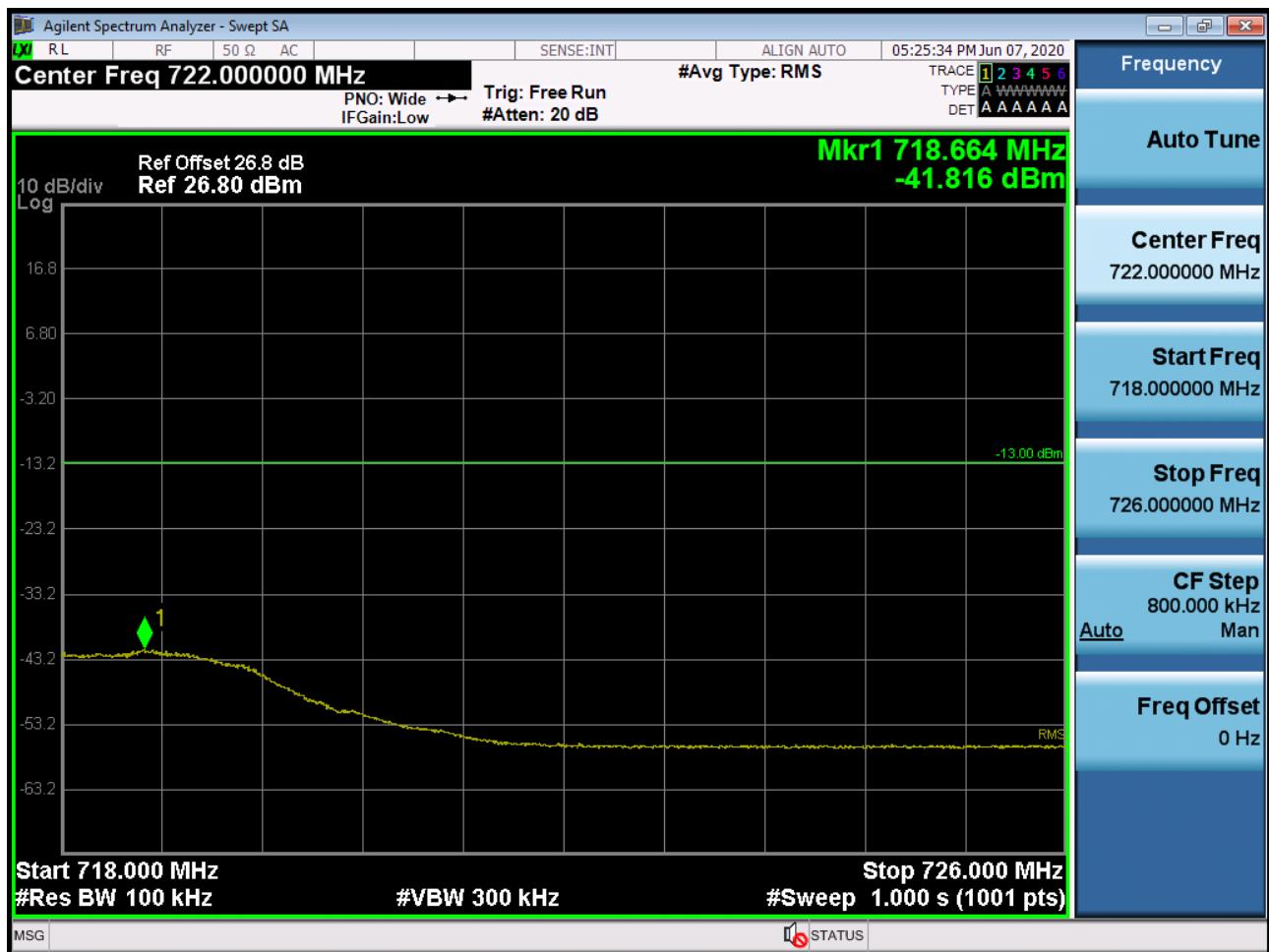
BAND 12. Upper Band Edge Plot (10M BW Ch.23130 QPSK\_RB1\_Offset 49)\_1
