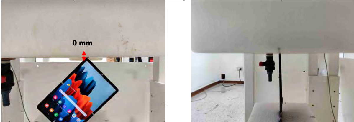
Fig.9 EUT Left corner side to flat phantom
