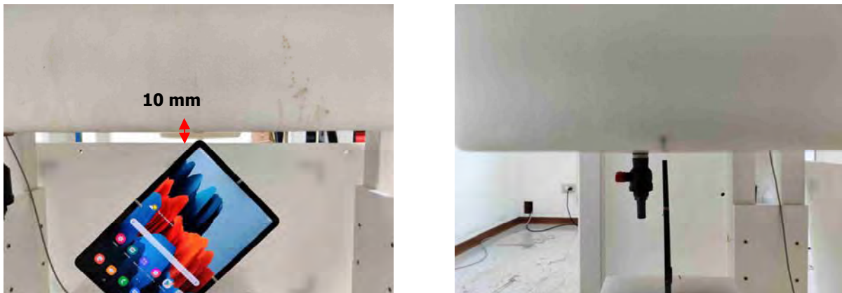
Fig.13 EUT Left corner side to flat phantom
