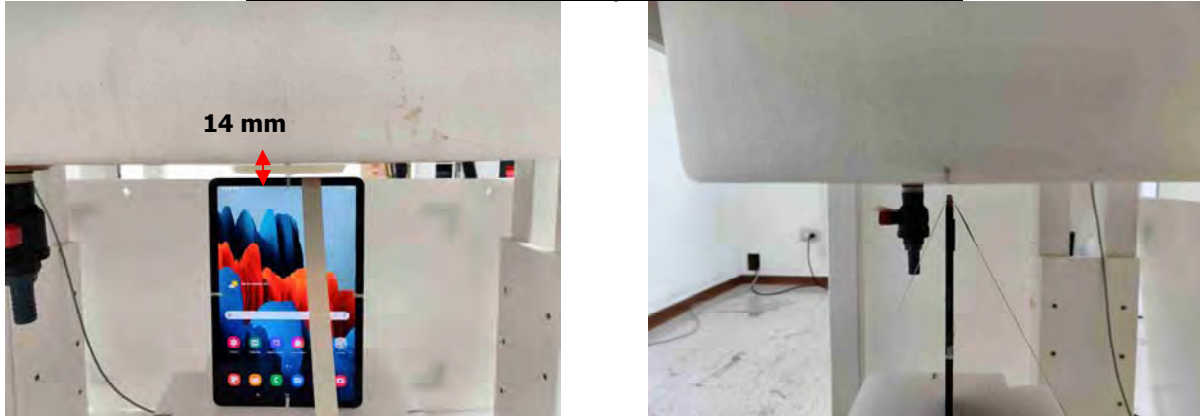
Fig.16 EUT Top side to flat phantom
