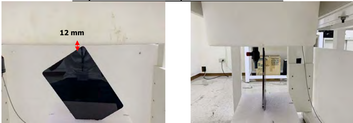
Fig.15 EUT Right corner side to flat phantom
