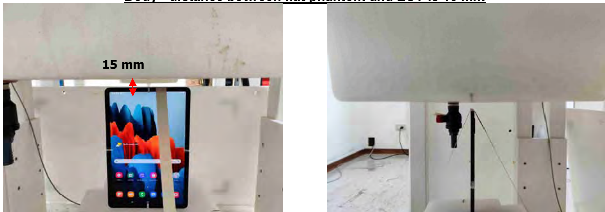
Fig.17 EUT Top side to flat phantom
