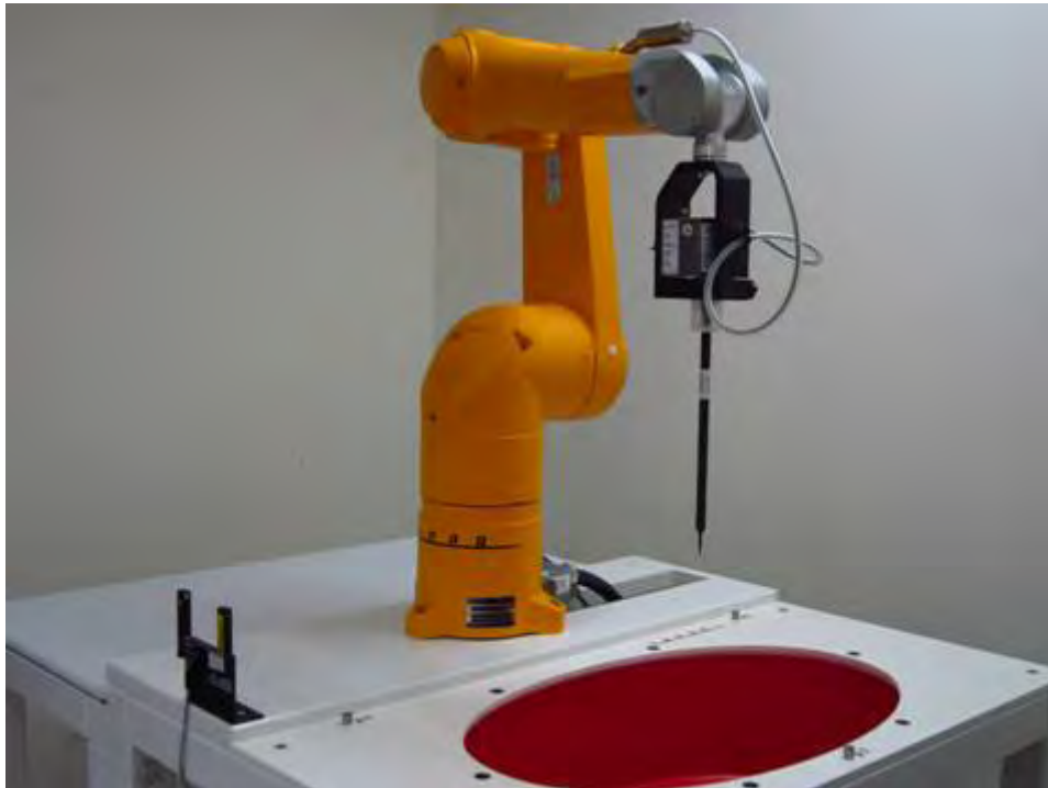
Fig.1 Photograph of the SAR measurement system
