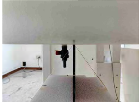
Fig.6 EUT Right side to flat phantom
