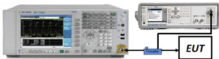
Figure 7-7. Test Instrument & Measurement Setup
