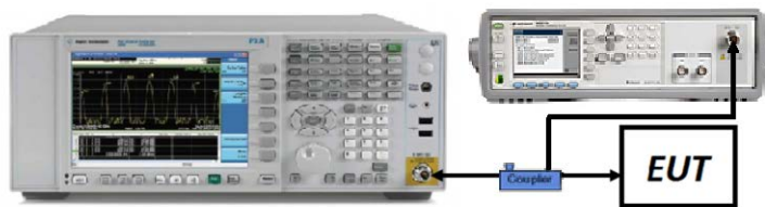
Figure 7-4. Test Instrument & Measurement Setup
