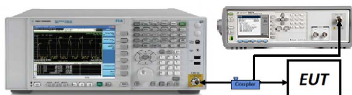
Figure 7-6. Test Instrument & Measurement Setup
