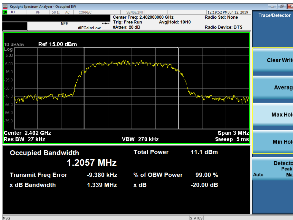
Plot 7-7. 20dB Bandwidth Plot (Bluetooth, 3Mbps – Ch. 0)
