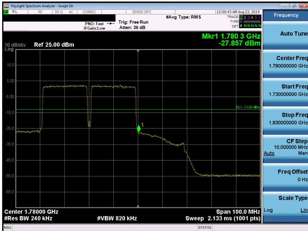
Plot 7-381. Upper Band Edge Plot (Band 66- QPSK – PCC: 20 MHz SCC:20 MHz – Full RB)
