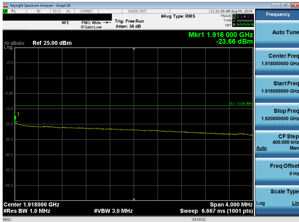
Plot 7-274. Upper Extended Band Edge Plot (Band 25 - 10.0MHz QPSK - Full RB Configuration)
