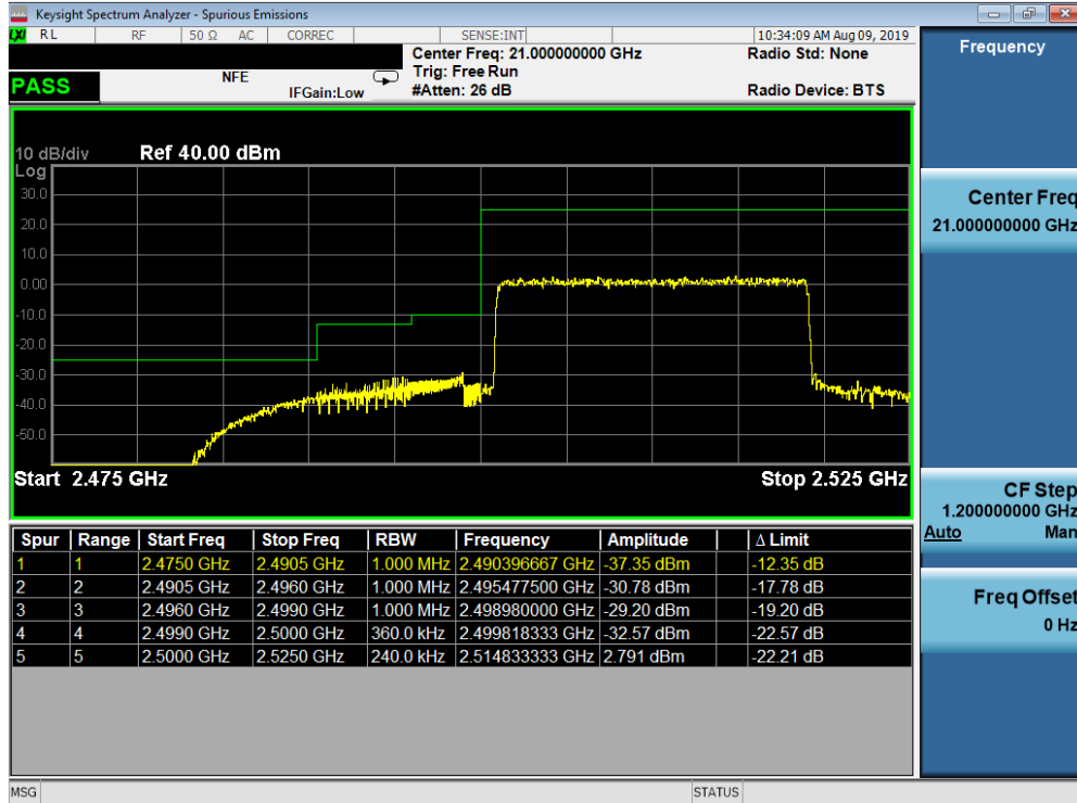
Plot 7-293. Lower ACP Plot (Band 7 - 20.0MHz QPSK - Full RB Configuration)
