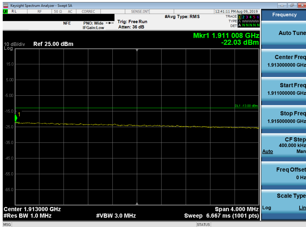
Plot 7-284. Upper Extended Band Edge Plot (Band 2 - 20.0MHz QPSK - Full RB Configuration)
