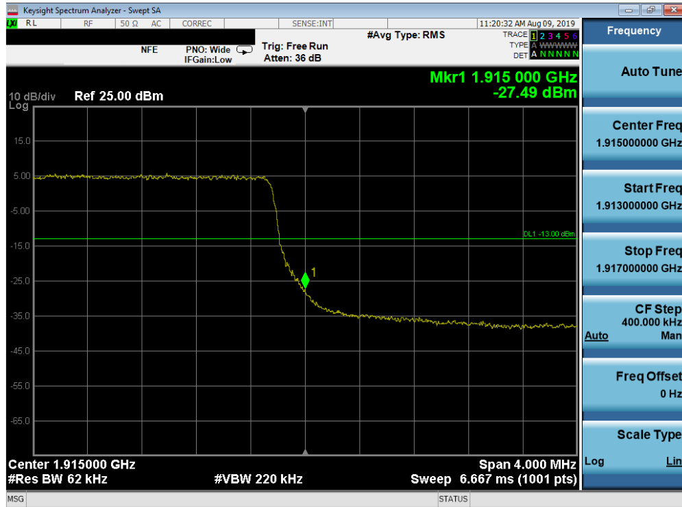
Plot 7-267. Upper Band Edge Plot (Band 25 - 5.0MHz QPSK - Full RB Configuration)
