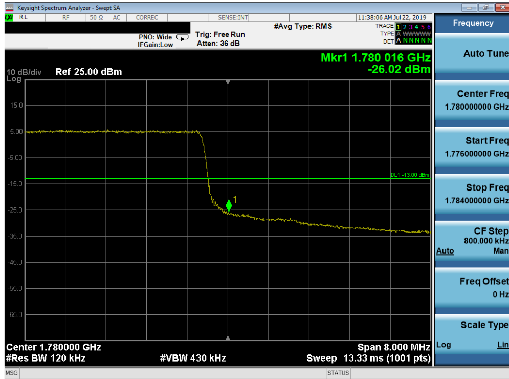
Plot 7-237. Upper Band Edge Plot (Band 66 - 10.0MHz QPSK - Full RB Configuration)
