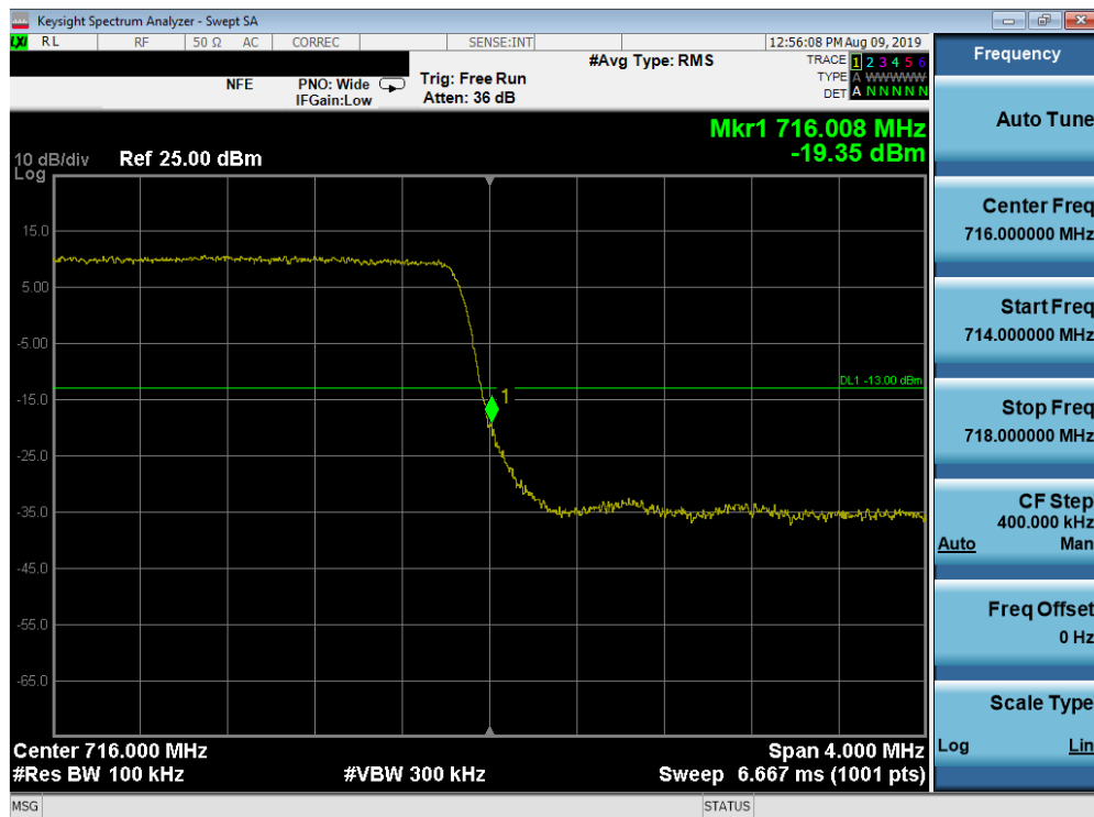
Plot 7-192. Upper Band Edge Plot (Band 12 - 3.0MHz QPSK - Full RB Configuration)
