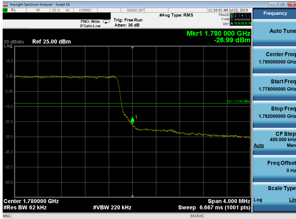
Plot 7-231. Upper Band Edge Plot (Band 66 - 5.0MHz QPSK - Full RB Configuration)
