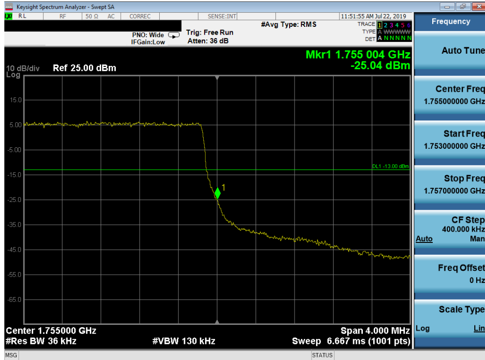
Plot 7-223. Upper Band Edge Plot (Band 4 - 3.0MHz QPSK - Full RB Configuration)
