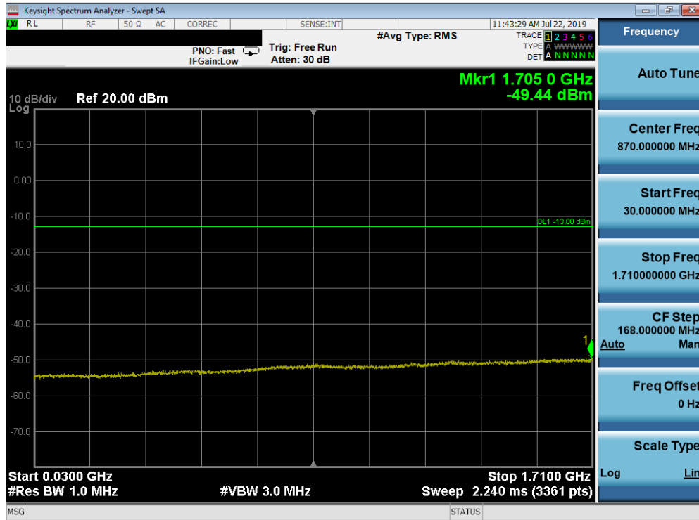
Plot 7-151. Conducted Spurious Plot (Band 66/4 - 15.0MHz QPSK - RB Size 1, RB Offset 0 - High Channel)
