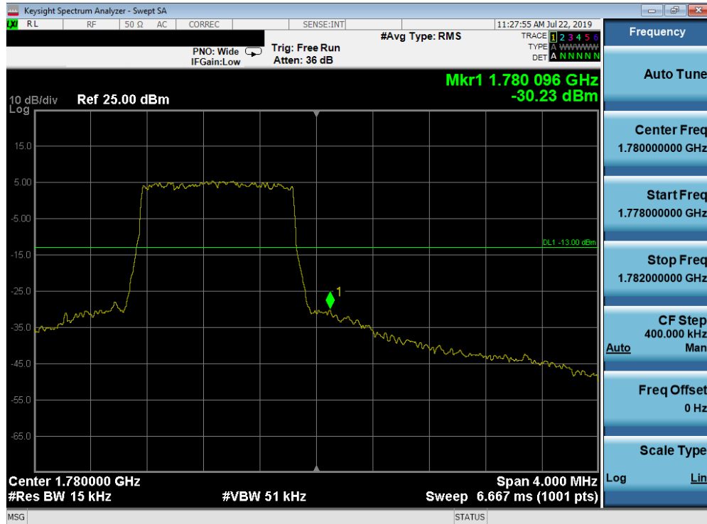
Plot 7-219. Upper Band Edge Plot (Band 66 - 1.4MHz QPSK - Full RB Configuration)
