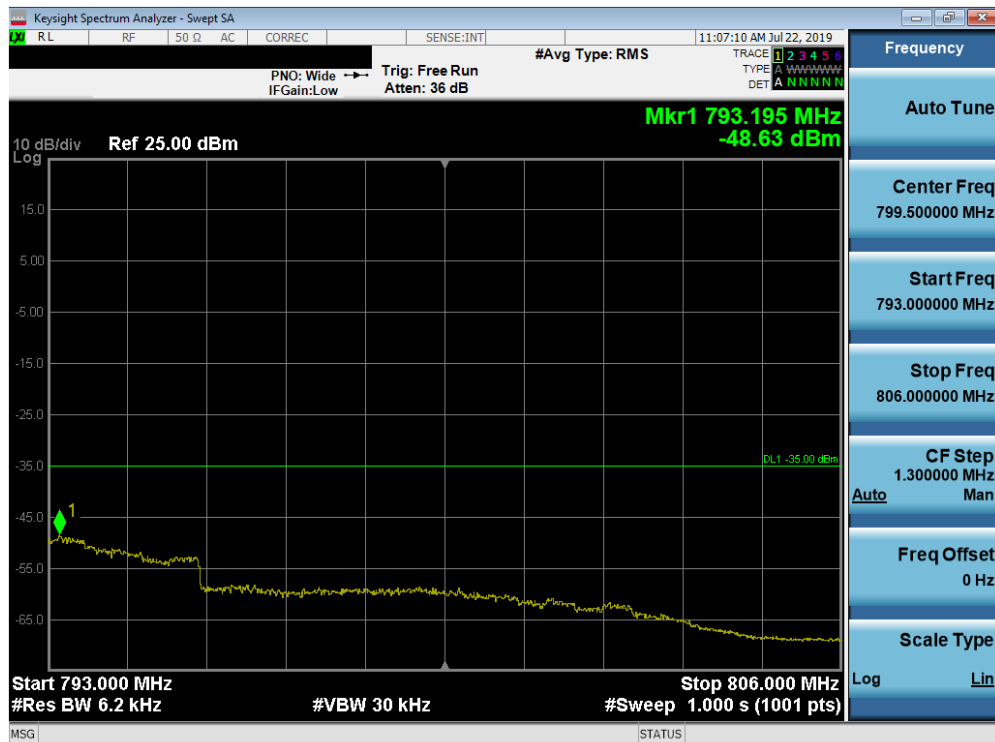
Plot 7-204. Upper Emission Mask Plot (Band 13 - 10.0MHz QPSK - Full RB Configuration)
