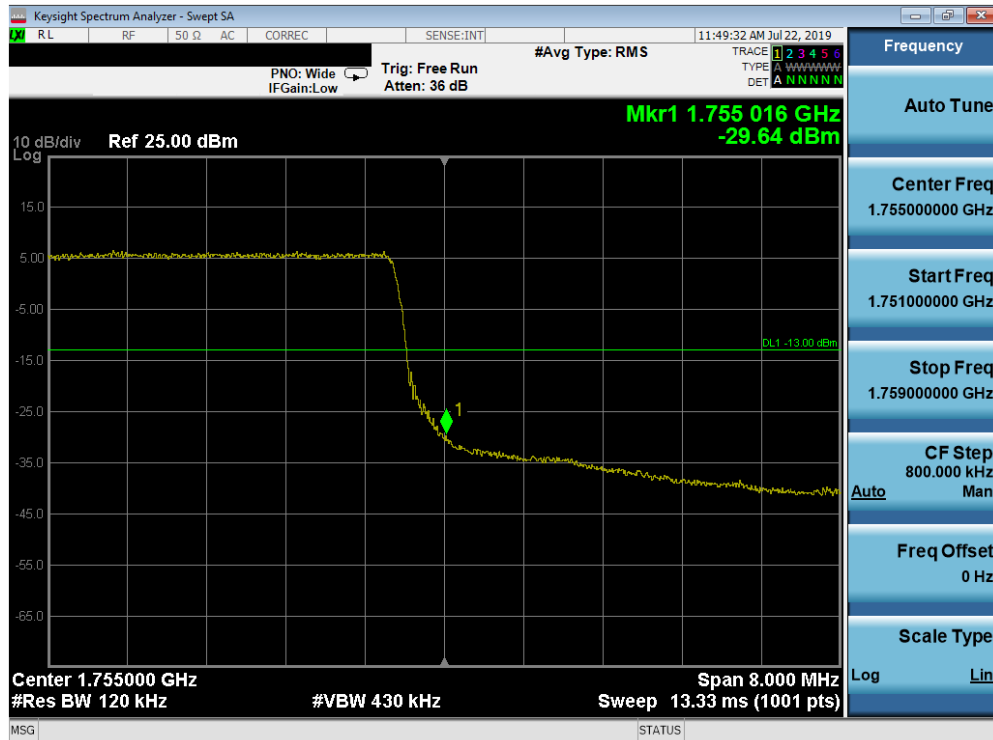
Plot 7-235. Upper Band Edge Plot (Band 4 - 10.0MHz QPSK - Full RB Configuration)
