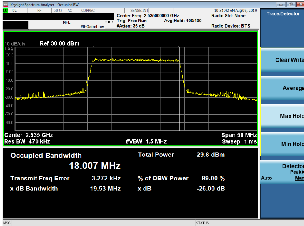
Plot 7-92. Occupied Bandwidth Plot (Band 7 - 20.0MHz 16-QAM - Full RB Configuration)
