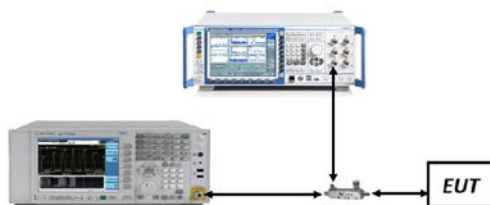
Figure 7-3. Test Instrument & Measurement Setup
