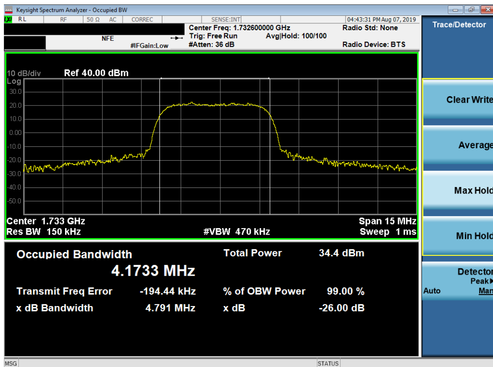
Plot 7-2. Occupied Bandwidth Plot (AWS WCDMA Mode)
