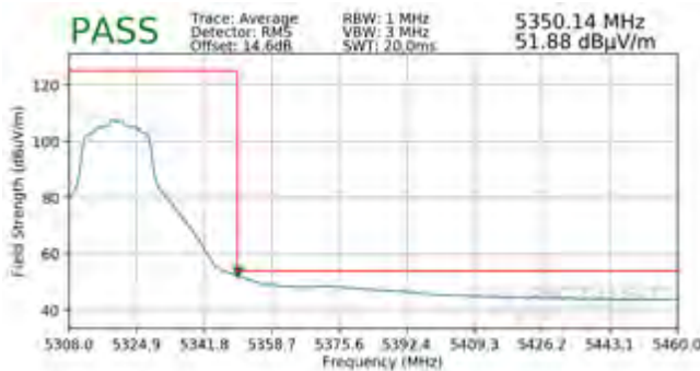
Plot 7-194. Radiated Upper Band Edge Plot SISO ANT2 (Average – UNII Band 2A)
