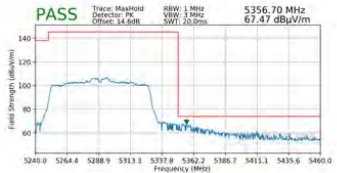
Plot 7-209. Radiated Upper Band Edge Plot SISO ANT2 (Peak – UNII Band 2A)
