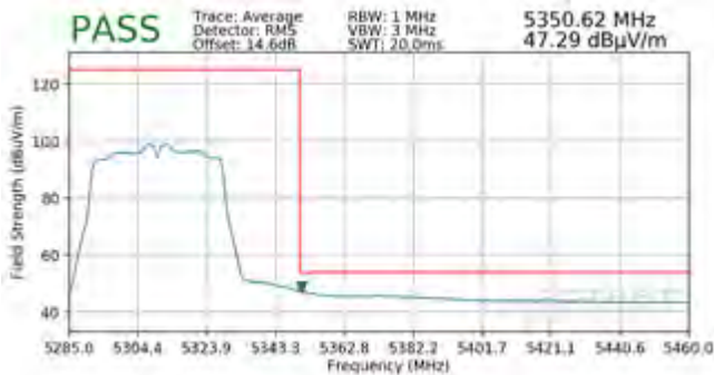
Plot 7-201. Radiated Upper Band Edge Plot SISO ANT2 (Average – UNII Band 2A)
