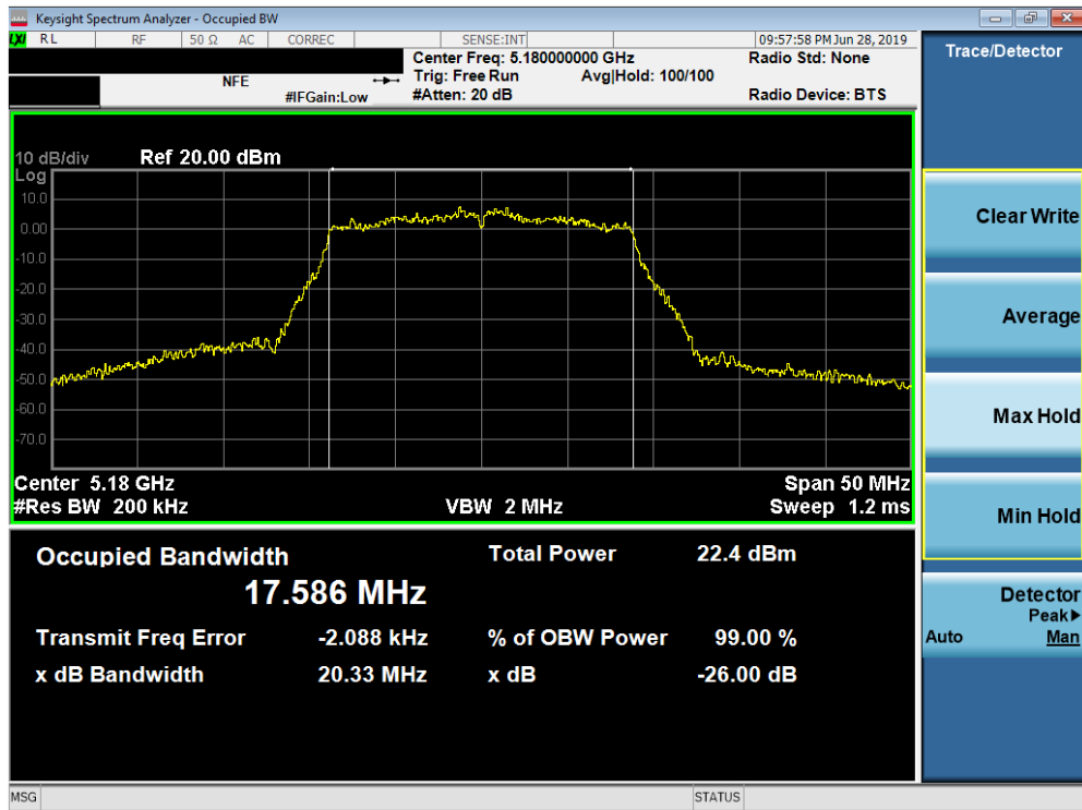
Plot 7-33. 26dB Bandwidth Plot SISO ANT2 (20MHz BW 802.11n (UNII Band 1) – Ch. 36)
