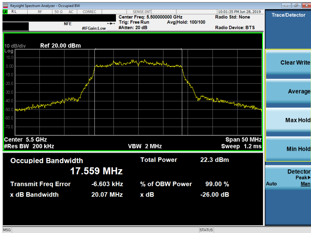
Plot 7-51. 26dB Bandwidth Plot SISO ANT2 (20MHz BW 802.11n (UNII Band 2C) – Ch. 100)
