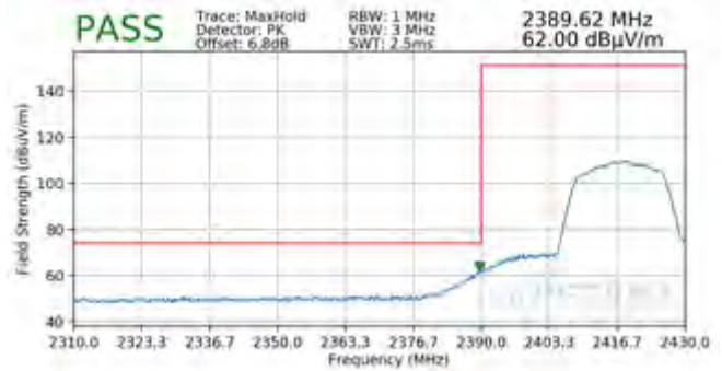
Plot 7-107. Radiated Restricted Lower Band Edge Measurement SISO ANT1 (Peak)
