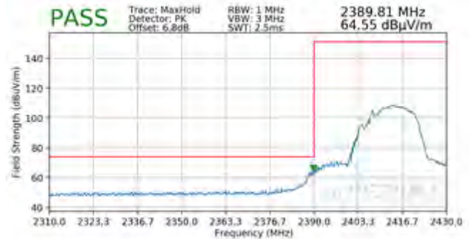
Plot 7-135. Radiated Restricted Lower Band Edge Measurement MIMO (Peak)
