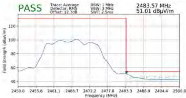
Plot 7-144. Radiated Restricted Upper Band Edge Measurement MIMO (Average)
