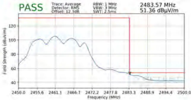
Plot 7-142. Radiated Restricted Upper Band Edge Measurement MIMO (Average)
