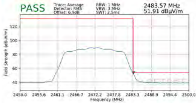
Plot 7-120. Radiated Restricted Upper Band Edge Measurement SISO ANT1 (Average)
