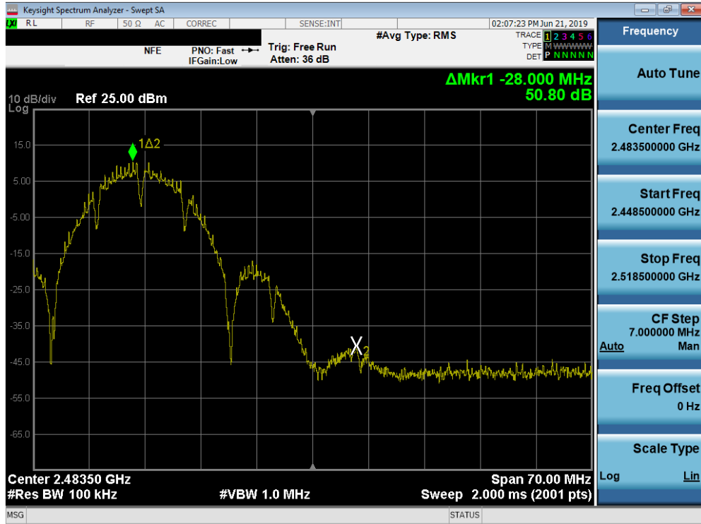
Plot 7-61. Band Edge Plot SISO ANT2 (802.11b – Ch. 11)
