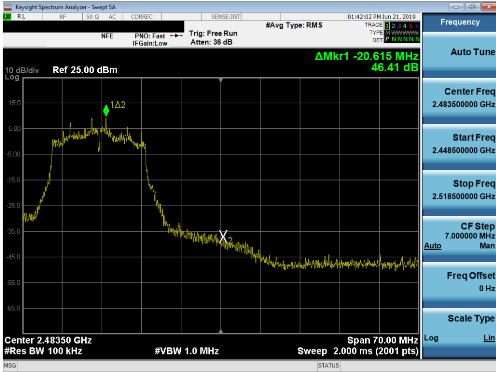
Plot 7-47. Band Edge Plot SISO ANT1 (802.11g – Ch. 11)
