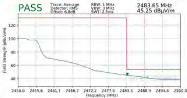
Plot 7-110. Radiated Restricted Upper Band Edge Measurement SISO ANT1 (Average)
