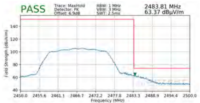
Plot 7-119. Radiated Restricted Upper Band Edge Measurement SISO ANT1 (Peak)
