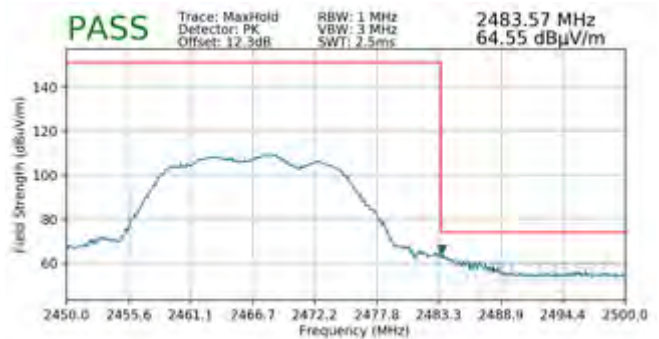
Plot 7-145. Radiated Restricted Upper Band Edge Measurement MIMO (Peak)
