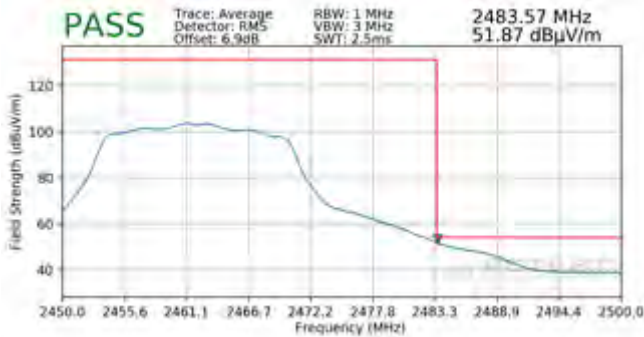
Plot 7-128. Radiated Restricted Upper Band Edge Measurement SISO ANT2 (Average)
