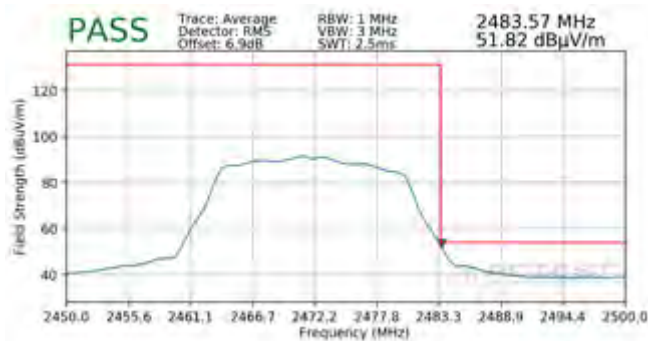
Plot 7-132. Radiated Restricted Upper Band Edge Measurement SISO ANT2 (Average)
