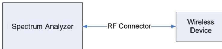
Figure 7-1. Test Instrument & Measurement Setup
