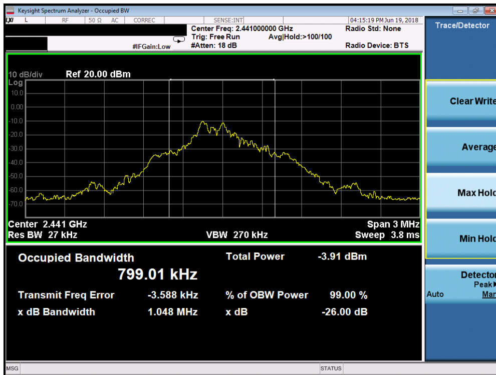
Plot 7-1. Occupied Bandwidth Plot (ANT+ – Ch. 39)
