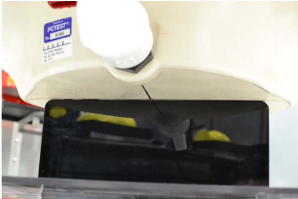
SAR Test Setup Photo 8 – Right Edge at 0.0 cm (Licensed and Unlicensed Modes)
