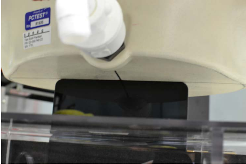
SAR Test Setup Photo 7 – Bottom Edge at 0.0 cm, (Unlicensed Modes)
