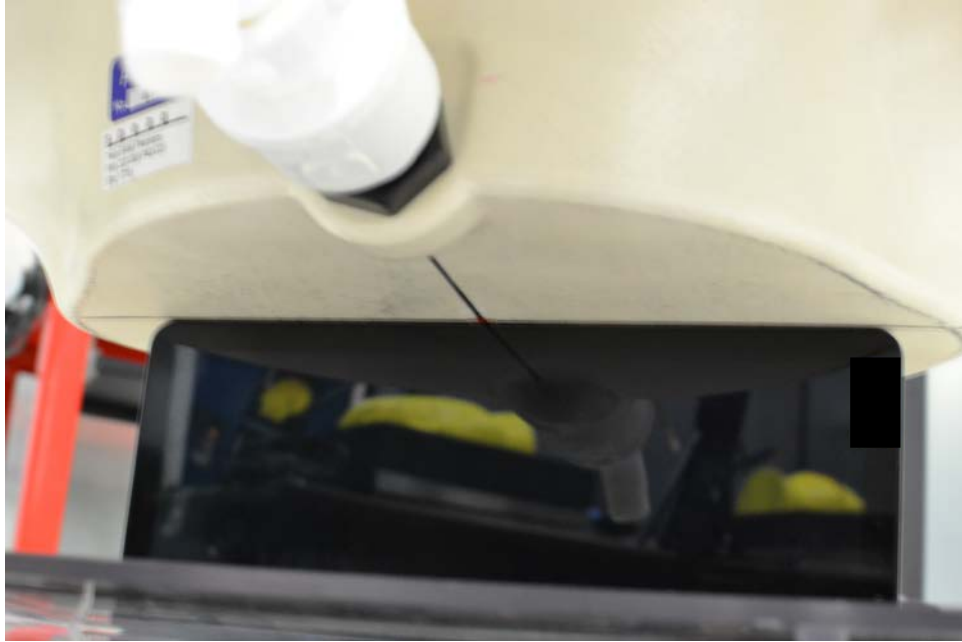
SAR Test Setup Photo 9 – Left Edge at 0.0 cm (Licensed and Unlicensed Modes)
